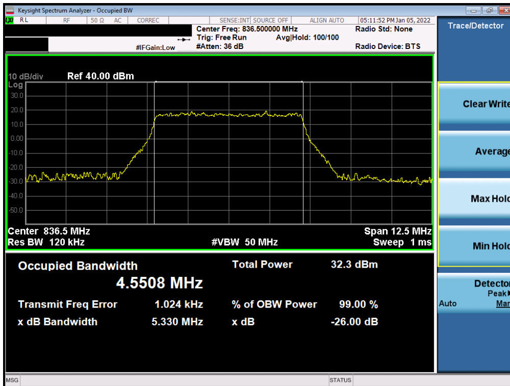
Plot 7-23. Occupied Bandwidth Plot (NR Band n5 - 5MHz \pi/2 BPSK - Full RB)
