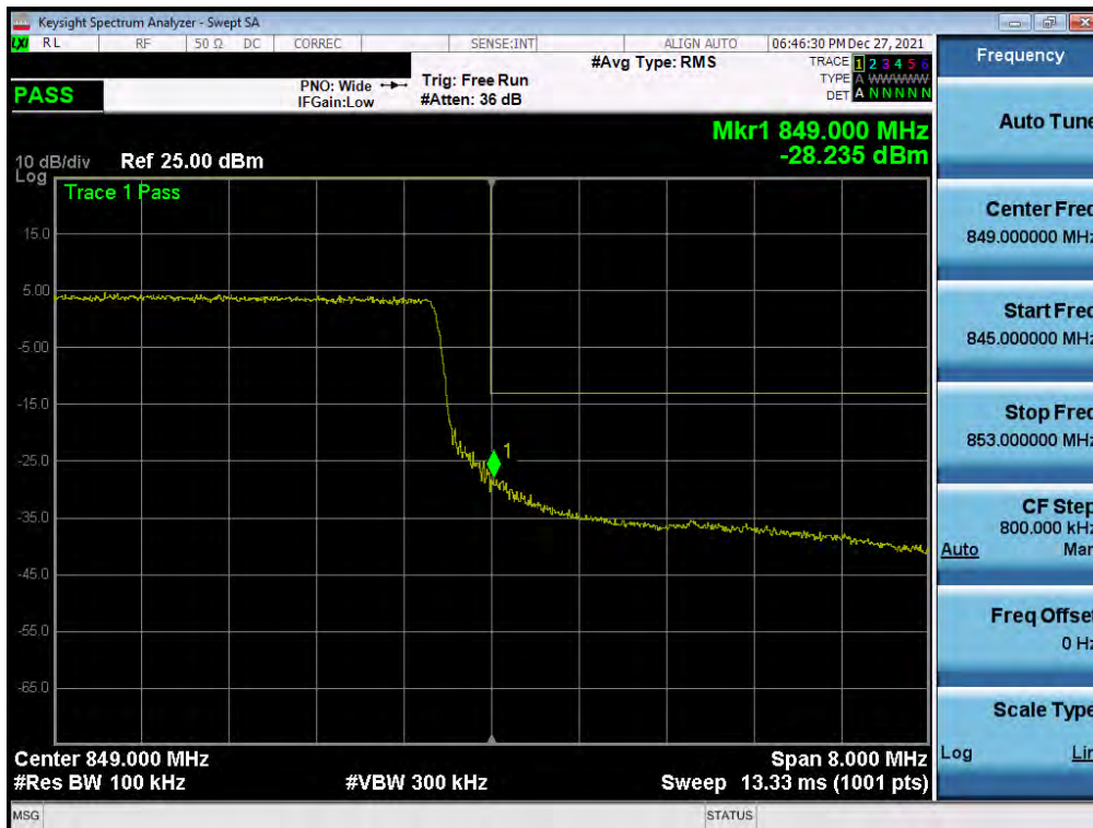
Plot 7-69. Upper Band Edge Plot (LTE Band 26/5 - 10MHz QPSK – Full RB)
