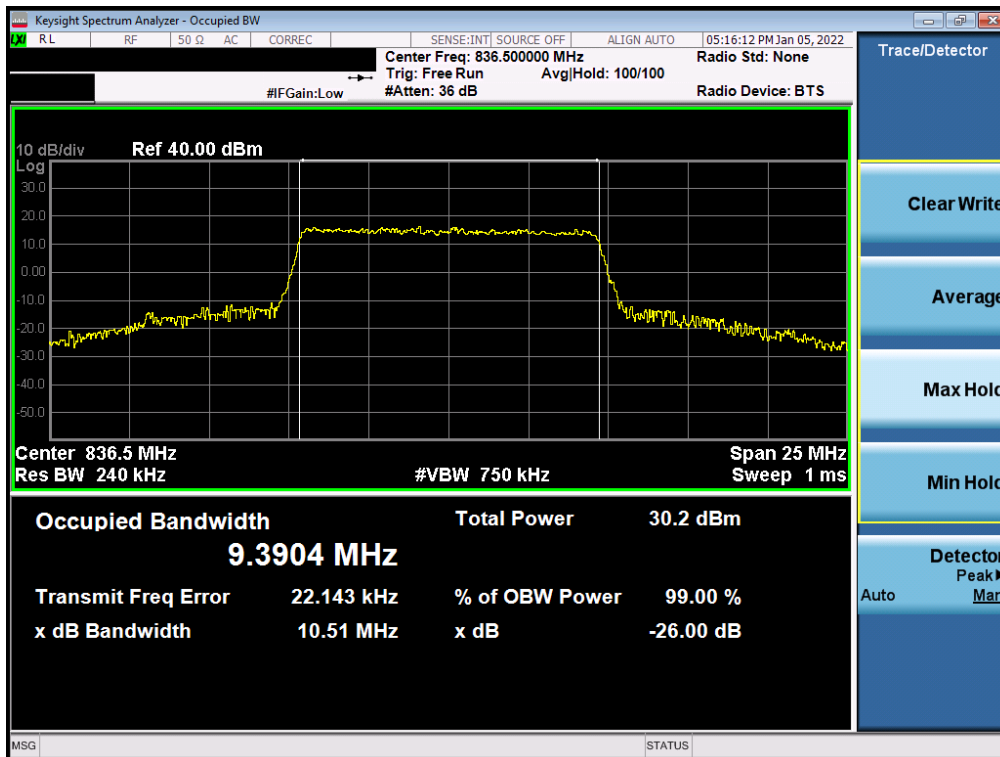
Plot 7-21. Occupied Bandwidth Plot (NR Band n5 - 10MHz QPSK - Full RB)
