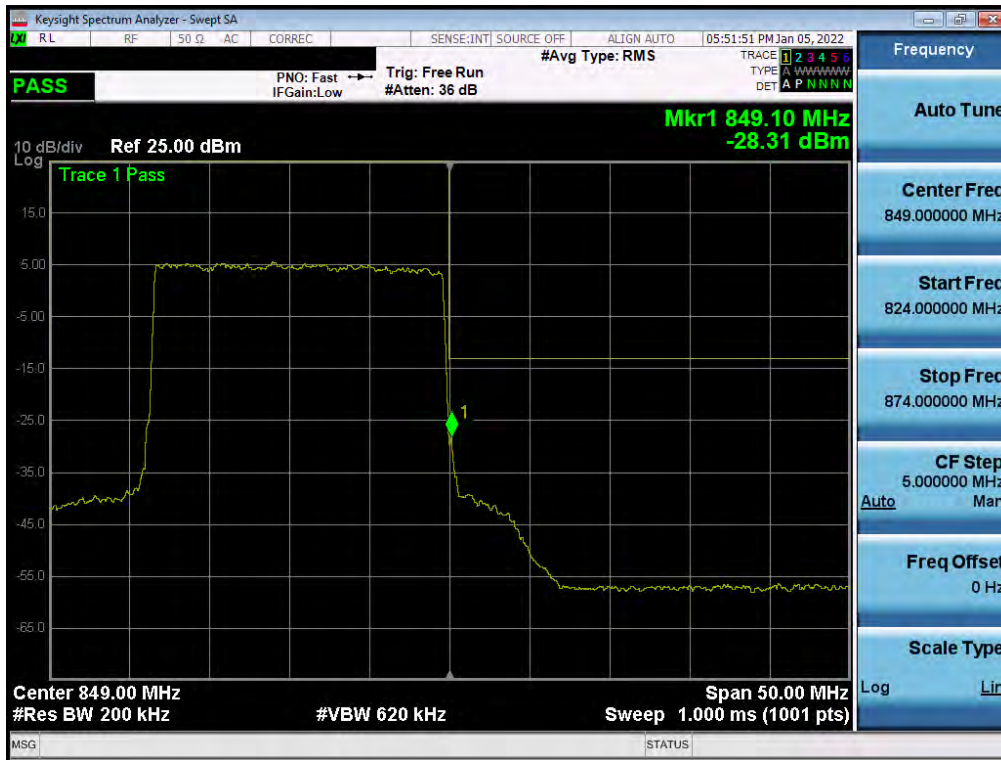
Plot 7-77. Upper Band Edge Plot (NR Band n5 – 20.0MHz - Full RB)
