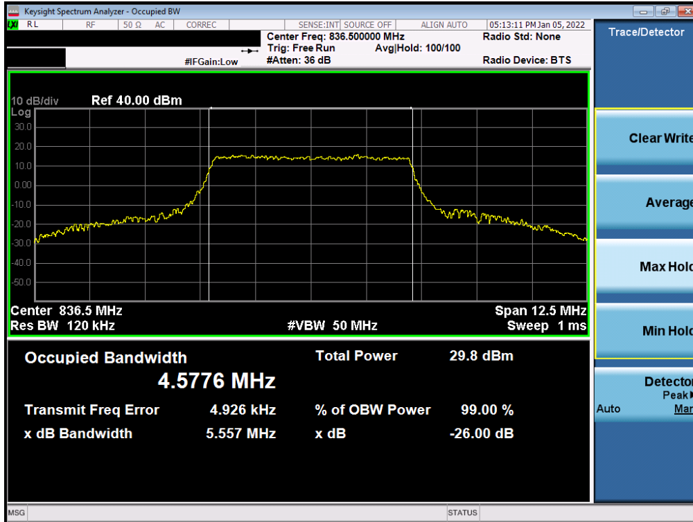
Plot 7-24. Occupied Bandwidth Plot (NR Band n5 - 5MHz QPSK - Full RB)
