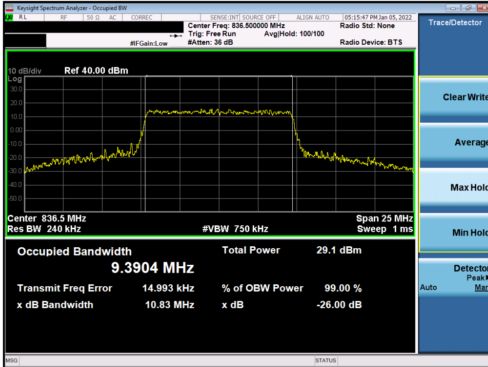
Plot 7-22. Occupied Bandwidth Plot (NR Band n5 - 10MHz 16-QAM - Full RB)
