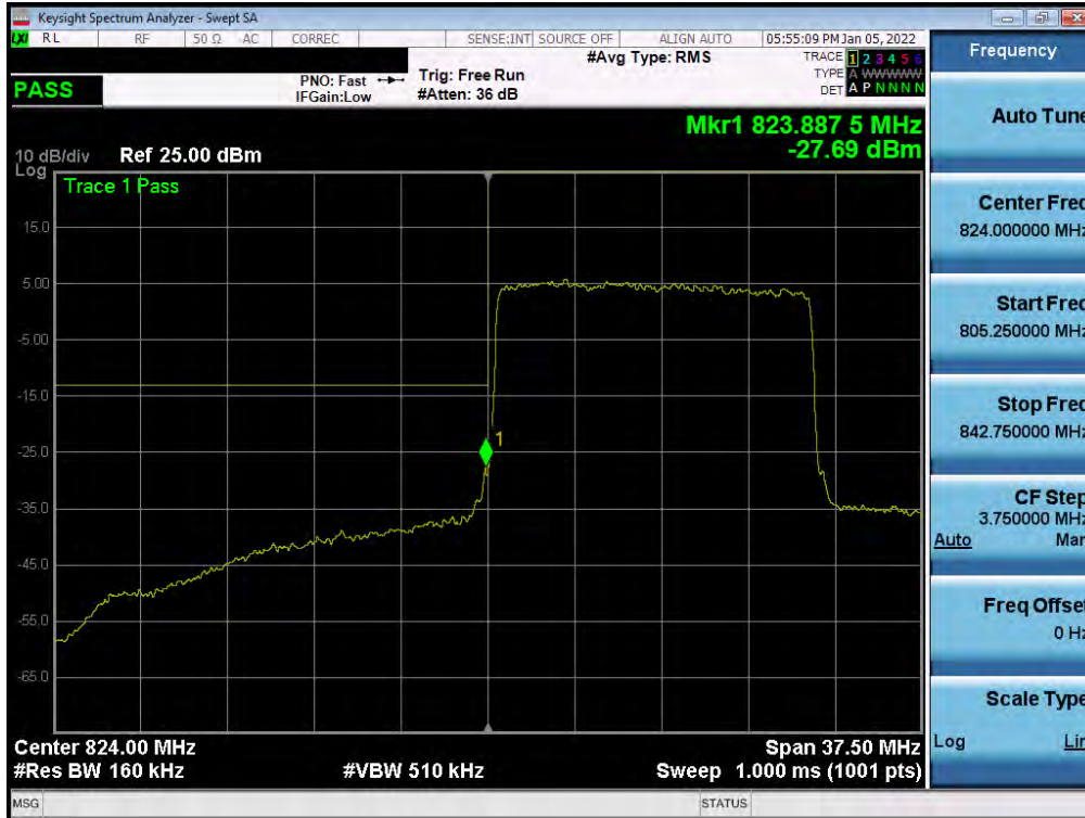
Plot 7-78. Lower Band Edge Plot (NR Band n5 – 15.0MHz - Full RB)
