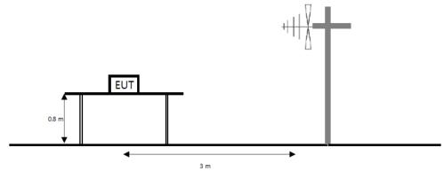
The diagram below shows the test setup that is utilized to make the measurements for emission from 1 ℍ to the tenth harmonic of the highest fundamental frequency or to 40 ℍ emissions, whichever is lower.
