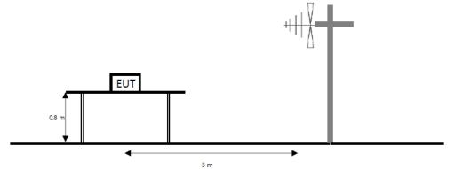
The diagram below shows the test setup that is utilized to make the measurements for emission from 1 Gh to the tenth harmonic of the highest fundamental frequency or to 40 Gh emissions, whichever is lower.
