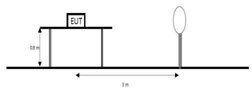
The diagram below shows the test setup that is utilized to make the measurements for emission from 30 Mb to 1 Gb emissions.
