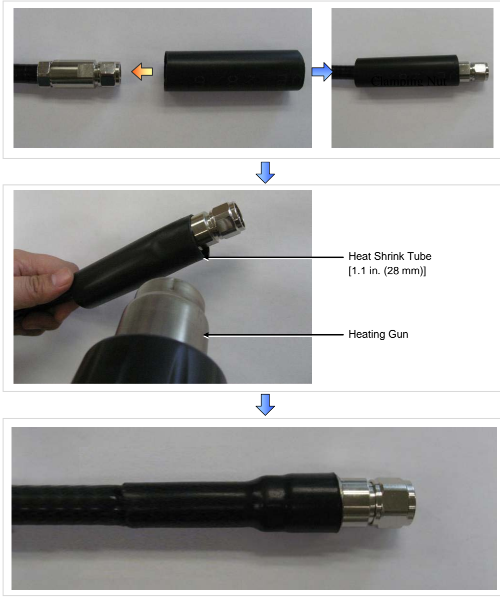
Figure C.11 Assembling the N type-male Connector (1/2 in. Feeder Line) (4)
