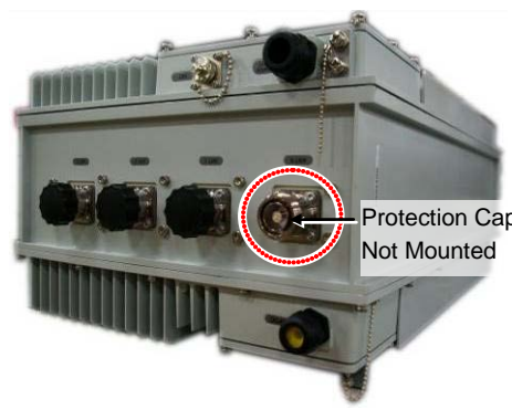
[Bad: Protection Cap Not Mounted]
