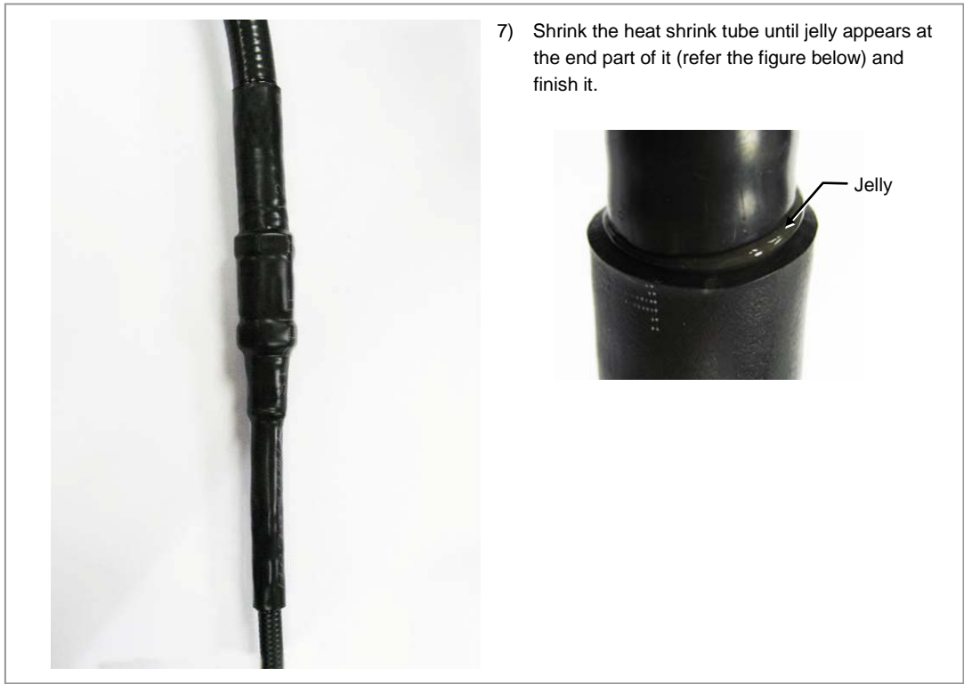
Figure C.19 Shrinking the Heat Shrink Tube-Connector (3)
