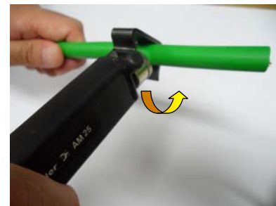
Figure E.4 Stripping Cable Sheath (1)
