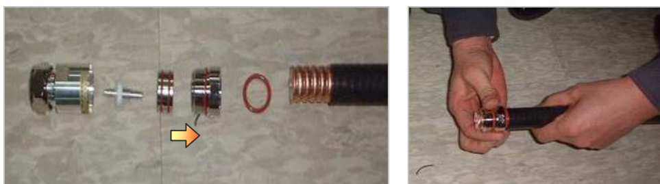
Figure C.12 Assembling the Din type-male Connector (1/2 in. Feeder Line) (1)
