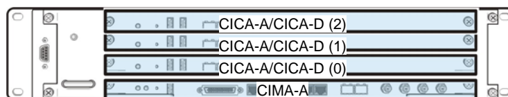
Figure 3.8 UADU Configuration - CDMA Only
