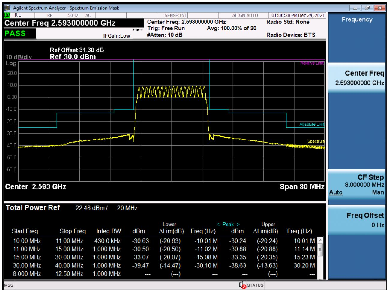
High Channel Edge Plot (20 MHz Ch.41490 QPSK RB 1, Offset 99) (POWER CLASS 3)
