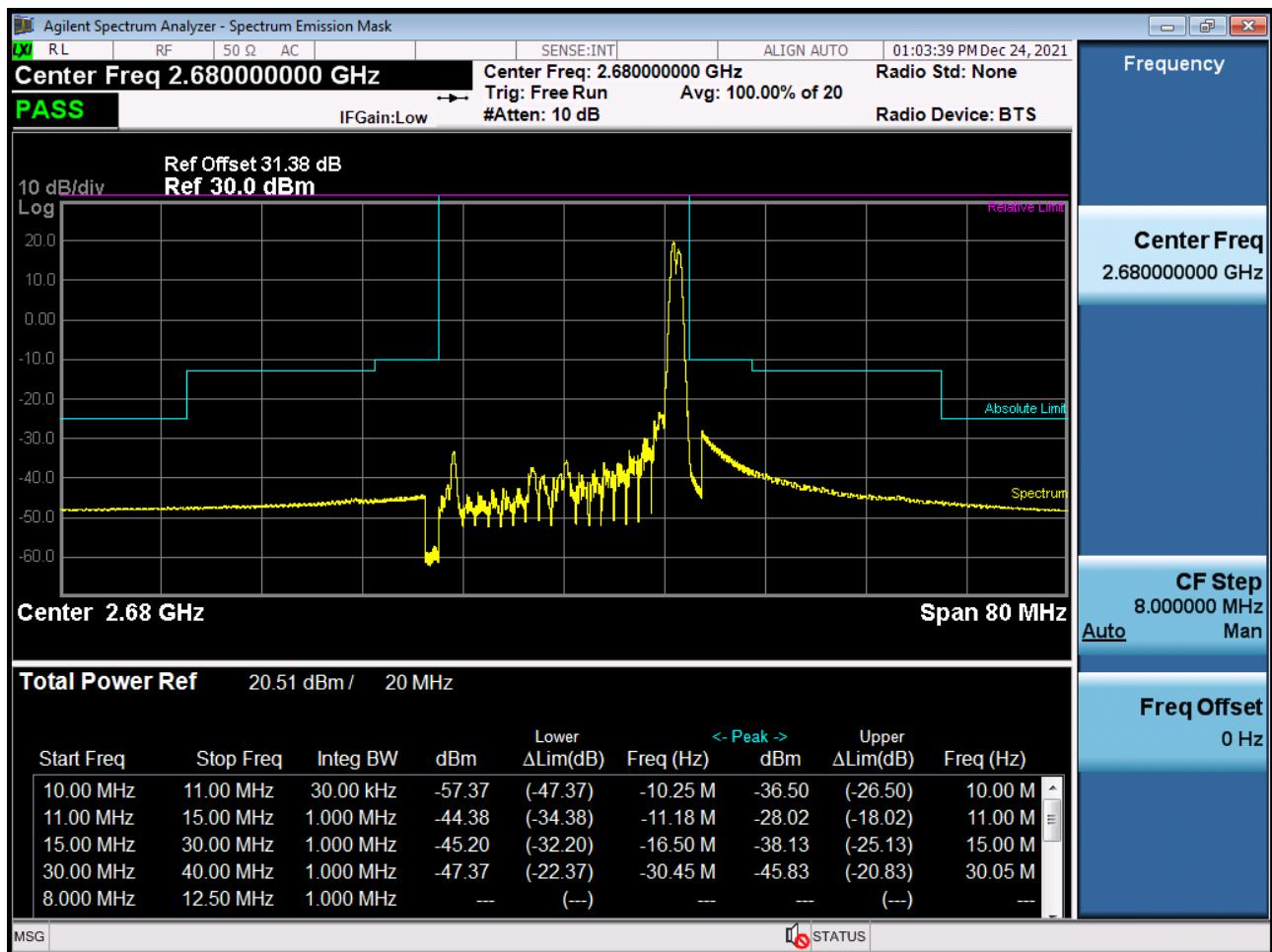
High Channel Edge Plot (20 MHz Ch.41490 QPSK\_RB100\_Offset 0) (POWER CLASS 3)
