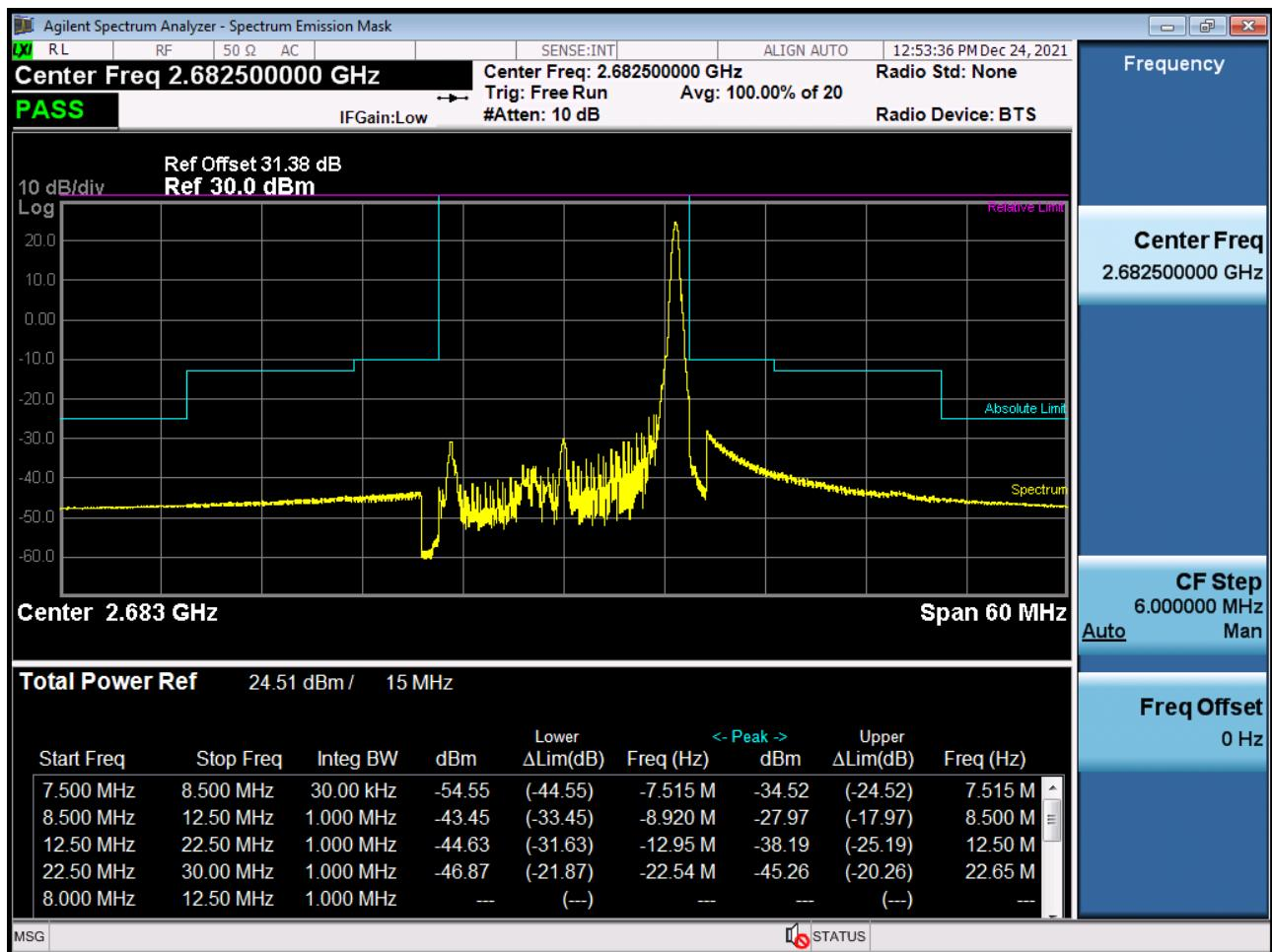
High Channel Edge Plot (15 MHz Ch.41515 QPSK\_RB75\_Offset 0) (POWER CLASS 3)
