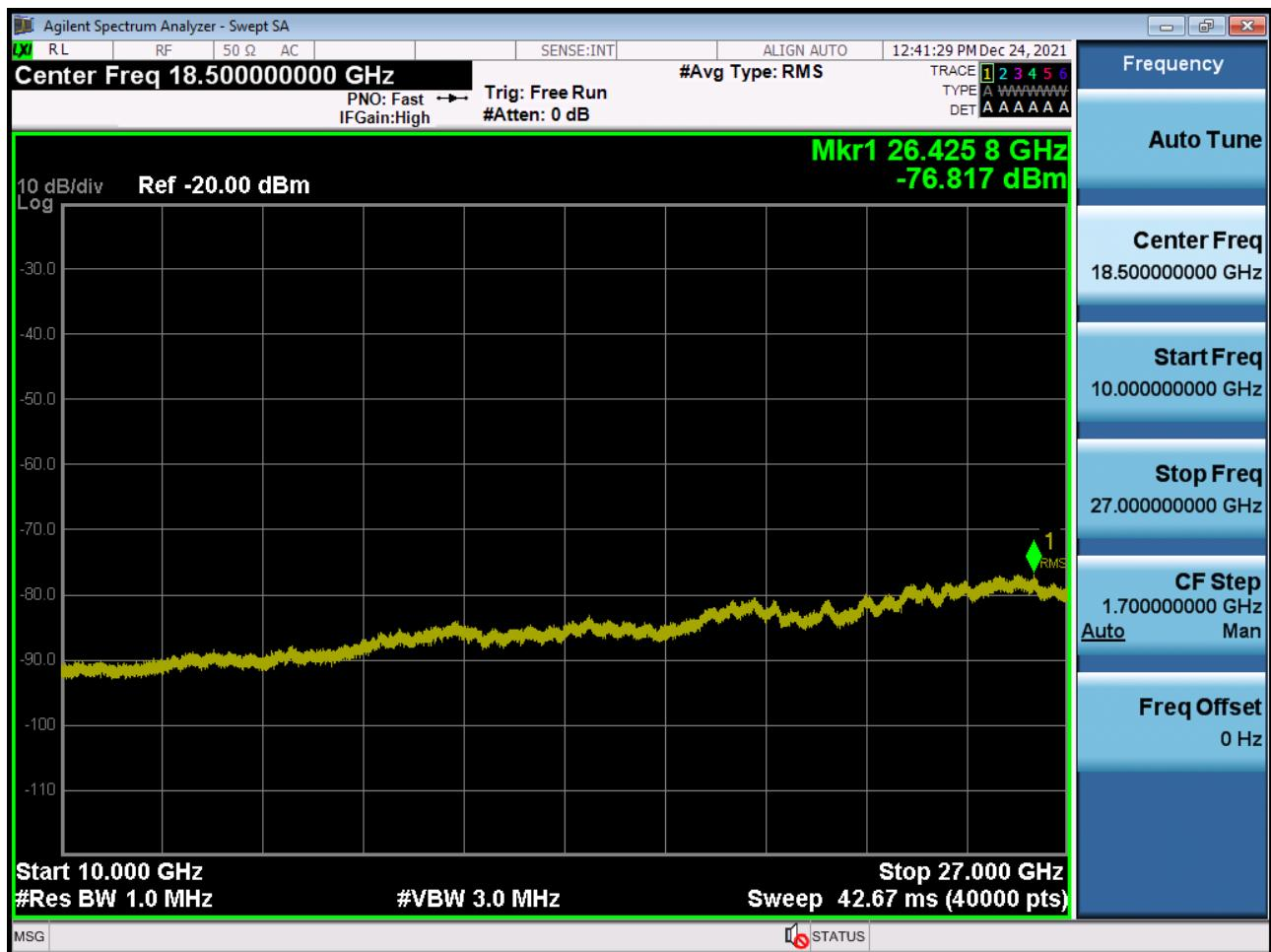
Conducted Spurious Plot 1 (10 MHz Ch. 41540 QPSK RB 1, Offset 0) (POWER CLASS 3)
