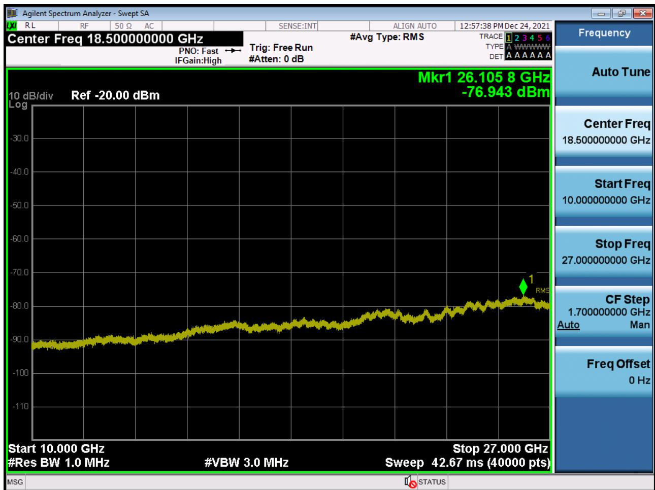
Conducted Spurious Plot 1 (20 MHz Ch.40620 QPSK RB 1, Offset 0) (POWER CLASS 3)
