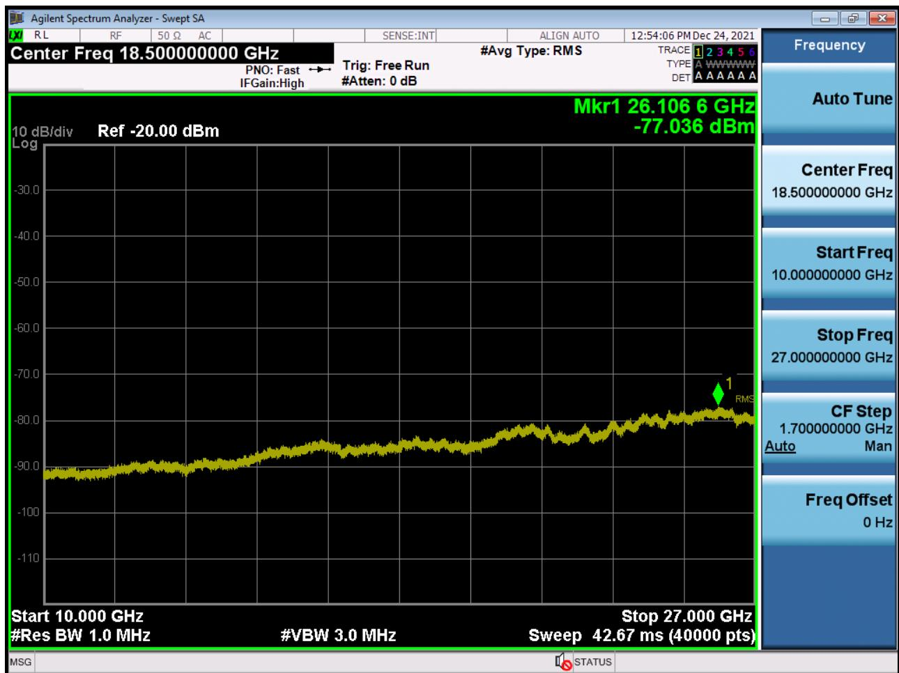
Conducted Spurious Plot 1 (20 MHz Ch.39750 QPSK RB 1, Offset 0) (POWER CLASS 3)
