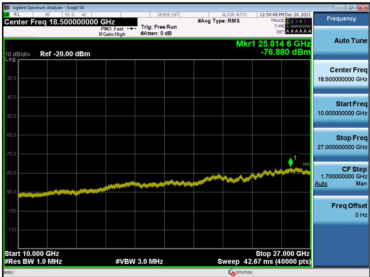
Conducted Spurious Plot 1 (10 MHz Ch.39700 QPSK RB 1, Offset 0) (POWER CLASS 3)
