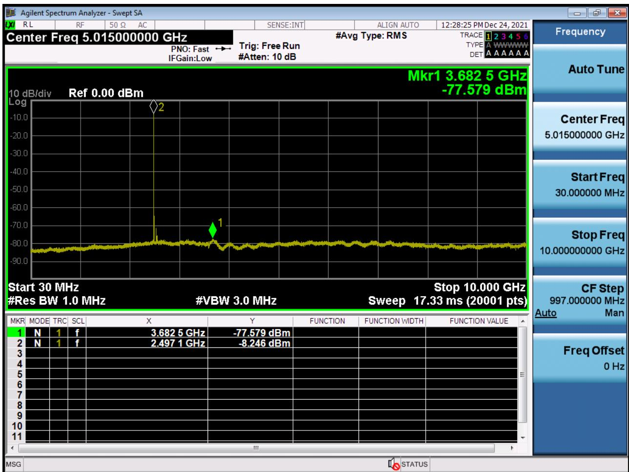
Conducted Spurious Plot 2 (5 MHz Ch. 39675 QPSK RB 1, Offset 0) (POWER CLASS 3)
