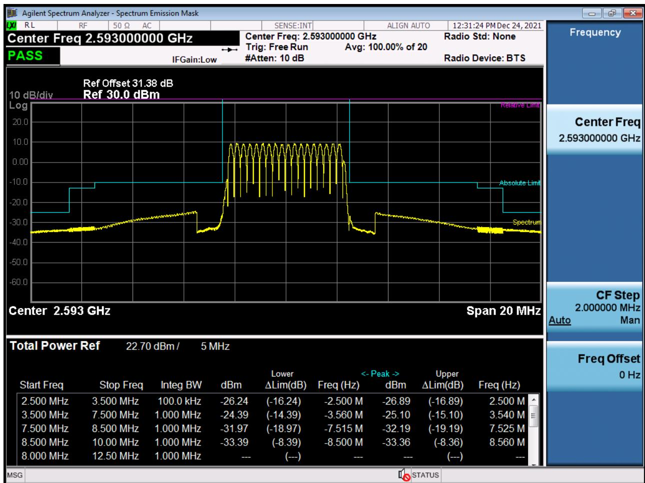
High Channel Edge Plot (5 MHz Ch.41565 QPSK RB 1, Offset 24) (POWER CLASS 3)
