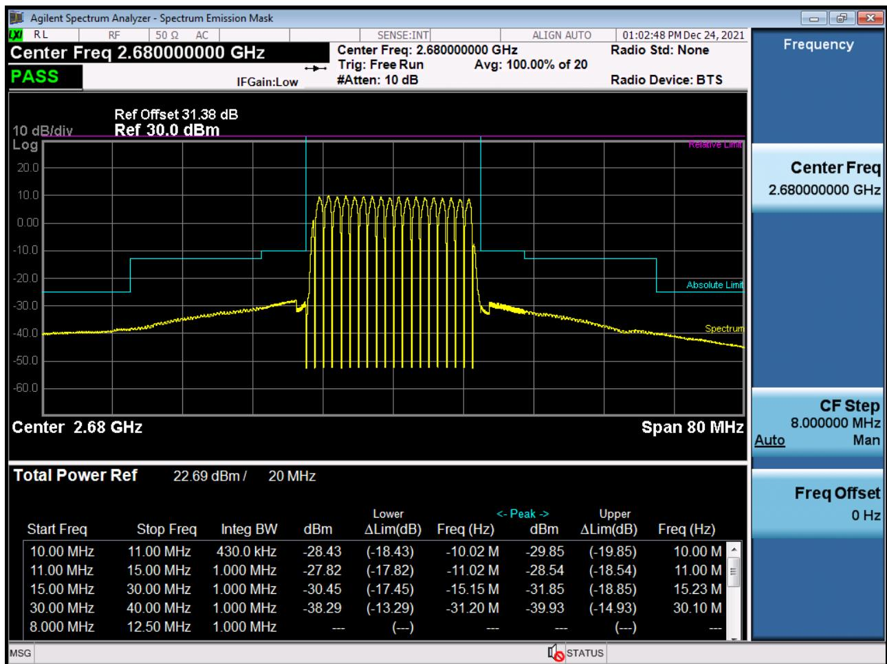
Conducted Spurious Plot 1 (5 MHz Ch.39675 QPSK RB 1, Offset 0) (POWER CLASS 3)
