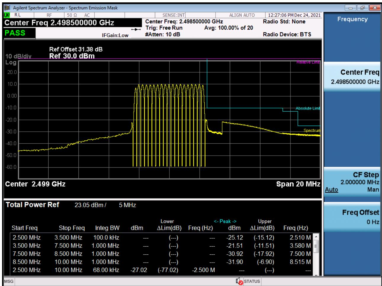
Mid Channel Edge Plot (5 MHz Ch.40620 QPSK RB 25) (POWER CLASS 3)
