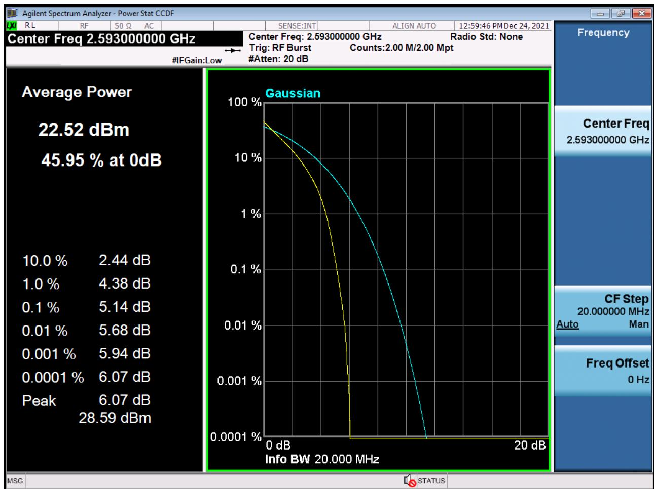
PAR Plot (20 M BW\_Ch.40620\_16QAM\_RB100\_0) (POWER CLASS 3)
