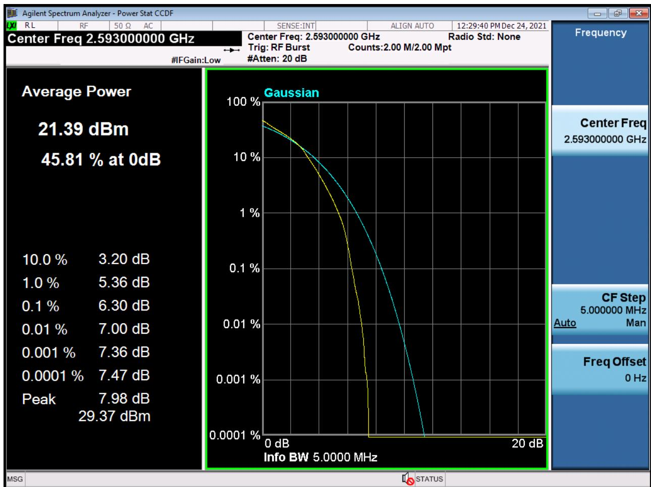
PAR Plot (5 M BW\_Ch.40620\_64QAM\_RB25\_0) (POWER CLASS 3)
