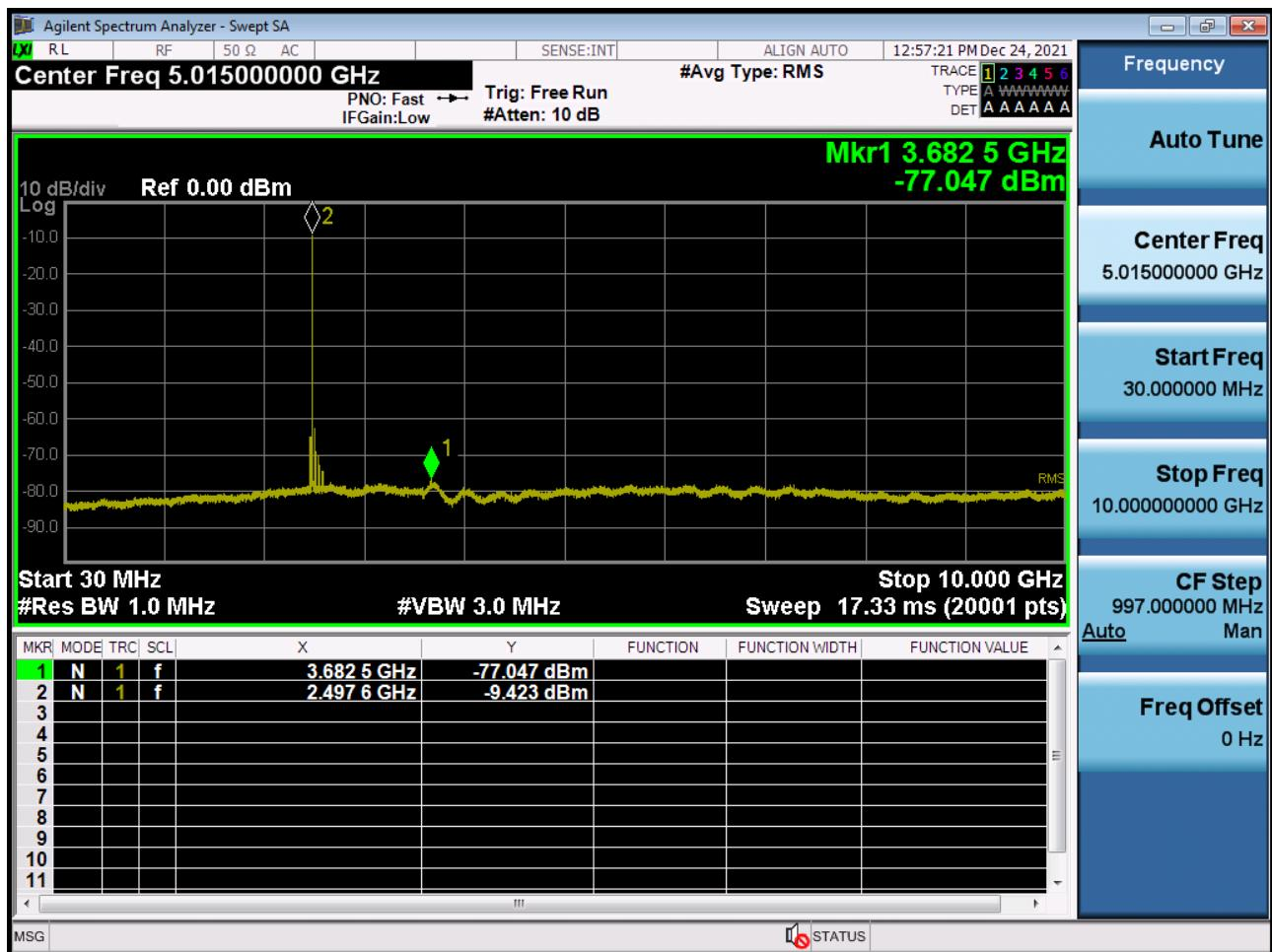
Conducted Spurious Plot 2 (20 MHz Ch. 39750 QPSK RB 1, Offset 0) (POWER CLASS 3)
