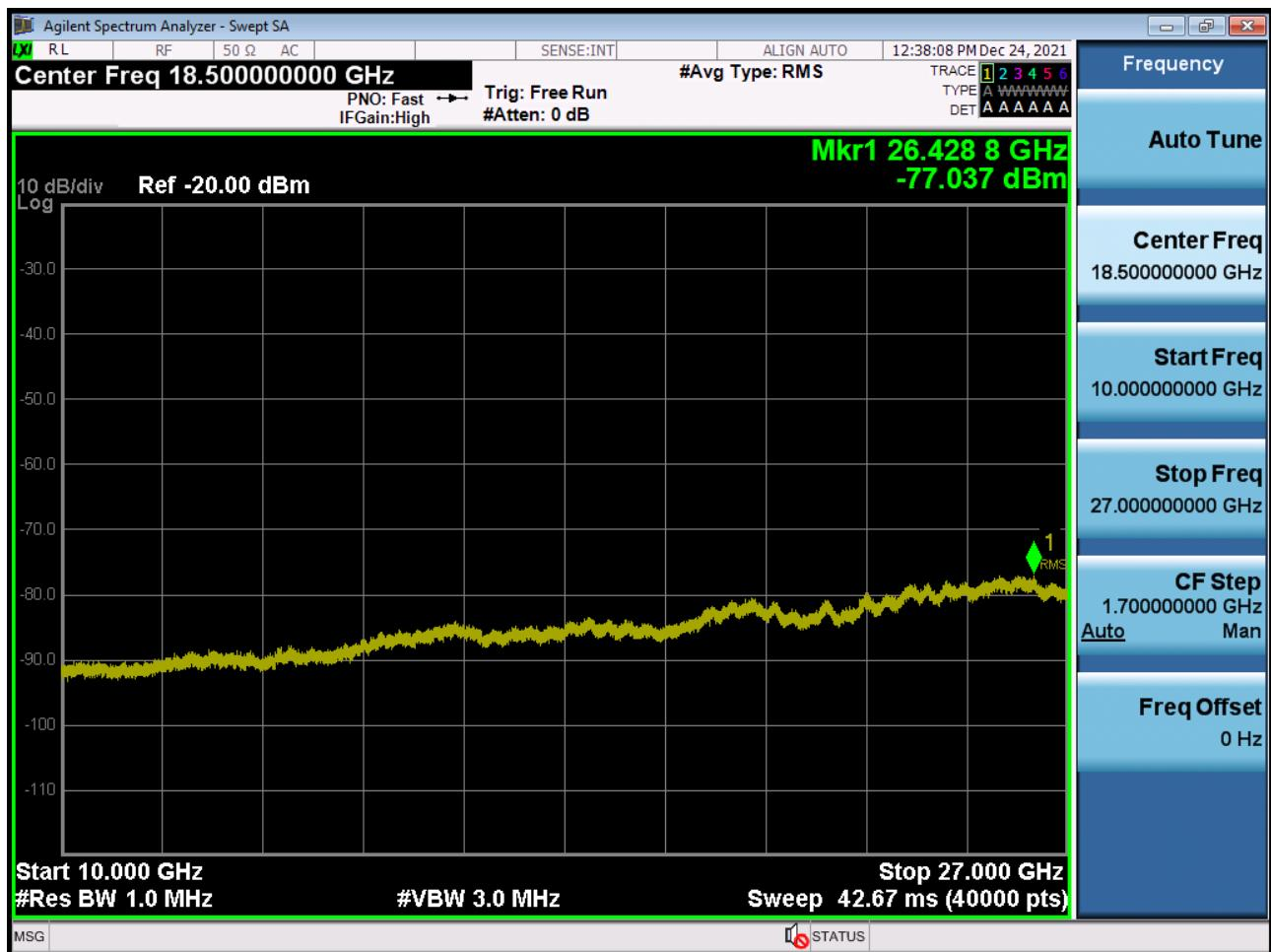
Conducted Spurious Plot 1 (10 MHz Ch.40620 QPSK RB 1, Offset 0) (POWER CLASS 3)
