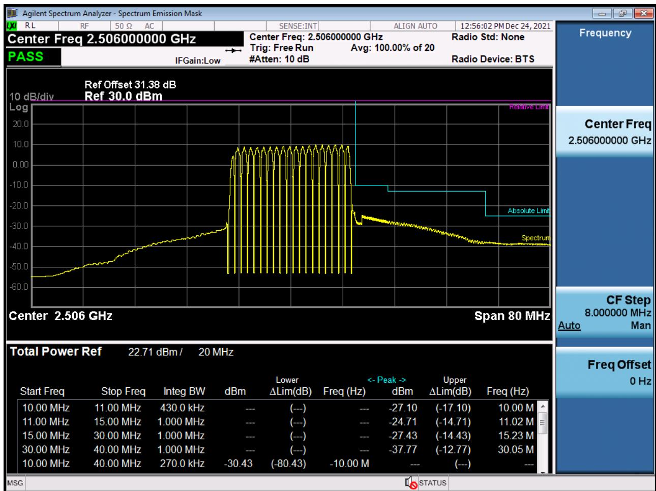
Mid Channel Edge Plot (20 MHz Ch.40620 QPSK RB 100) (POWER CLASS 3)
