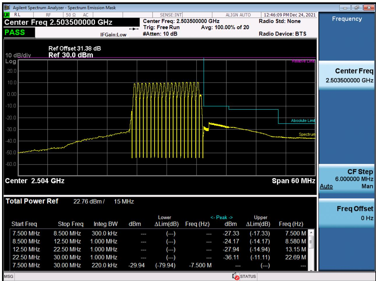
Mid Channel Edge Plot (15 MHz Ch.40620 QPSK RB 75) (POWER CLASS 3)
