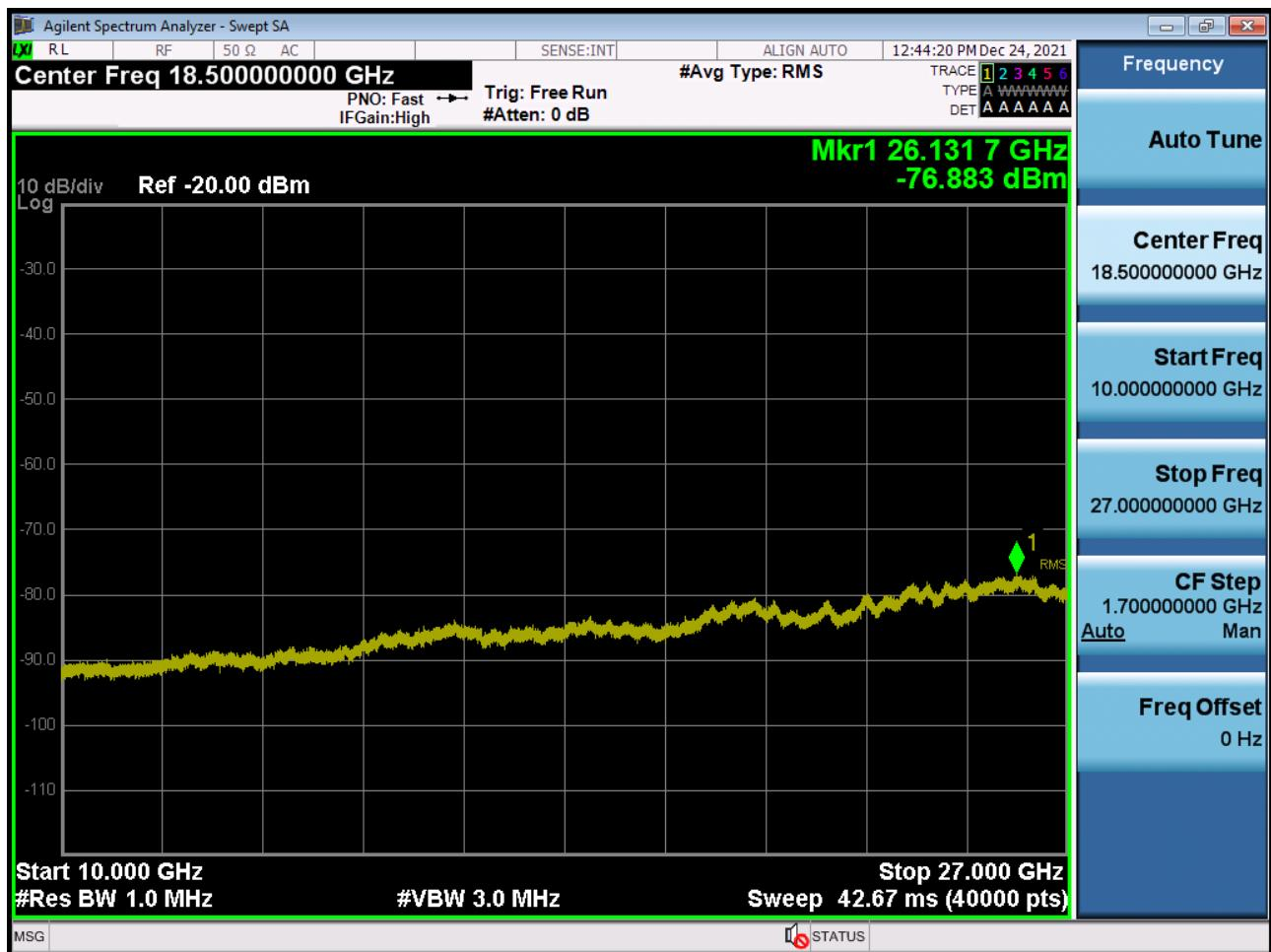
Conducted Spurious Plot 1 (15 MHz Ch.39725 QPSK RB 1, Offset 0) (POWER CLASS 3)
