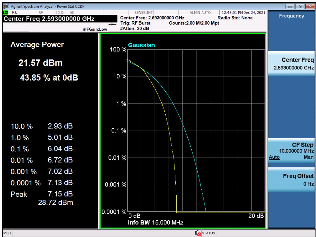
PAR Plot (15 M BW\_Ch.40620\_64QAM\_RB75\_0) (POWER CLASS 3)
