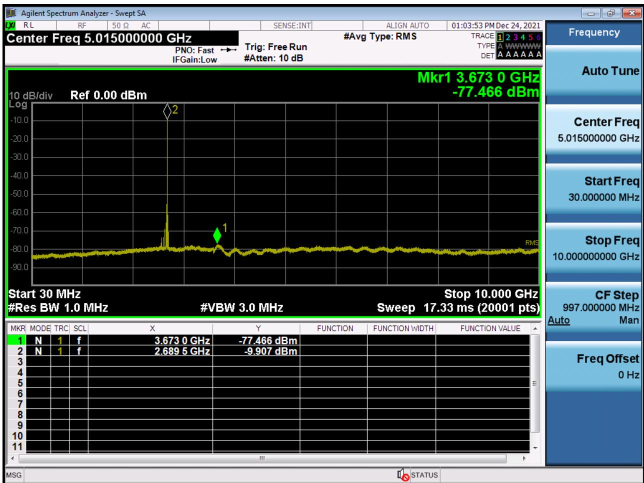
Conducted Spurious Plot 2 (20 MHz Ch. 41490 QPSK RB 1, Offset 0) (POWER CLASS 3)
