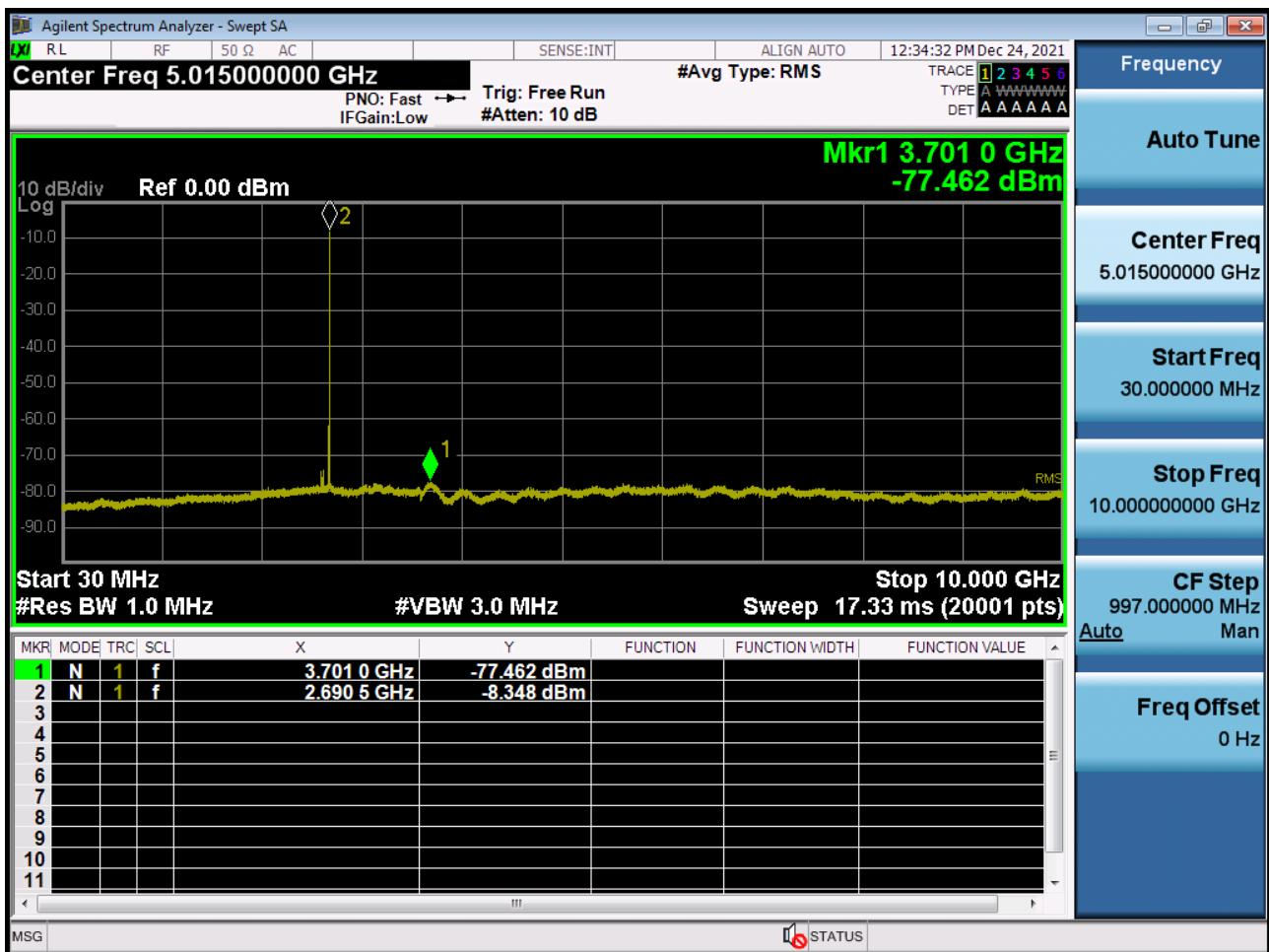
Conducted Spurious Plot 2 (5 MHz Ch. 41565 QPSK RB 1, Offset 0) (POWER CLASS 3)
