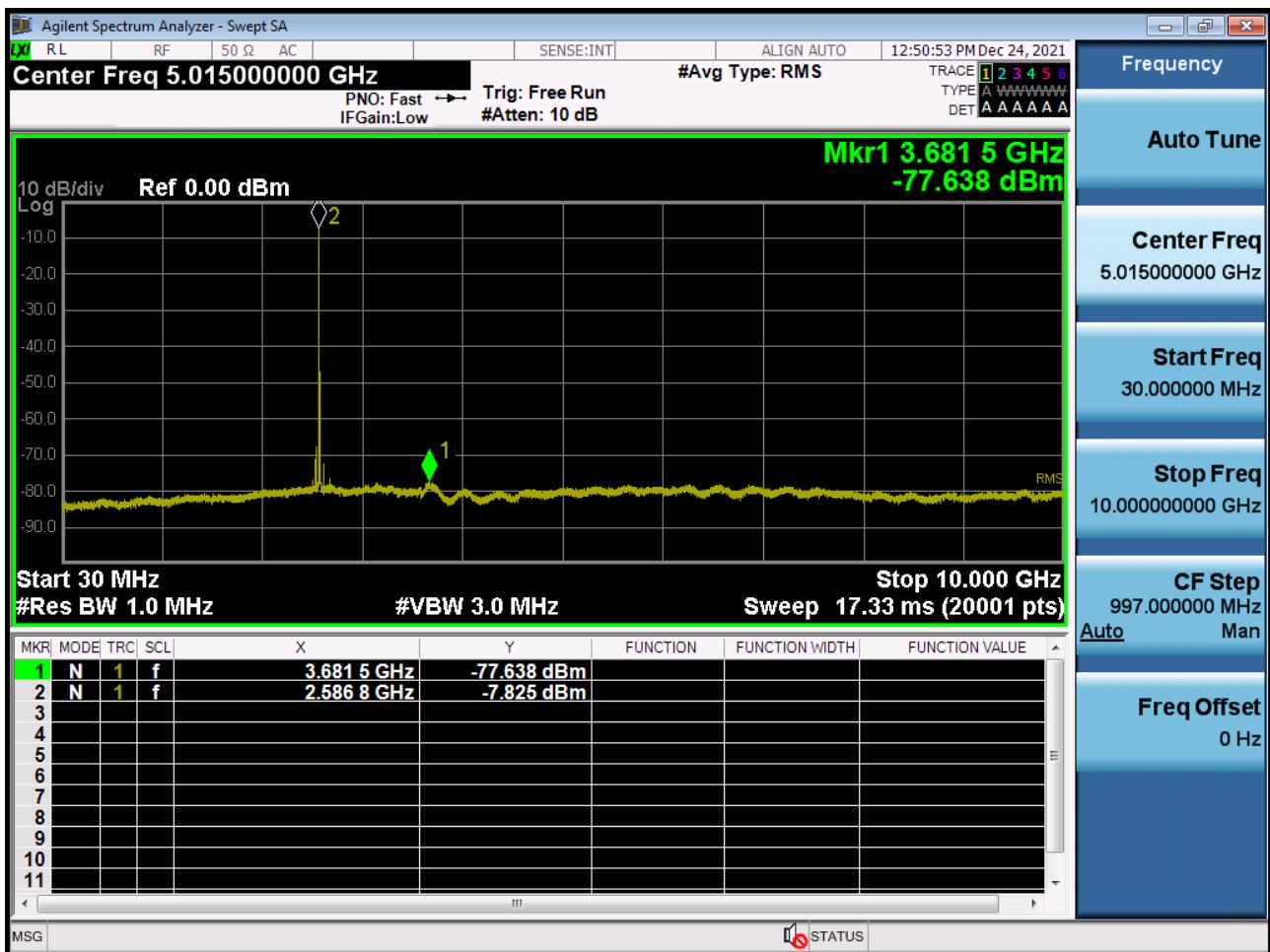
Conducted Spurious Plot 2 (15 MHz Ch. 40620 QPSK RB 1, Offset 0) (POWER CLASS 3)
