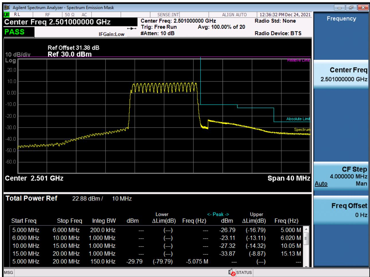
Mid Channel Edge Plot (10 MHz Ch.40620 QPSK RB 50) (POWER CLASS 3)
