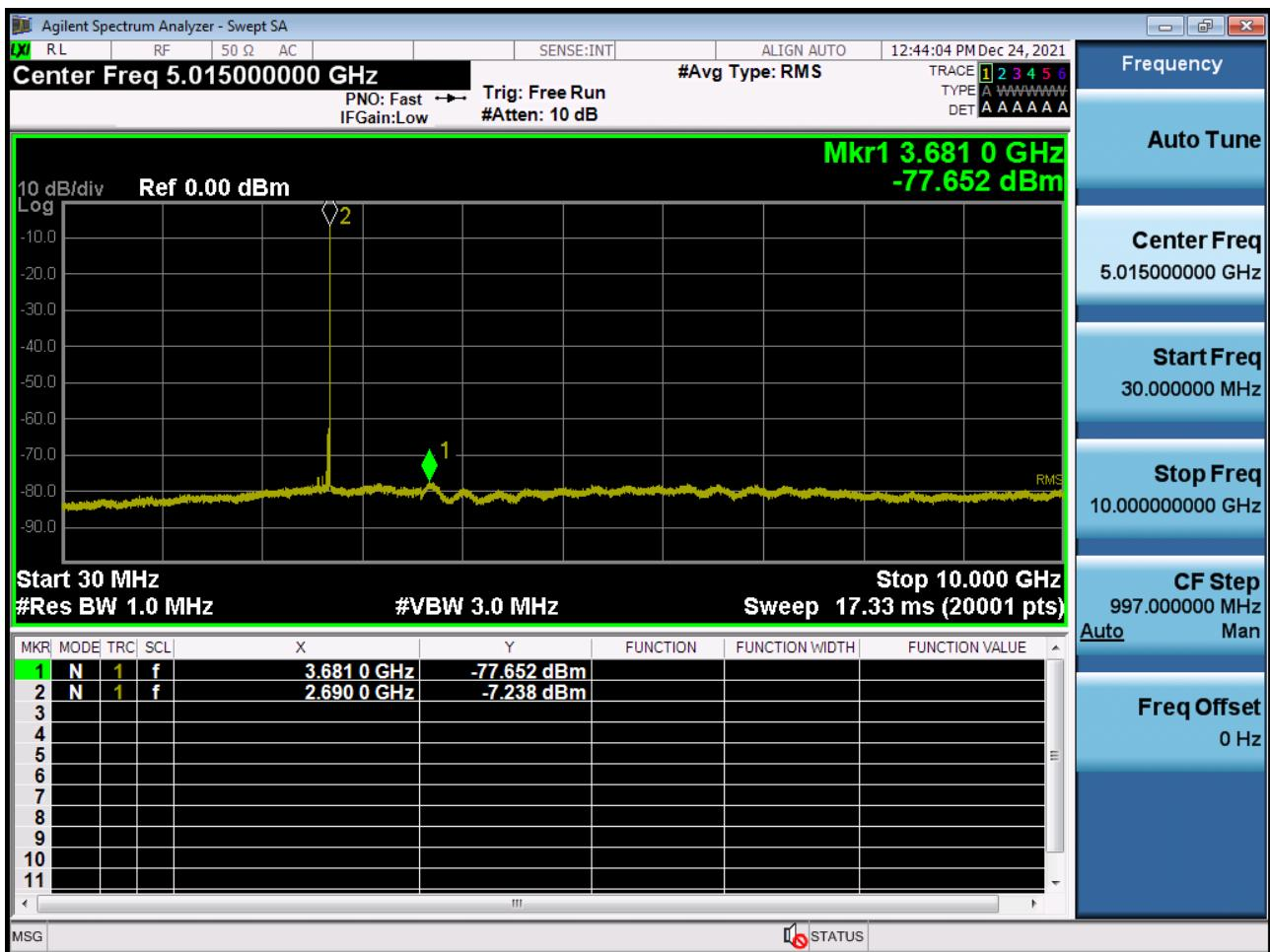
Conducted Spurious Plot 2 (10 MHz Ch. 41540 QPSK RB 1, Offset 0) (POWER CLASS 3)
