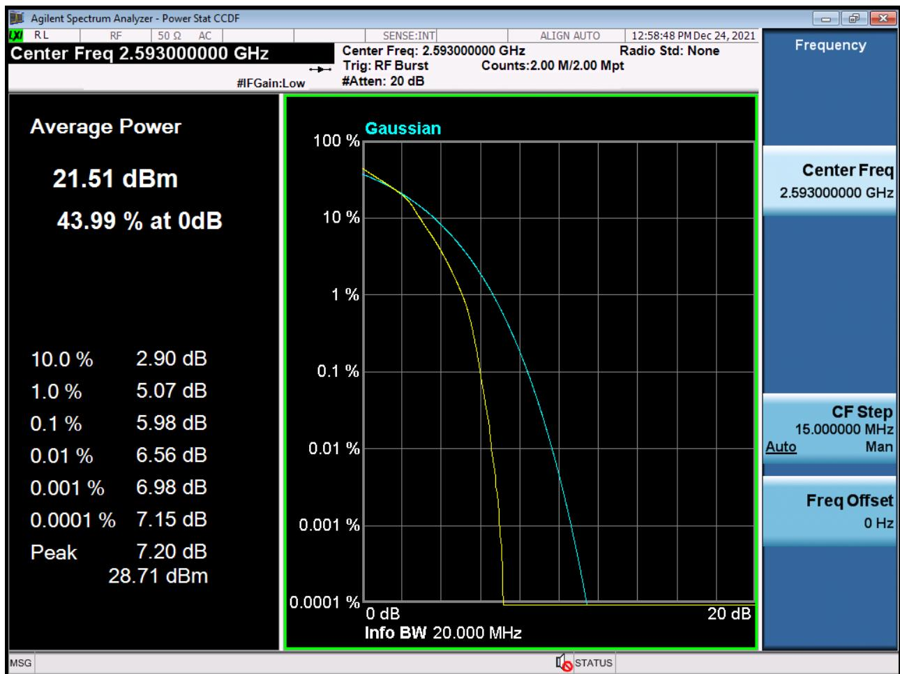
PAR Plot (20 M BW\_Ch.40620\_64QAM\_RB100\_0) (POWER CLASS 3)
