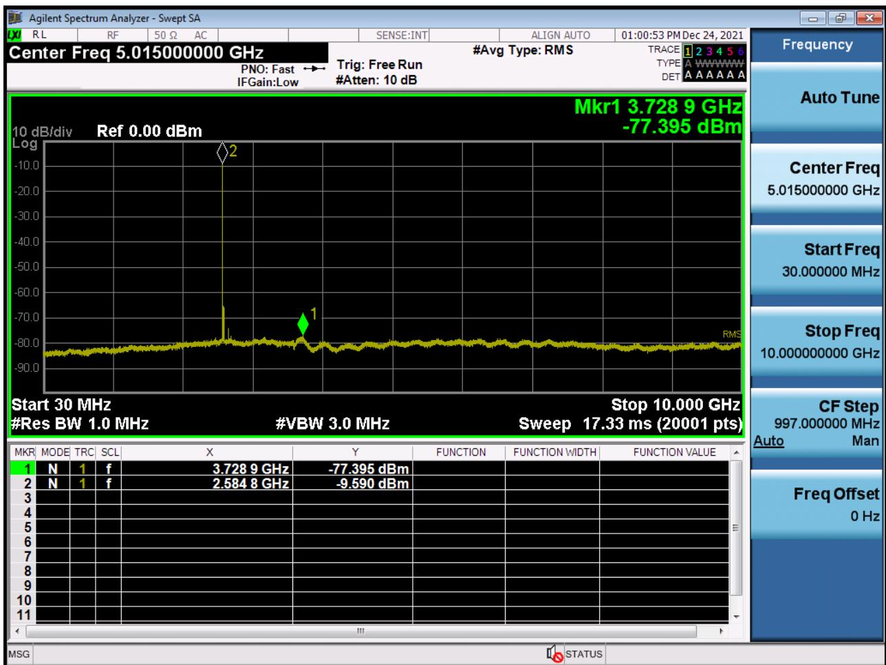
Conducted Spurious Plot 2 (20 MHz Ch. 40620 QPSK RB 1, Offset 0) (POWER CLASS 3)
