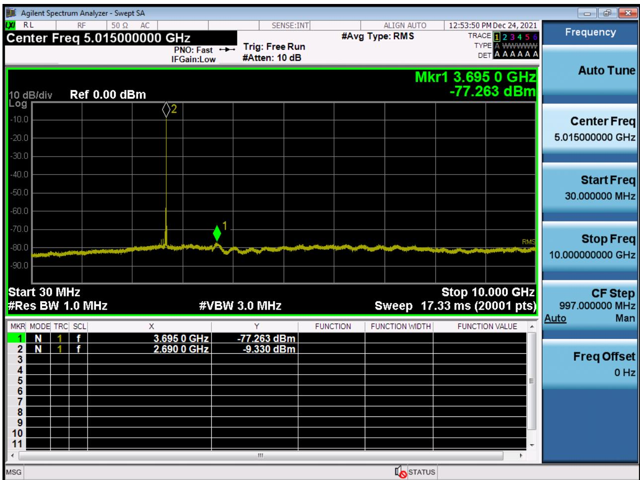
Conducted Spurious Plot 2 (15 MHz Ch. 41515 QPSK RB 1, Offset 0) (POWER CLASS 3)
