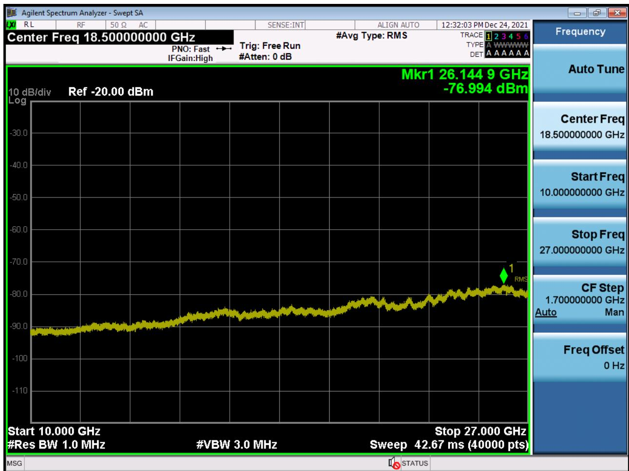
Conducted Spurious Plot 1 (5 MHz Ch.41565 QPSK RB 1, Offset 0) (POWER CLASS 3)
