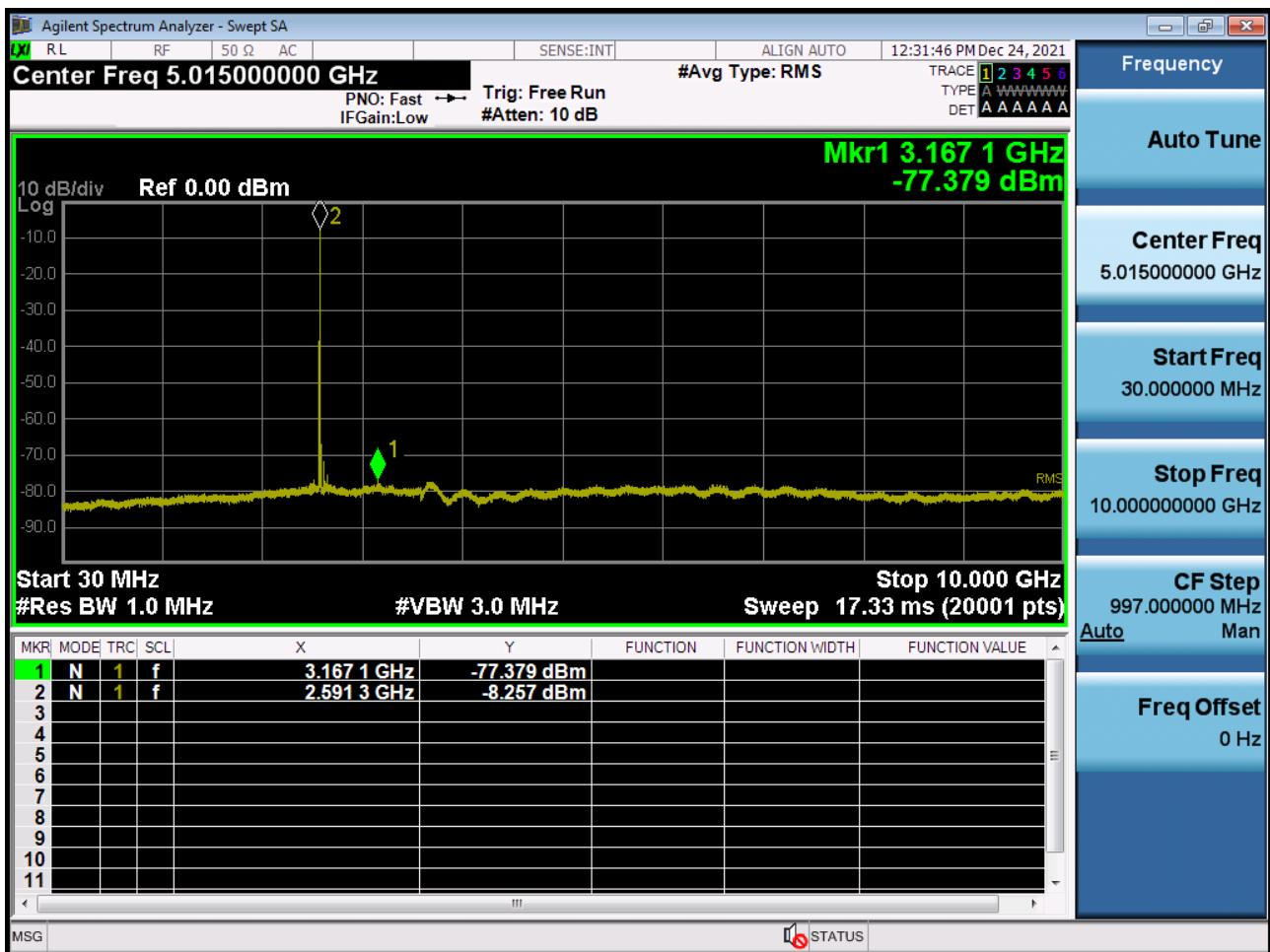
Conducted Spurious Plot 2 (5 MHz Ch. 40620 QPSK RB 1, Offset 0) (POWER CLASS 3)
