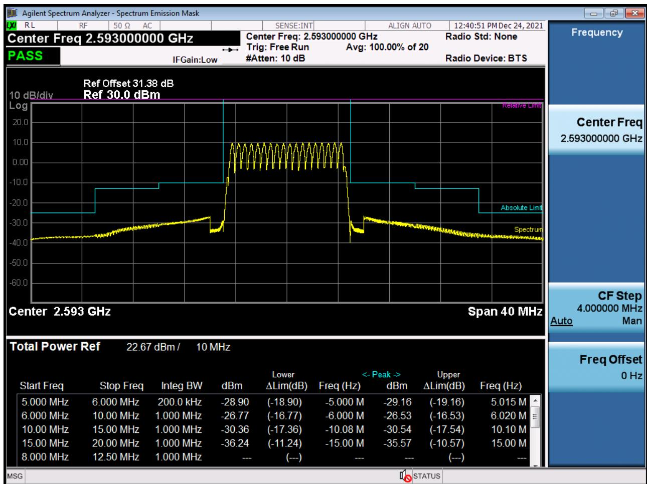
High Channel Edge Plot (10 MHz Ch.41540 QPSK RB 1, Offset 24) (POWER CLASS 3)
