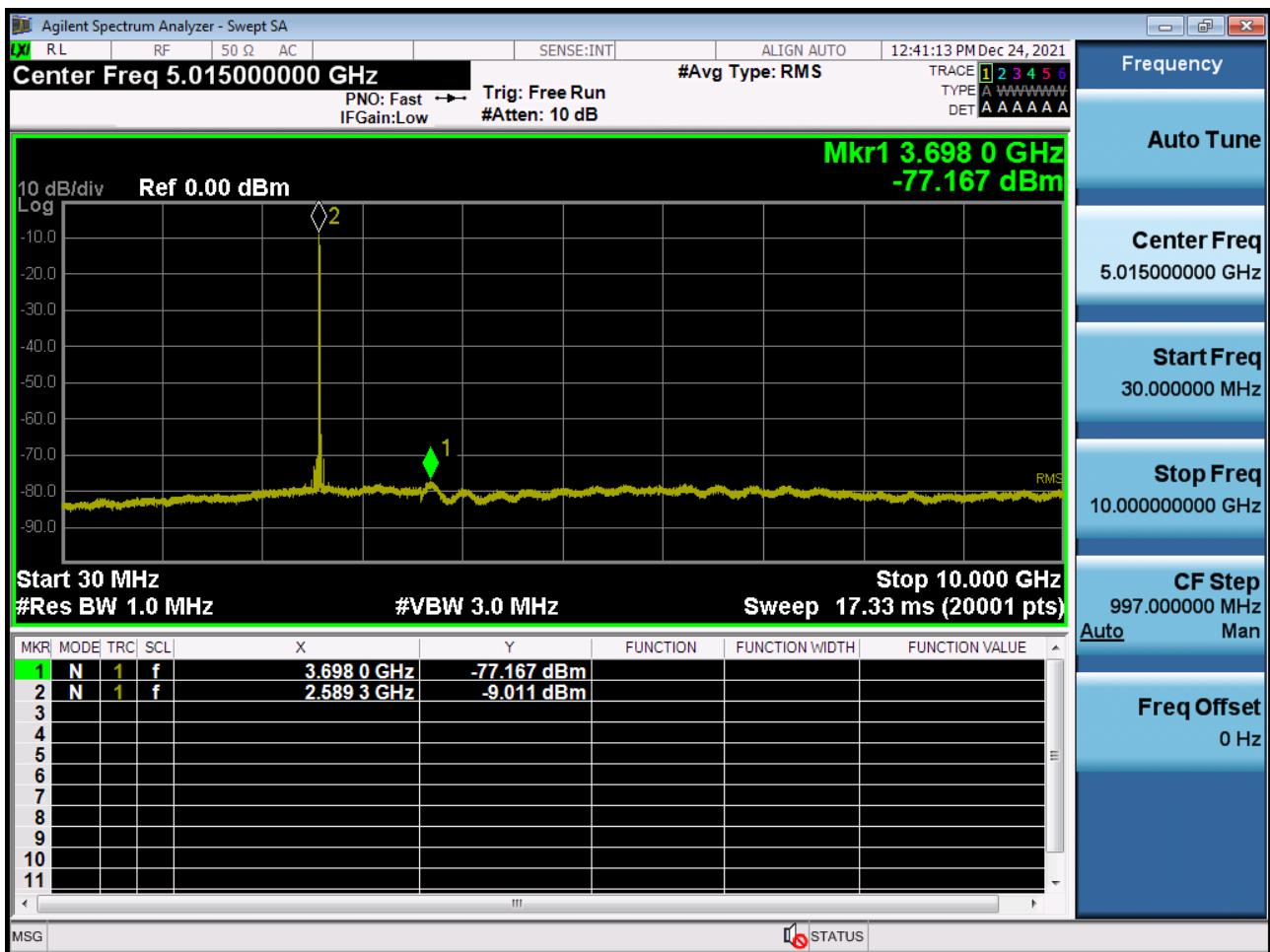
Conducted Spurious Plot 2 (10 MHz Ch. 40620 QPSK RB 1, Offset 0) (POWER CLASS 3)
