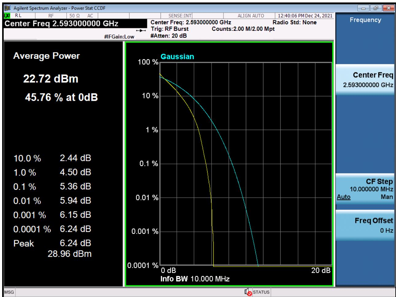
PAR Plot (10 M BW\_Ch.40620\_16QAM\_RB50\_0) (POWER CLASS 3)
