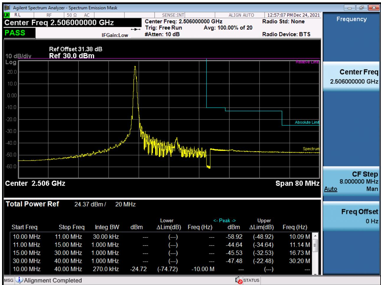
Low Channel Edge Plot (20 MHz Ch.39750 QPSK\_RB100\_Offset 0)-1 (POWER CLASS 3)
