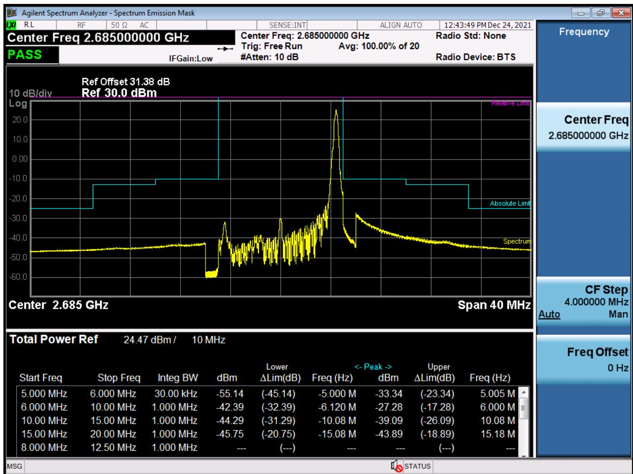
High Channel Edge Plot (10 MHz Ch.41540 QPSK\_RB50\_Offset 0) (POWER CLASS 3)
