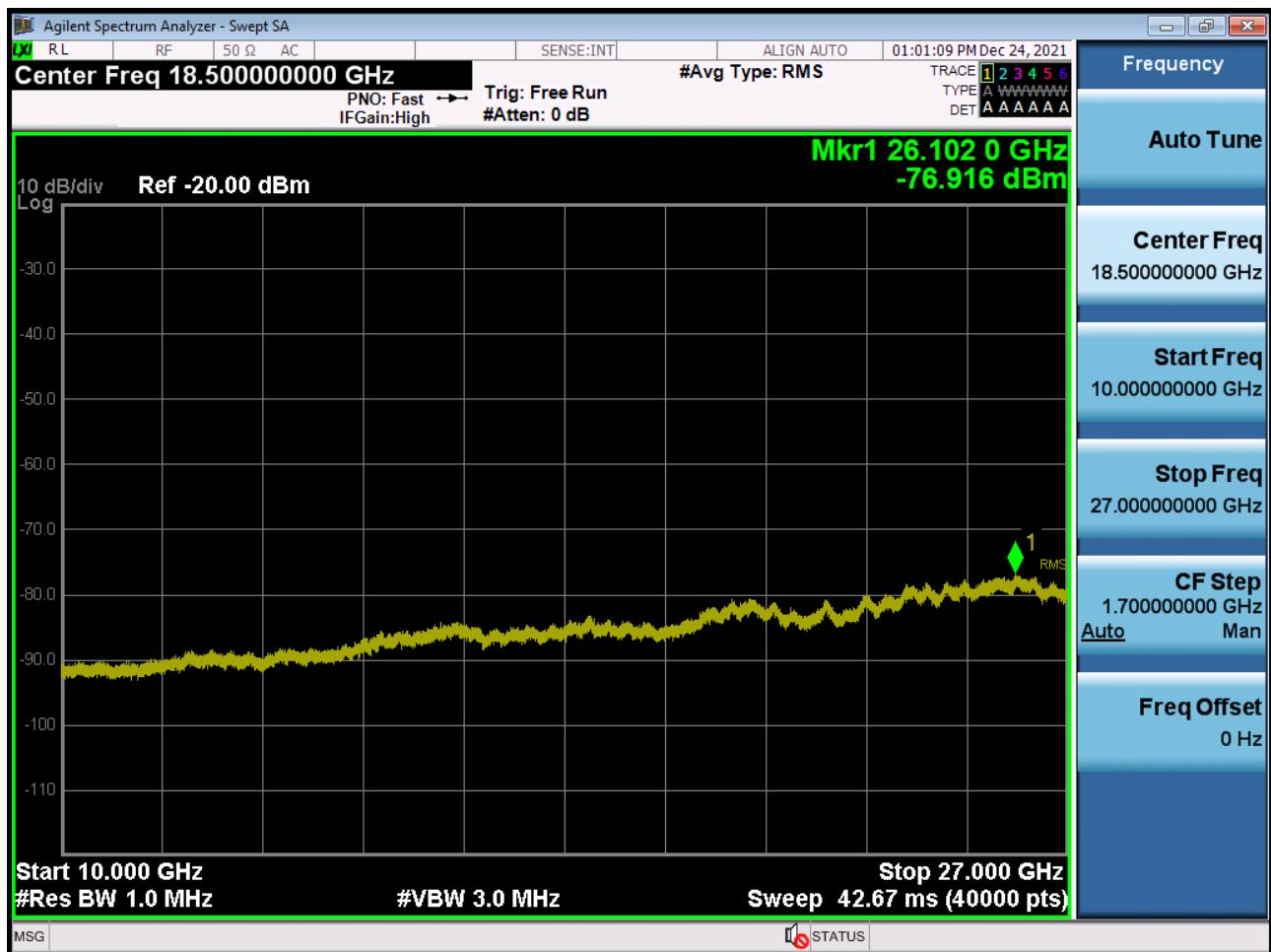
Conducted Spurious Plot 1 (20 MHz Ch.41490 QPSK RB 1, Offset 0) (POWER CLASS 3)
