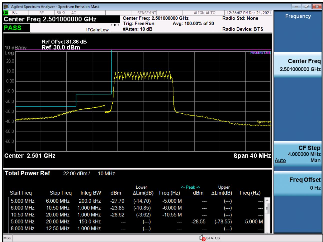
Low Channel Edge Plot (10 MHz Ch.39700 QPSK\_RB50\_Offset 0)-2 (POWER CLASS 3)
