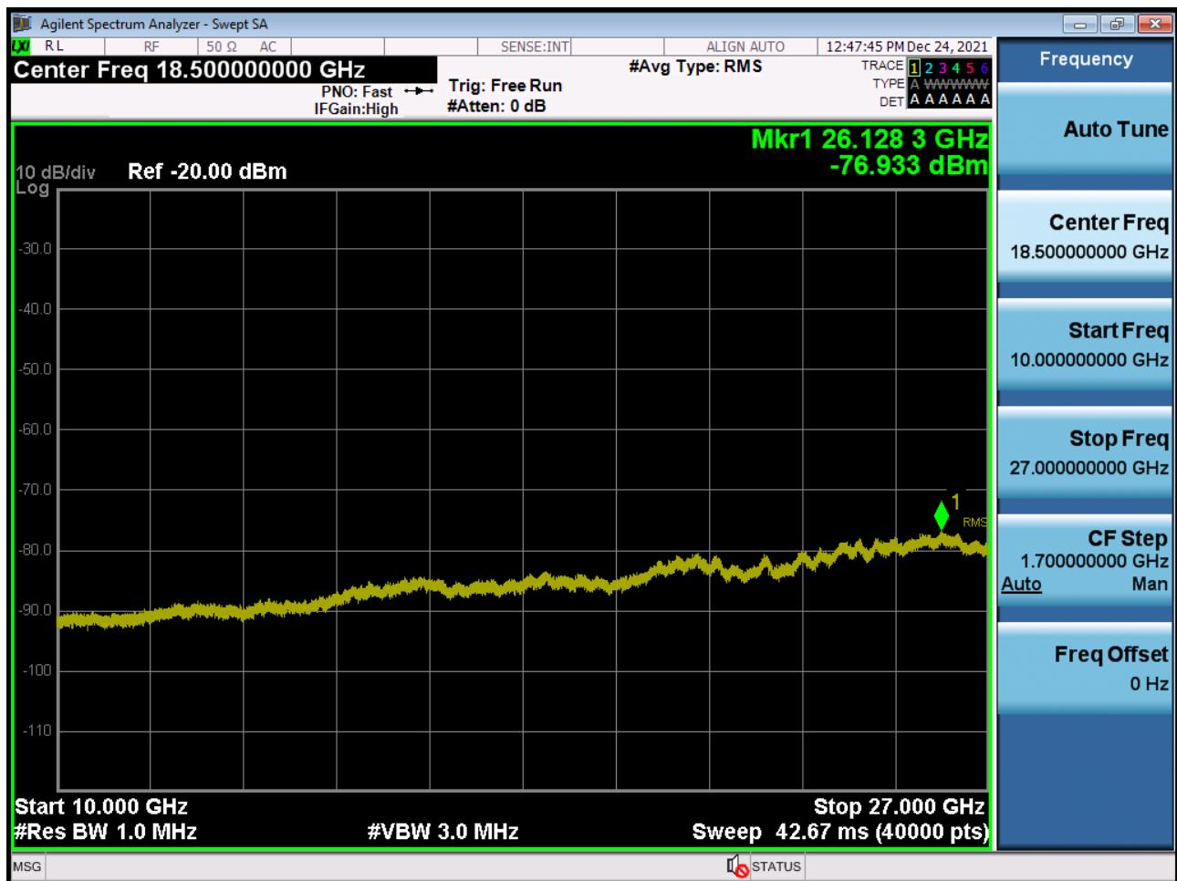
Conducted Spurious Plot 1 (15 MHz Ch.40620 QPSK RB 1, Offset 0) (POWER CLASS 3)
