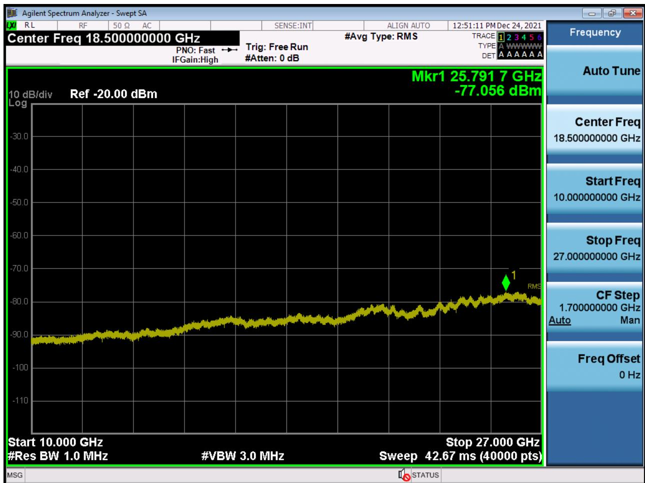
Conducted Spurious Plot 1 (15 MHz Ch.41515 QPSK RB 1, Offset 0) (POWER CLASS 3)
