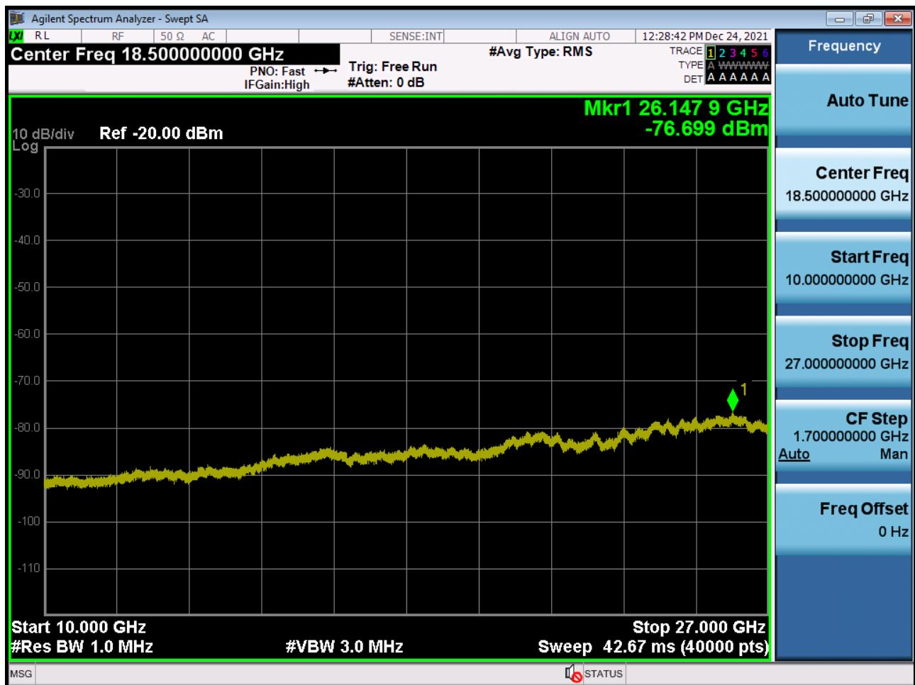
Conducted Spurious Plot 1 (5 MHz Ch.40620 QPSK RB 1, Offset 0) (POWER CLASS 3)
