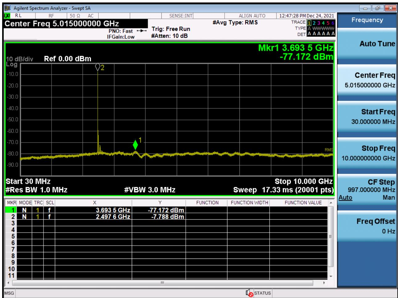
Conducted Spurious Plot 2 (15 MHz Ch. 39725 QPSK RB 1, Offset 0) (POWER CLASS 3)
