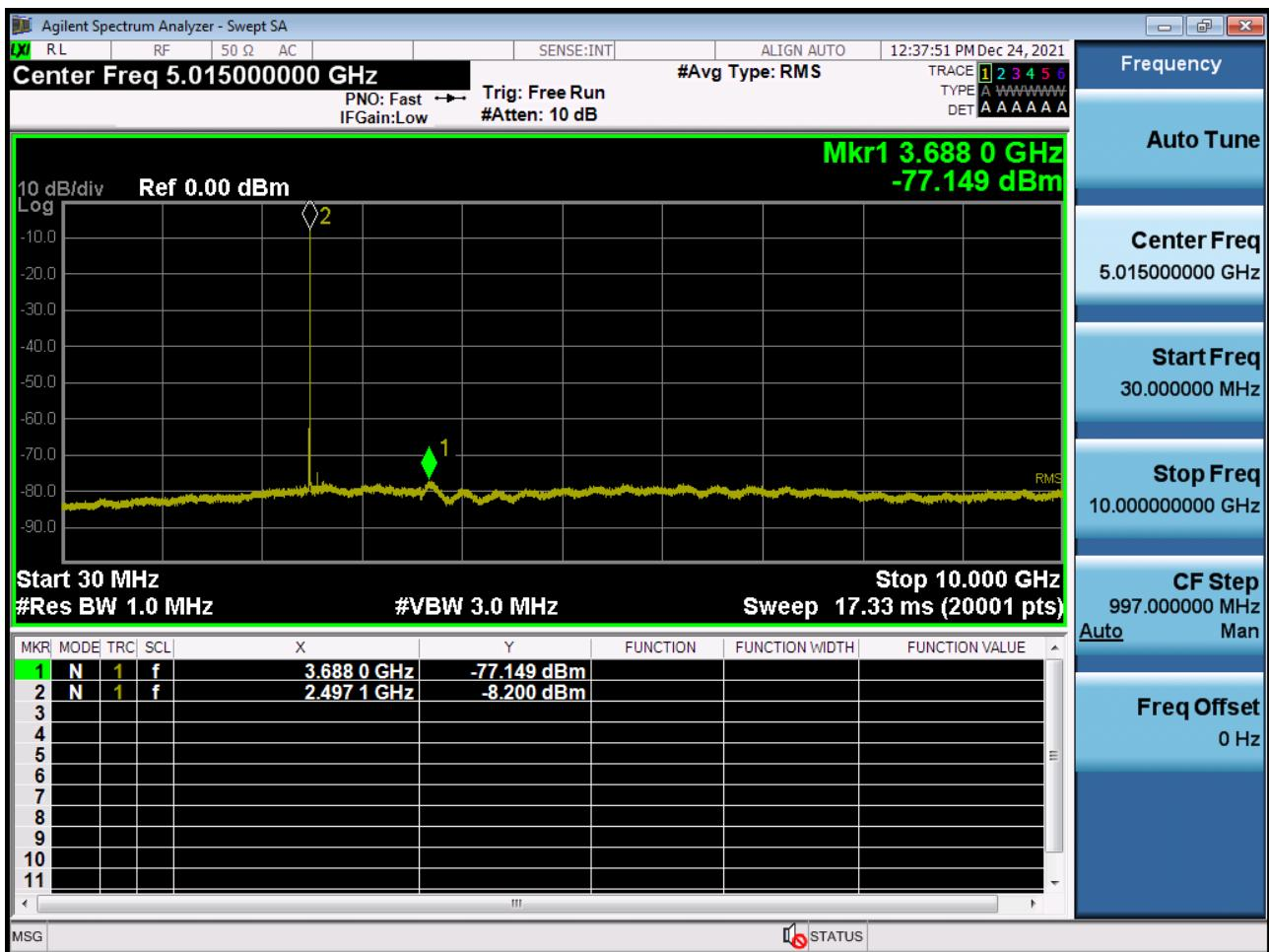
Conducted Spurious Plot 2 (10 MHz Ch. 39700 QPSK RB 1, Offset 0) (POWER CLASS 3)
