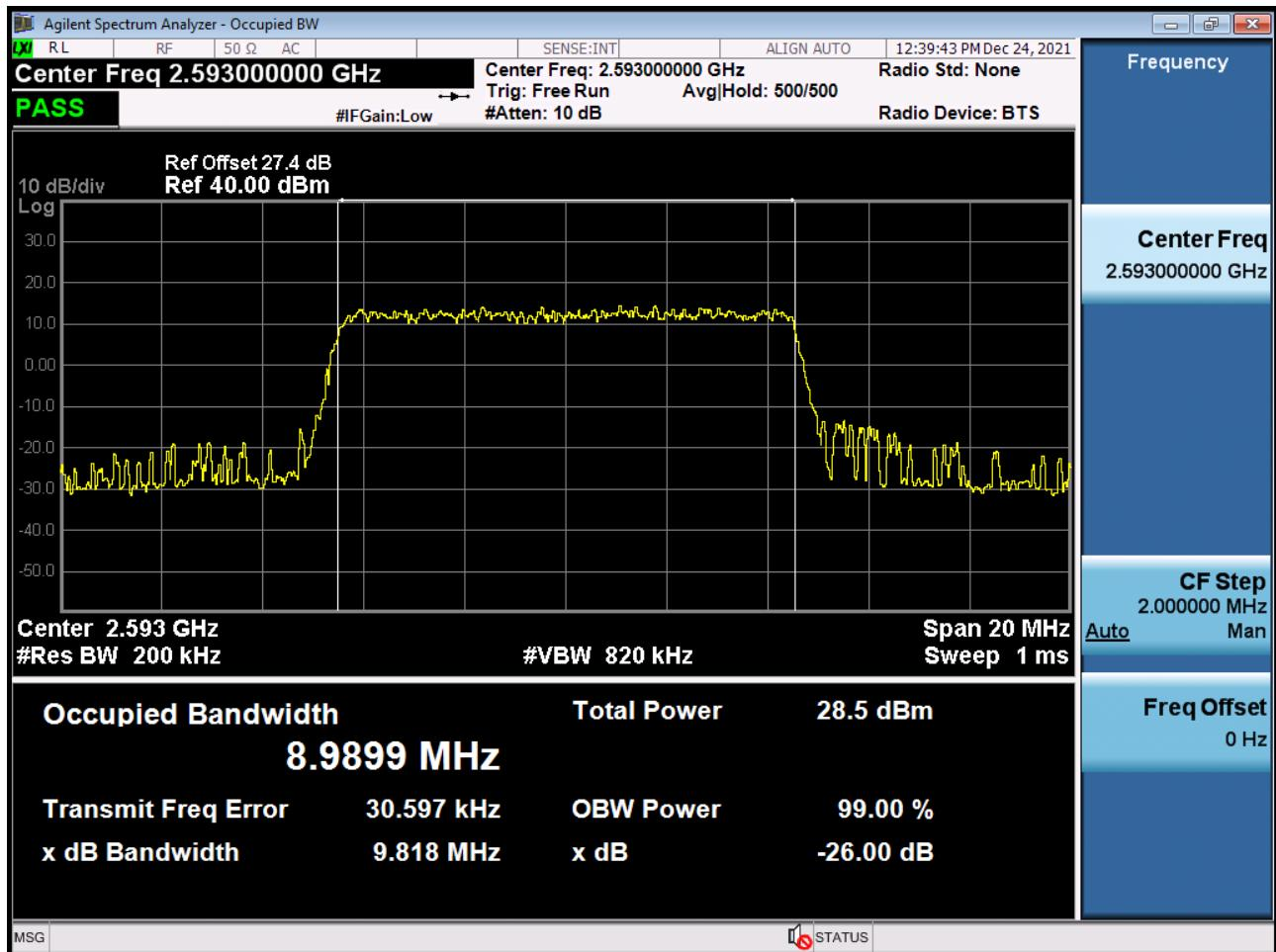
Occupied Bandwidth Plot (15 MHz Ch.40620 QPSK RB 75) (POWER CLASS 3)
