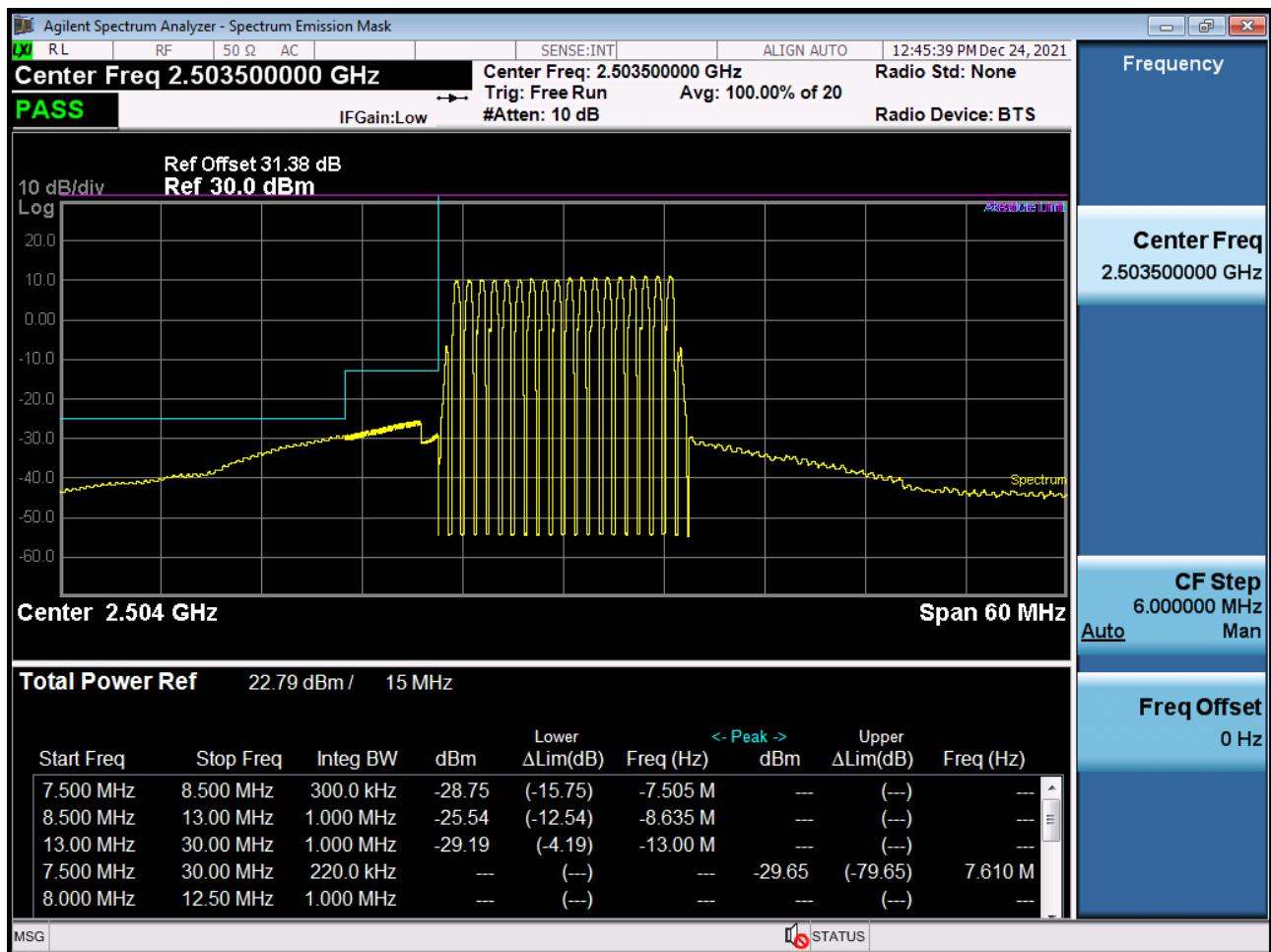
Low Channel Edge Plot (15 MHz Ch.39725 QPSK\_RB75\_Offset 0)-2 (POWER CLASS 3)
