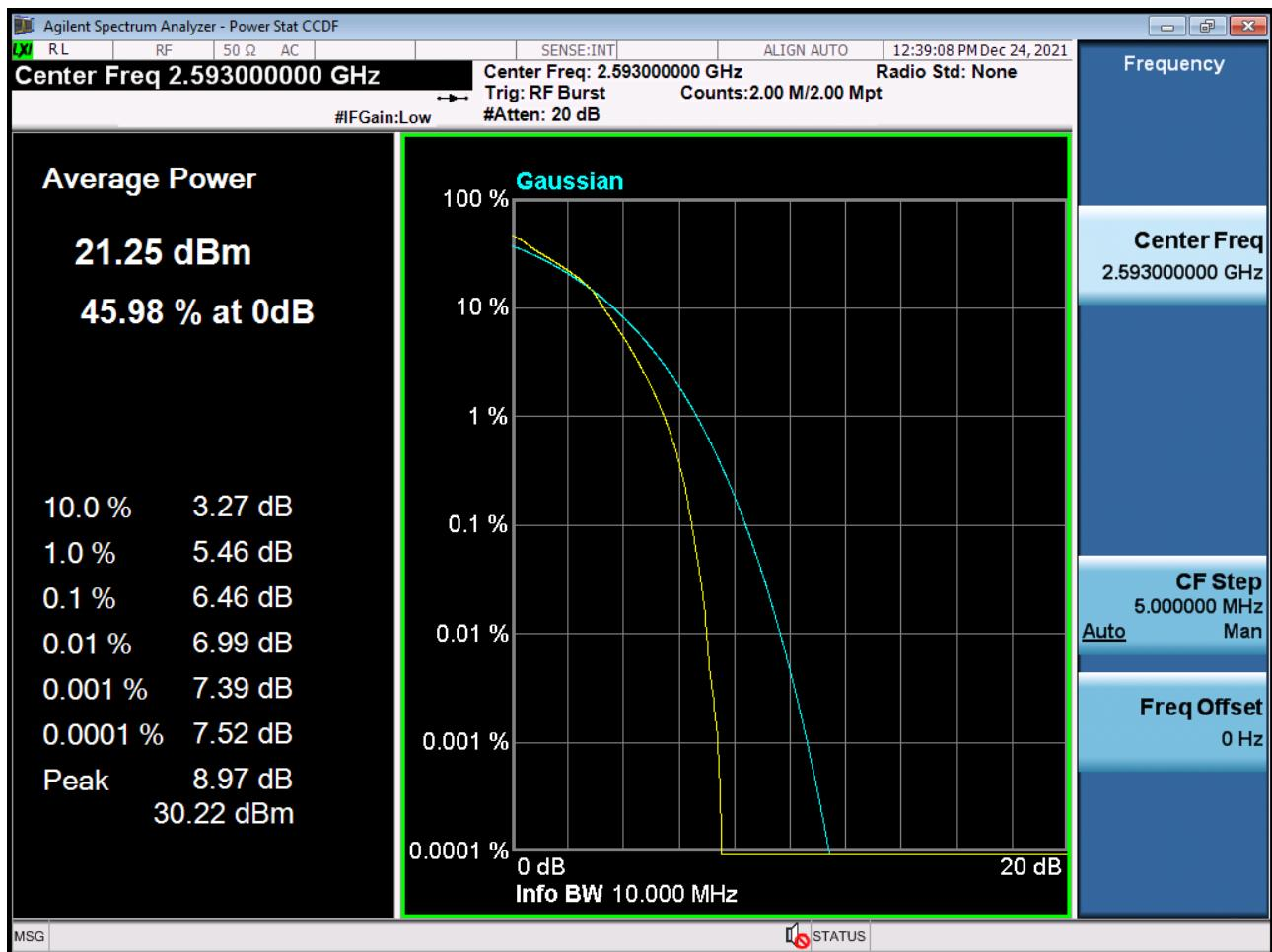
PAR Plot (10 M BW\_Ch.40620\_64QAM\_RB50\_0) (POWER CLASS 3)
