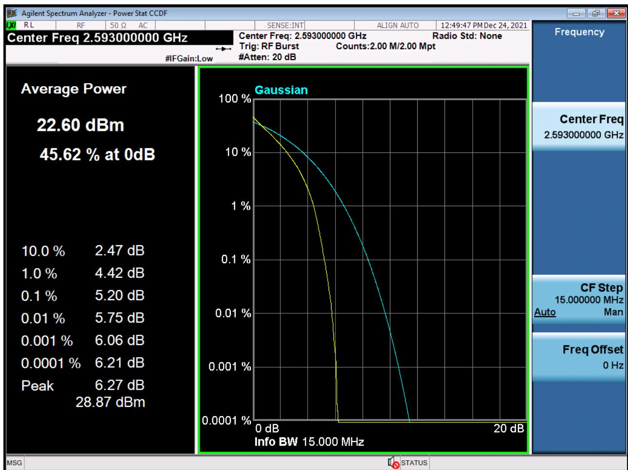
PAR Plot (15 M BW\_Ch.40620\_16QAM\_RB75\_0) (POWER CLASS 3)
