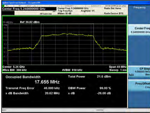
802.11n_HT20 UNII 2C BAND 26 dB Bandwidth(CH 120)
