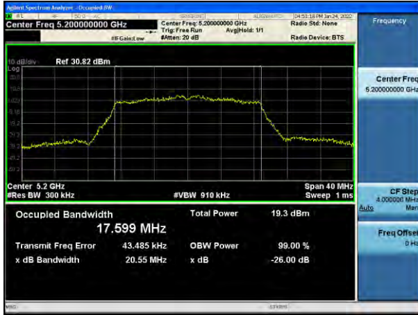
802.11ac_VHT20 UNII 2C BAND 26 dB Bandwidth(CH 144)
