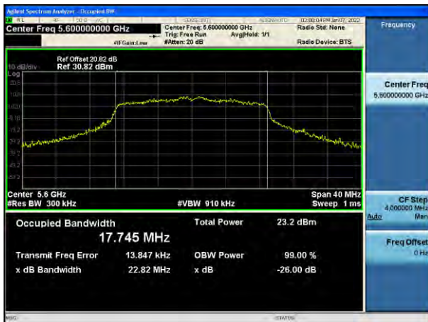
802.11n_HT20 UNII 2C BAND 26 dB Bandwidth(CH 120)
