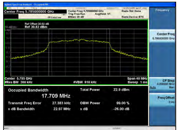
802.11ac_VHT20 UNII 3 BAND 26 dB Bandwidth(CH 157)
