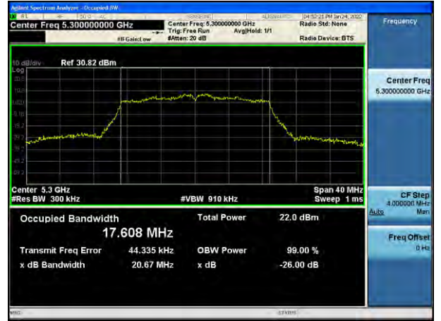
802.11ac_VHT20 UNII 3 BAND 26 dB Bandwidth(CH 157)
