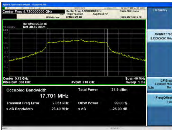
802.11ac_VHT20 UNII 2C BAND 26 dB Bandwidth(CH 144)
