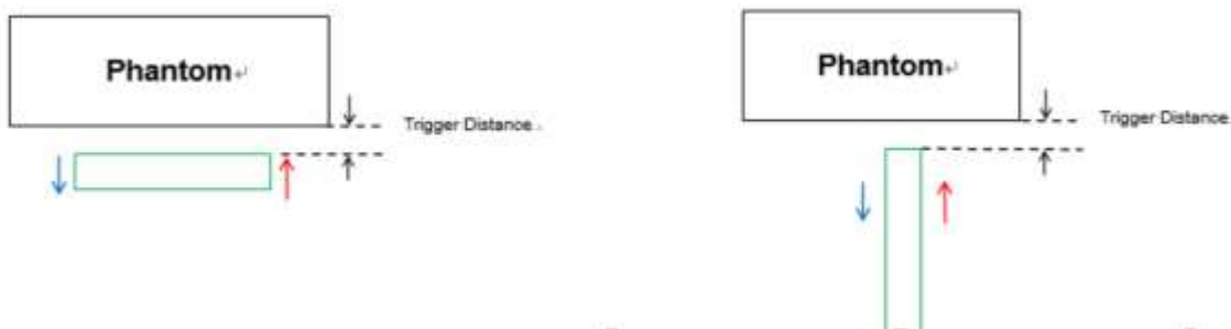
Proximity Sensor Trigger Distance Assessment KDB 616217 D04 §6.2 (Rear /Bottom)
