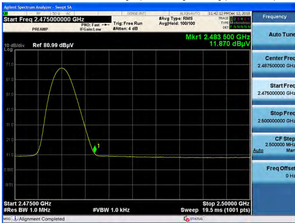
Radiated Restricted Band Edges plot – Average Reading (GFSK, Ch.78)
