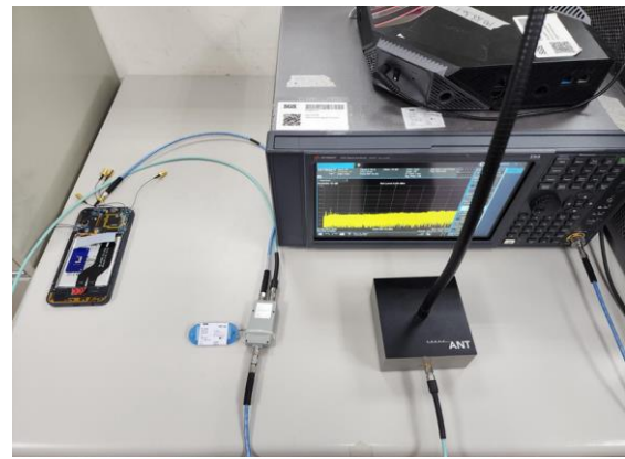
Photograph 8. Test Case 0, 2G SAR TX Mode Change between Normal Mode and Sleep Mode
