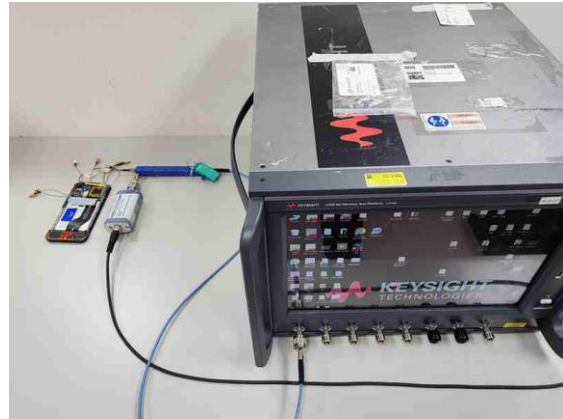
Photograph 4. Test Case 13, Call disconnection and re-establishment
