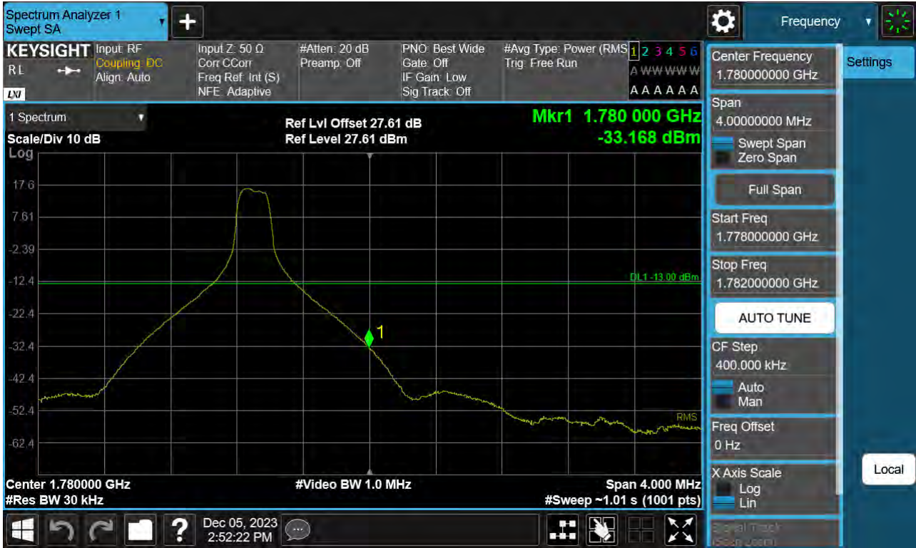
Sub6 n66. Upper Band Edge Plot (30 M BW Ch.353000 BPSK_RB1_Offset 105) -1
