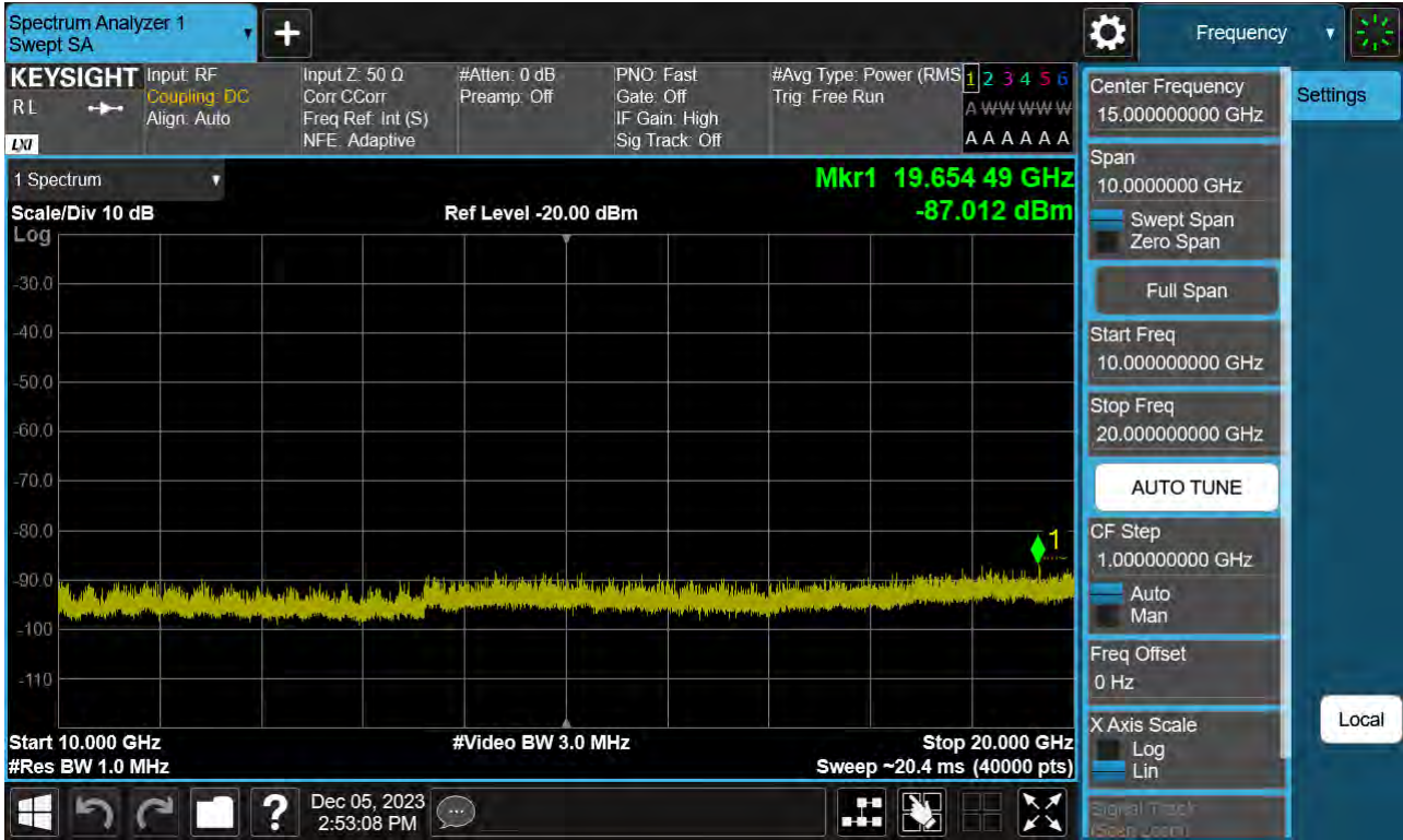
Sub6 n66. Conducted Spurious Plot_2 (353000ch_30 MHz_BPSK_RB 1_1)
