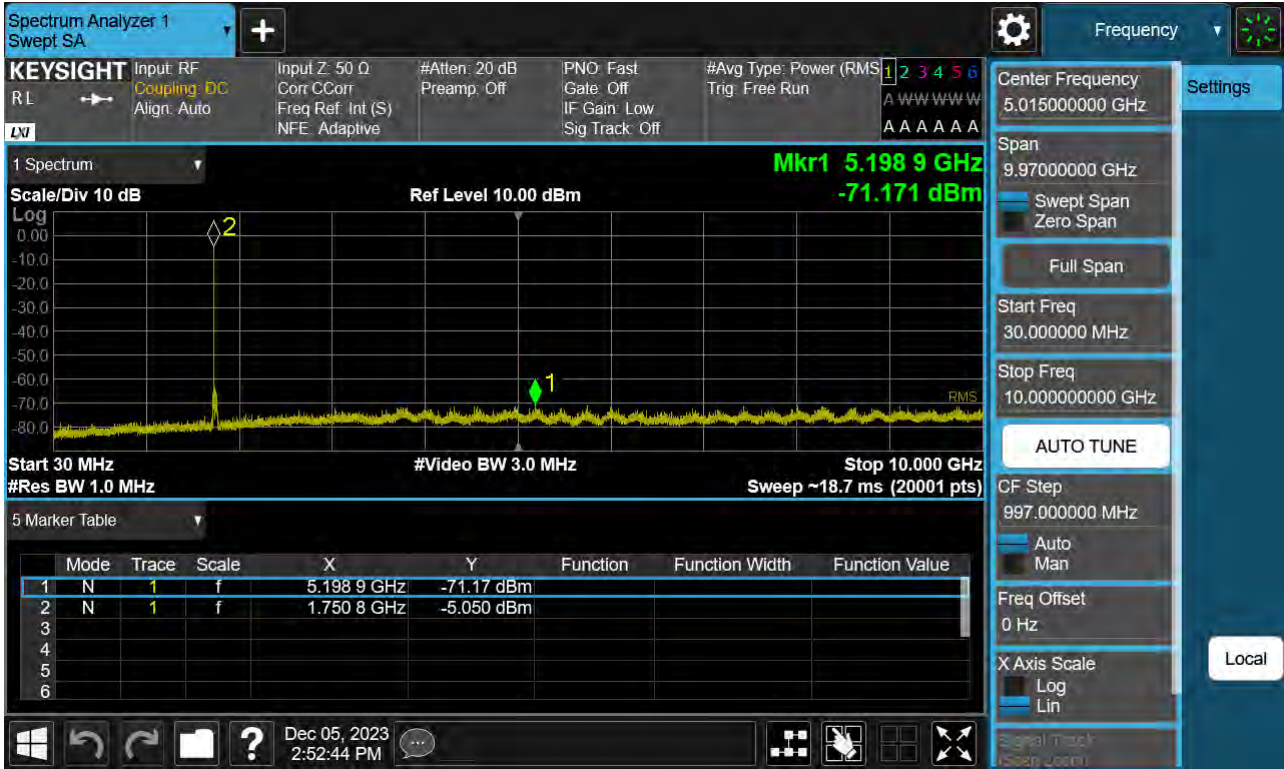
Sub6 n66. Conducted Spurious Plot_1 (353000ch_30 MHz_BPSK_RB 1_1)
