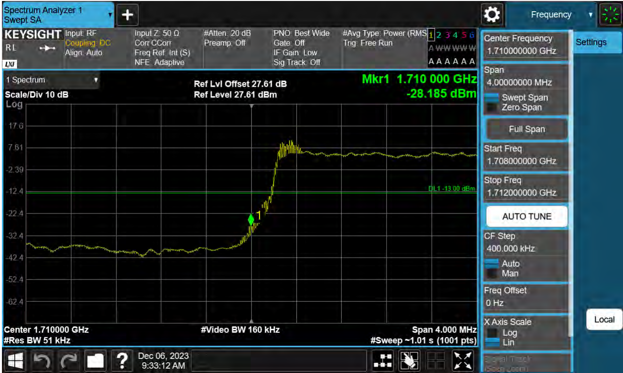
Sub6 n66. Lower Band Edge Plot (5 M BW Ch.342500 BPSK Full RB) -2
