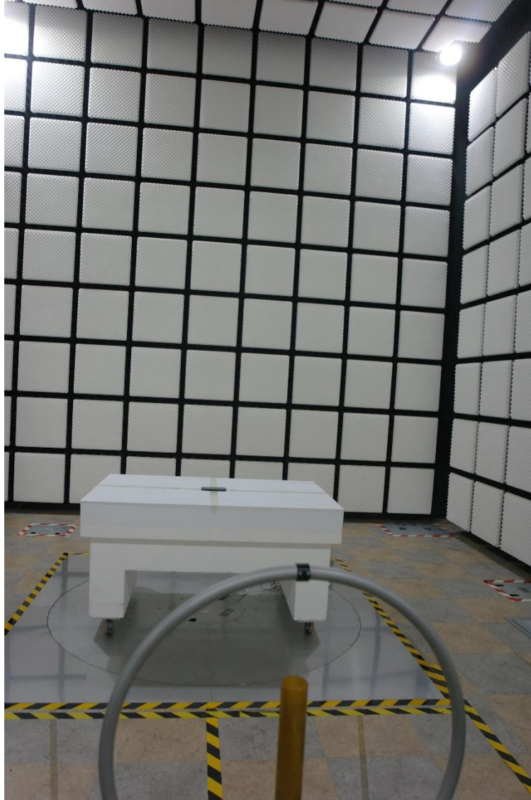
NFC Radiated Test Setup Photo for below 30 MHz:
