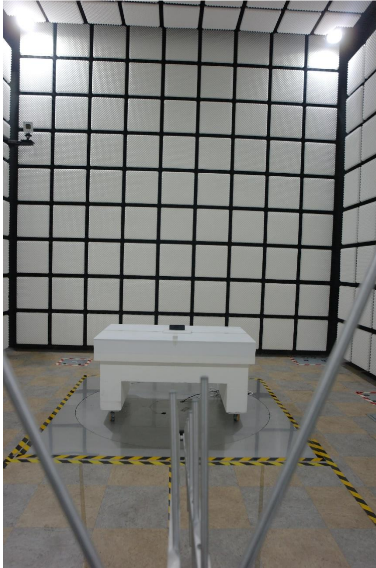
NFC Radiated Test Setup Photo for 30 MHz ~ 1 GHz:
