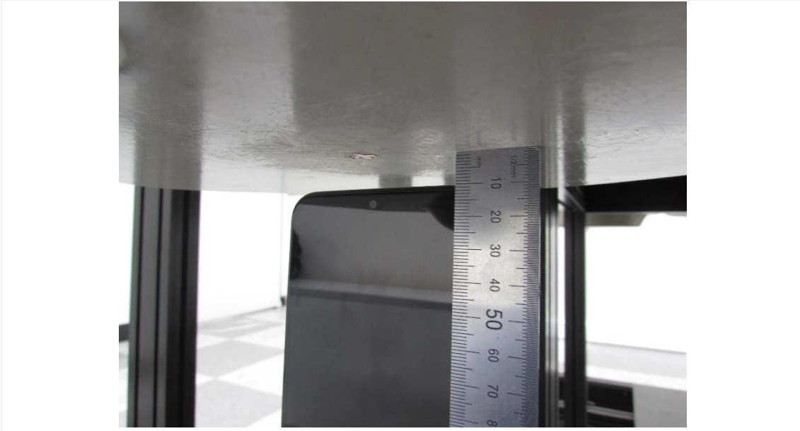
Distance of 10 mm from the EUT
