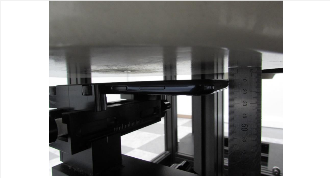
Distance of 10 mm from the EUT
