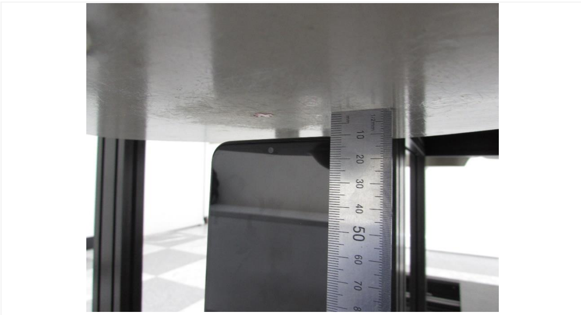
Distance of 10 mm from the EUT
