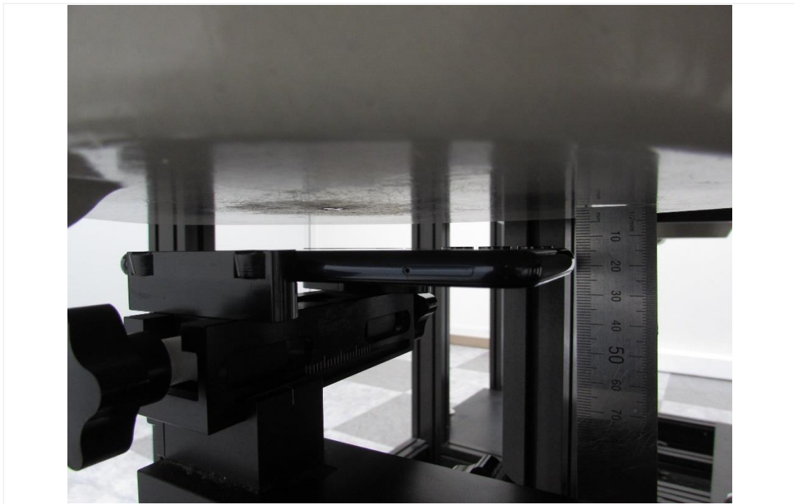
Distance of 15 mm from the EUT
