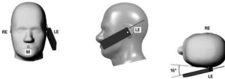
Figure 8.5. Tilt 15° position of the wireless device
