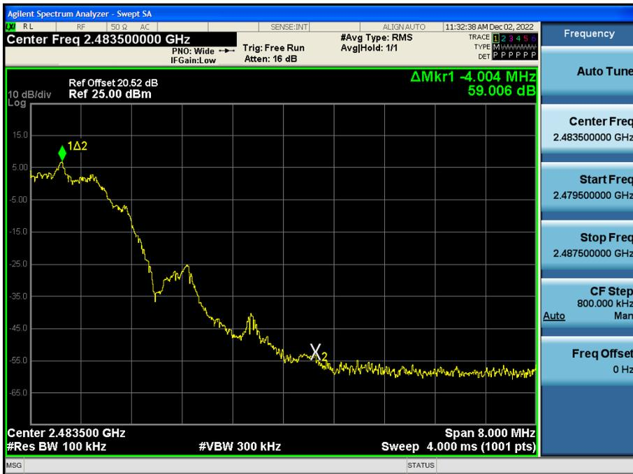
**1M Bit/s (37 Byte) Test Plots -Conducted Spurious Emission**
