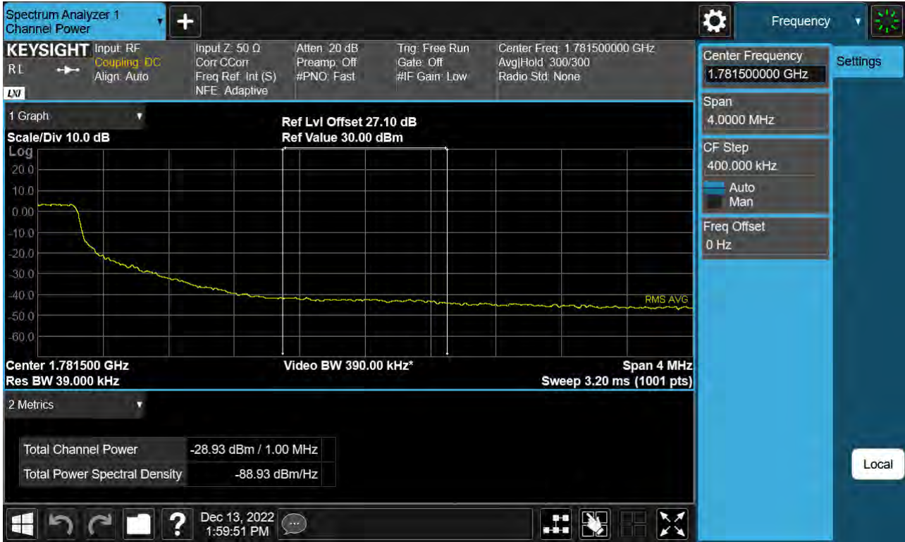
Sub6 n66. Upper Extended Band Edge Plot (5 M BW Ch.355500 BPSK_ Full RB) -3
