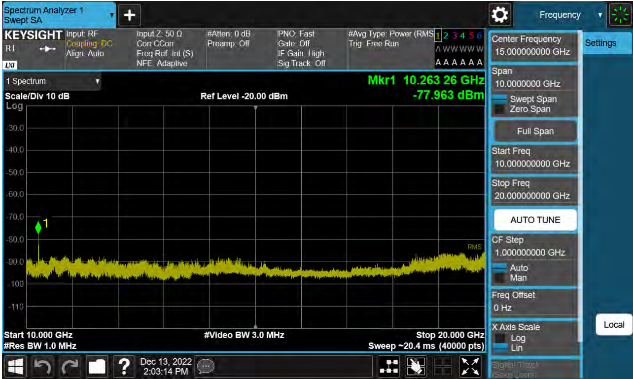
Sub6 n66. Conducted Spurious Plot_2 (343000ch_10 MHz_BPSK_RB 1_1)
