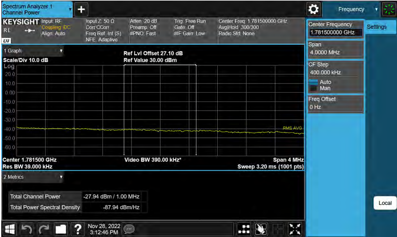
Sub6 n66. Upper Extended Band Edge Plot (20 M BW Ch.354000 BPSK_ Full RB) -3
