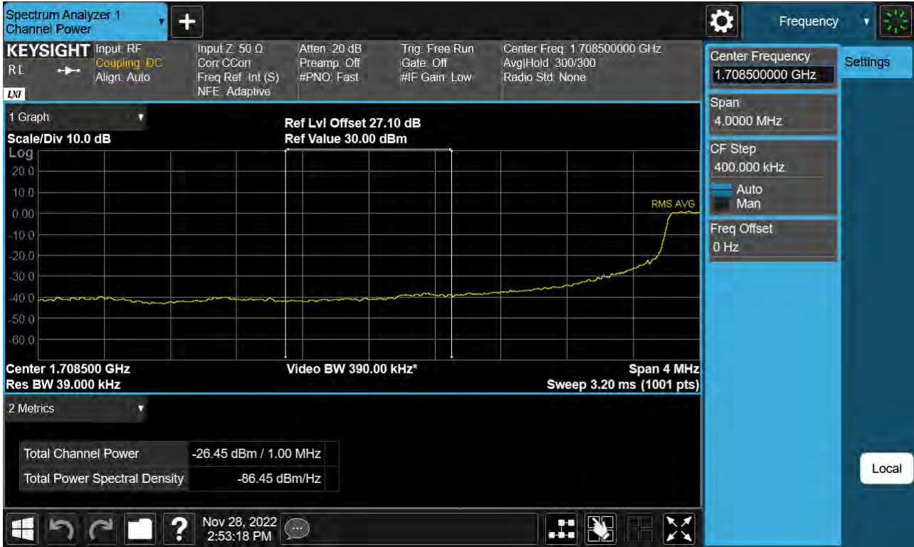
Sub6 n66. Lower Extended Band Edge Plot (10 M BW Ch.343000 BPSK_ Full RB) -3
