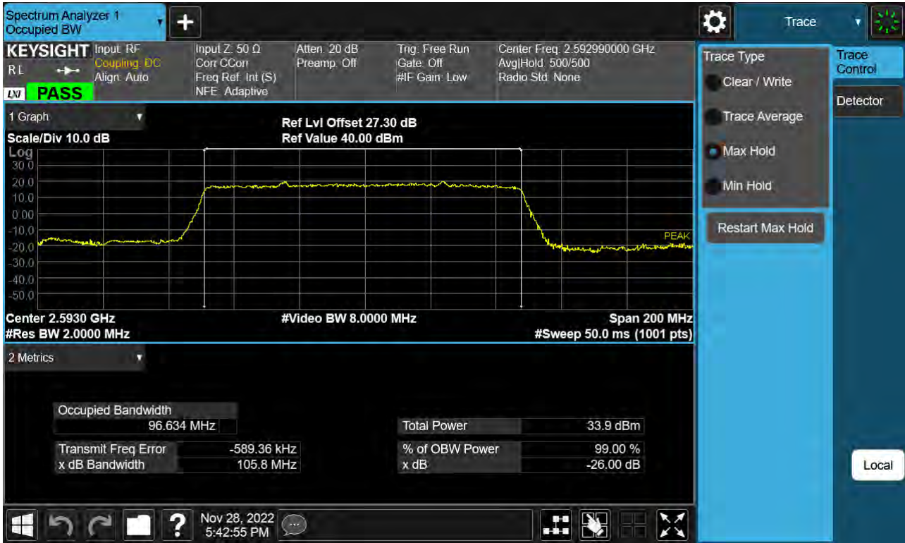
Sub6 n41. Occupied Bandwidth Plot (100 MHz Ch.518598 BPSK)
