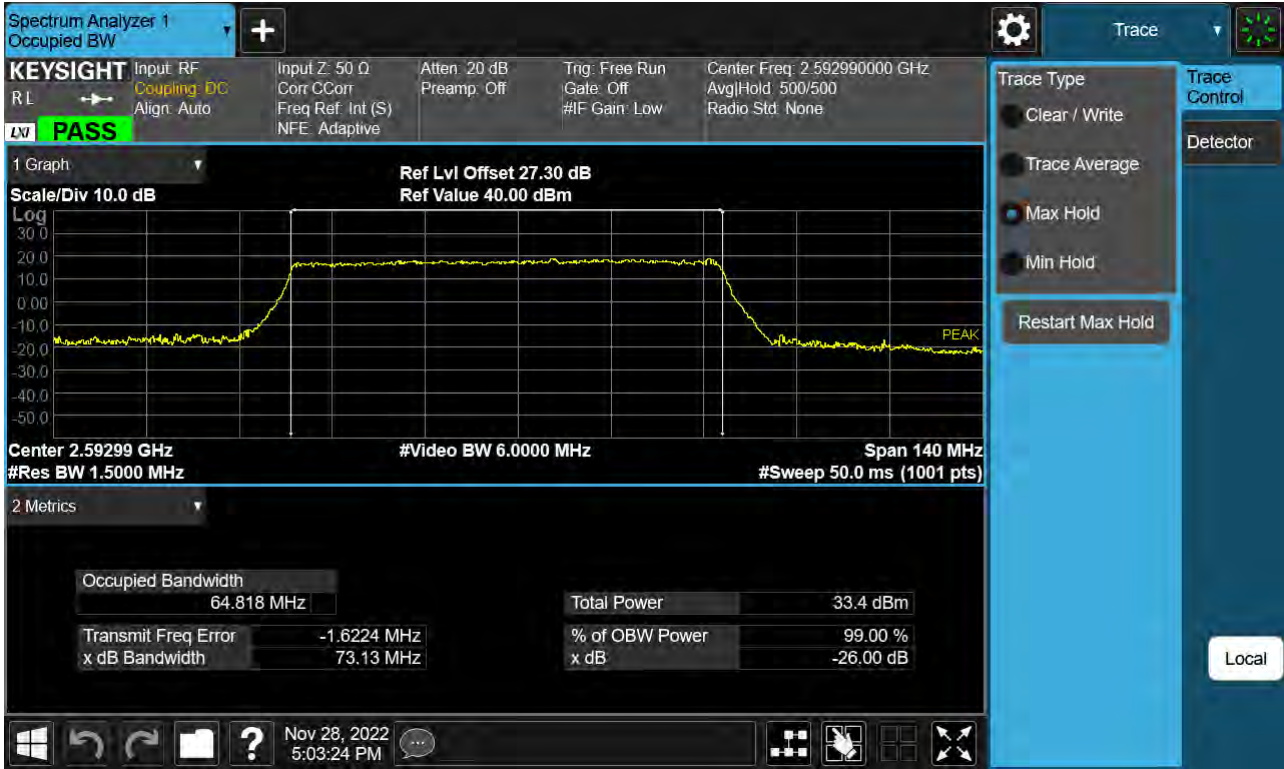
Sub6 n41. Occupied Bandwidth Plot (70 MHz Ch.518598 QPSK )
