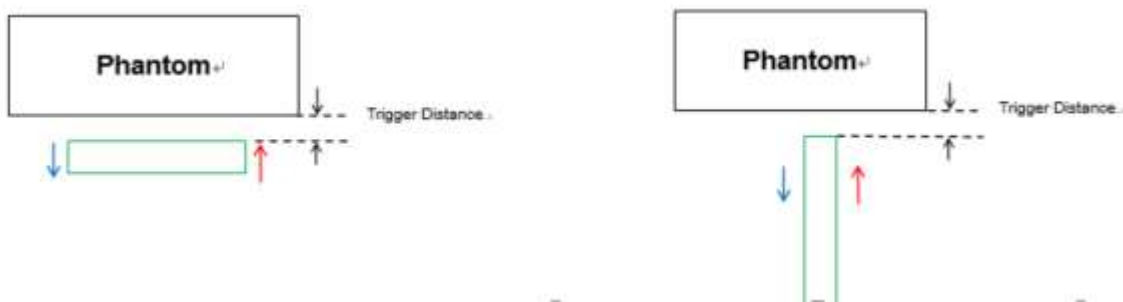
Proximity Sensor Trigger Distance Assessment KDB 616217 D04§6.2
