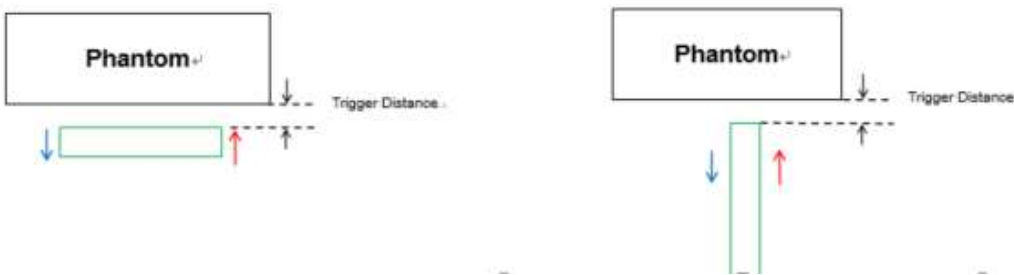
Proximity Sensor Trigger Distance Assessment KDB 616217 D04 §6.2 (Rear /Left side)
