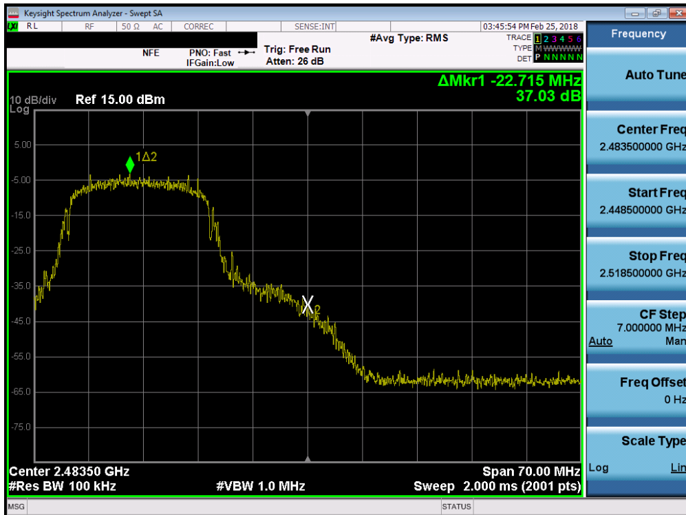
Plot 7-24. Band Edge Plot (802.11n (2.4GHz) – Ch. 11)
