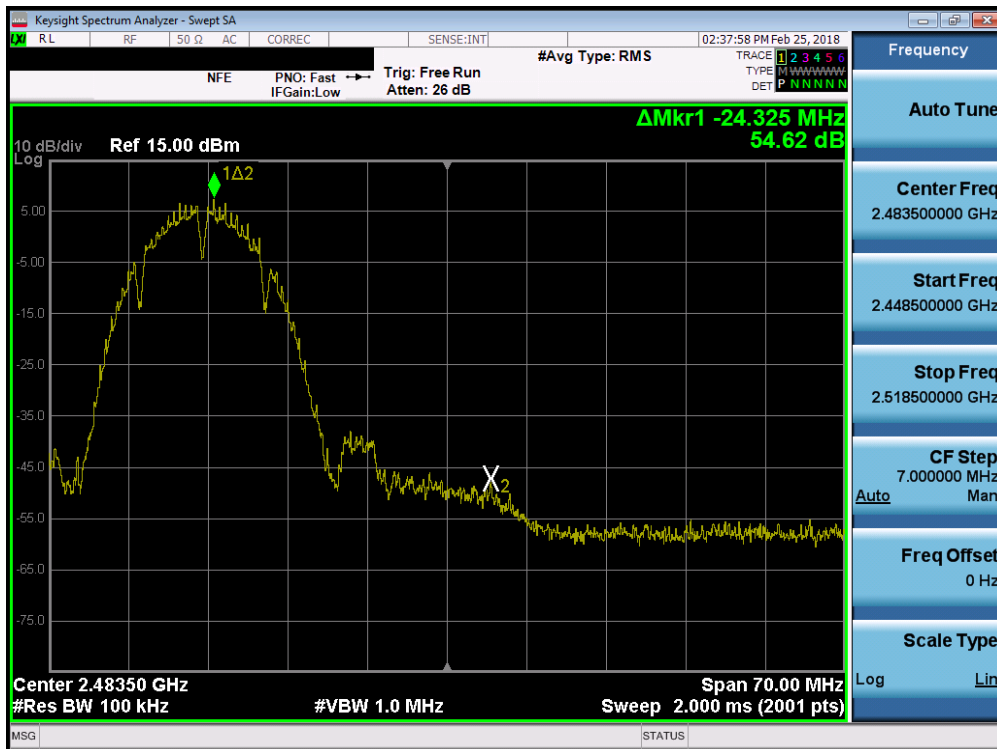
Plot 7-20. Band Edge Plot (802.11b – Ch. 11)
