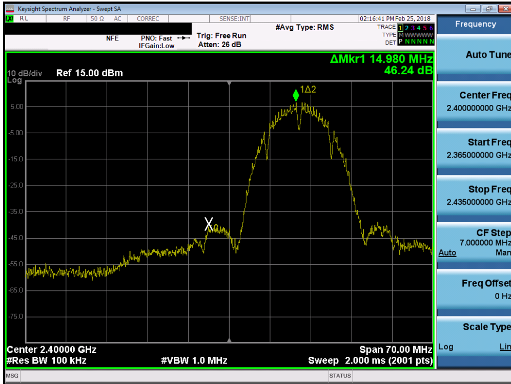
Plot 7-19. Band Edge Plot (802.11b – Ch. 1)
