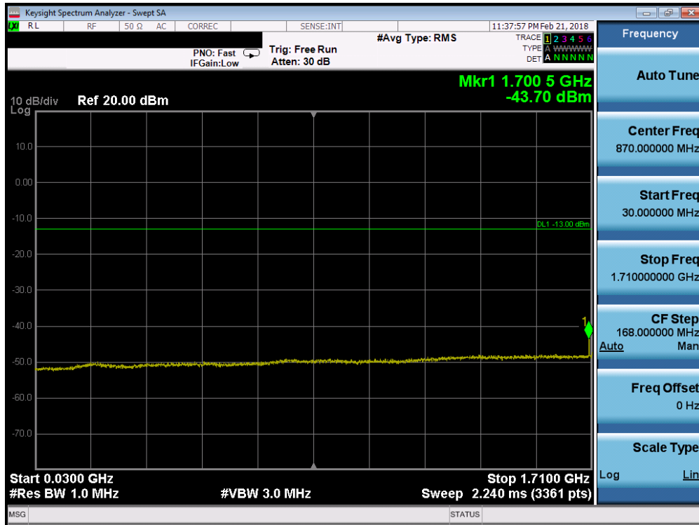
Plot 7-63. Conducted Spurious Plot (Band 4 - 20.0MHz QPSK - RB Size 1, RB Offset 0 - High Channel)
