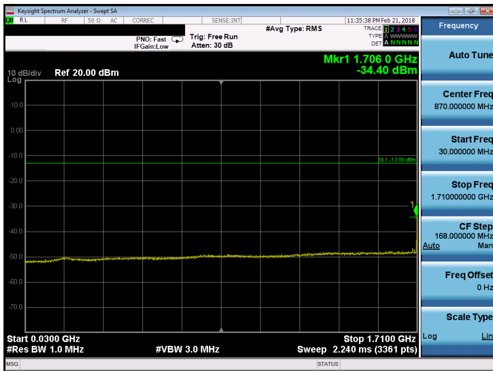
Plot 7-60. Conducted Spurious Plot (Band 4 - 20.0MHz QPSK - RB Size 1, RB Offset 0 - Mid Channel)
