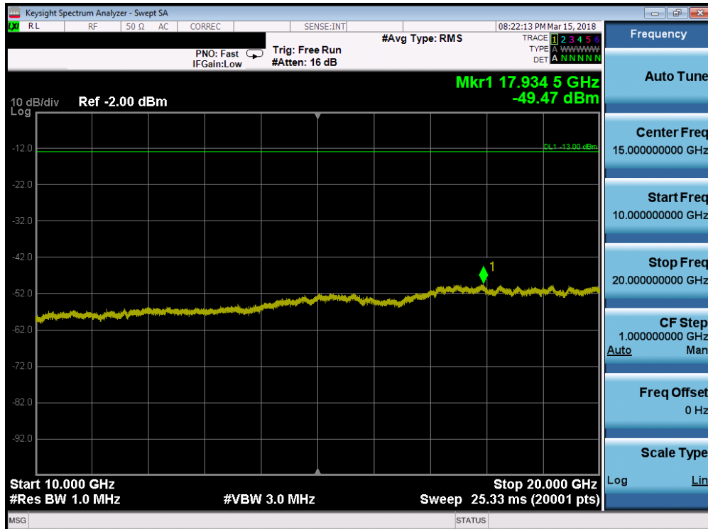
Plot 7-71. Conducted Spurious Plot (Band 2 - 10.0MHz QPSK - RB Size 1, RB Offset 0 - Mid Channel)
