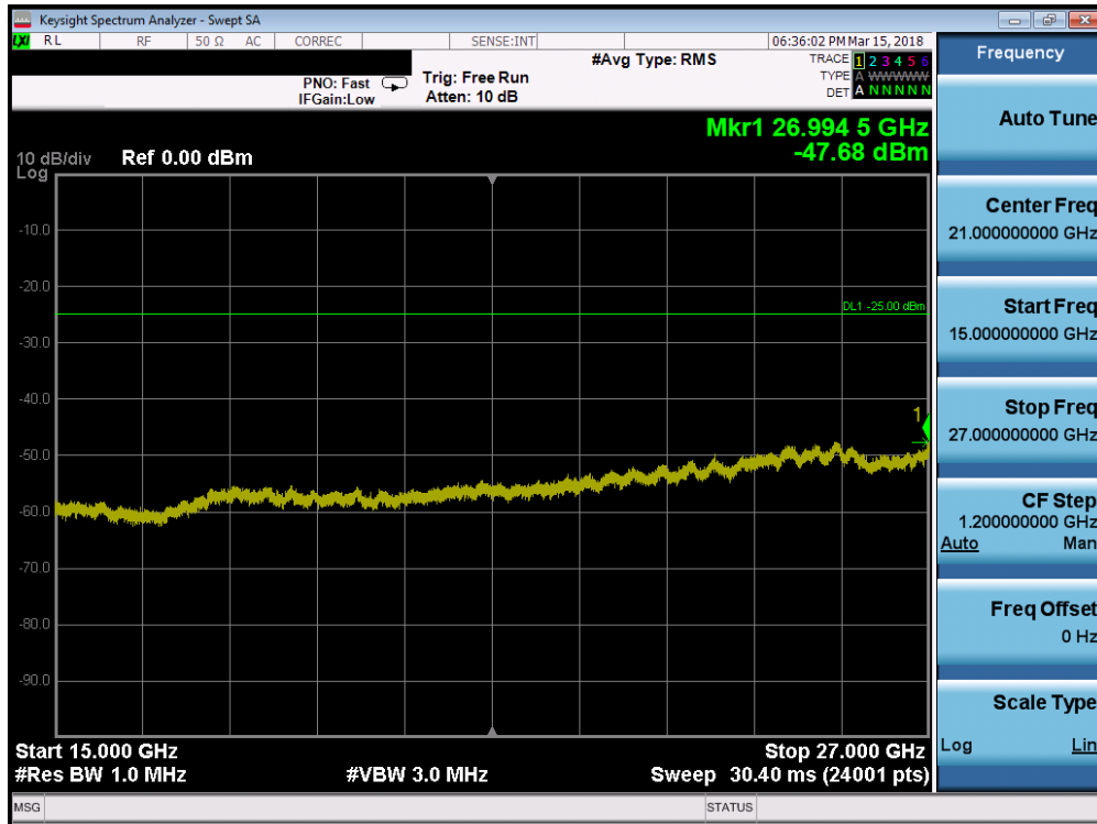
Plot 7-83. Conducted Spurious Plot (Band 7 - 10.0MHz QPSK - RB Size 1, RB Offset 0 - High Channel)
