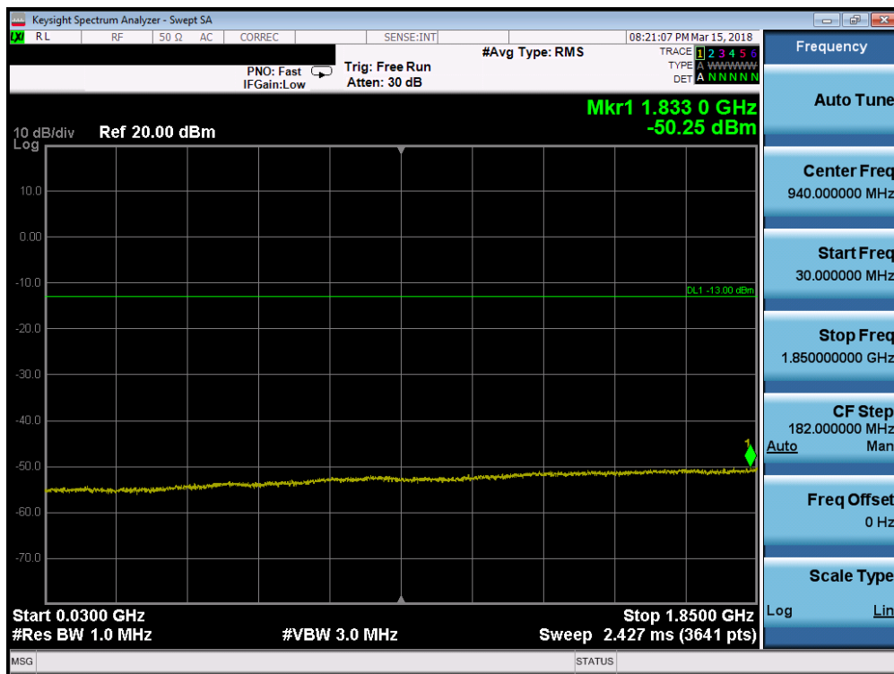
Plot 7-69. Conducted Spurious Plot (Band 2 - 10.0MHz QPSK - RB Size 1, RB Offset 0 - Mid Channel)
