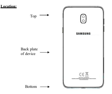
FCC ID is engraved on rear bottom of the device.
