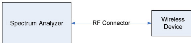
Figure 7-1. Test Instrument & Measurement Setup
