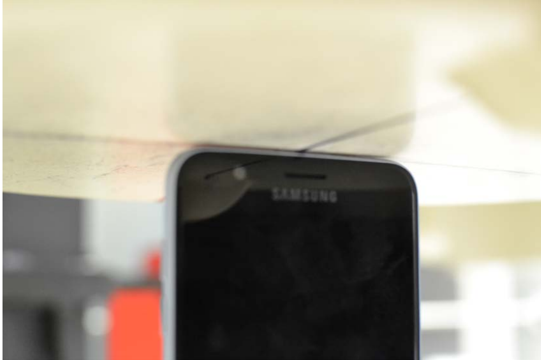
SAR Test Setup Photo 13: Top Edge at 0.0 cm
