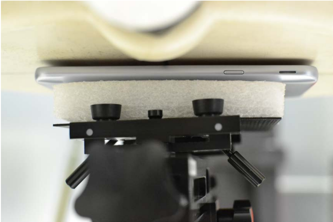
SAR Test Setup Photo 10: Front Side at 0.2 cm
