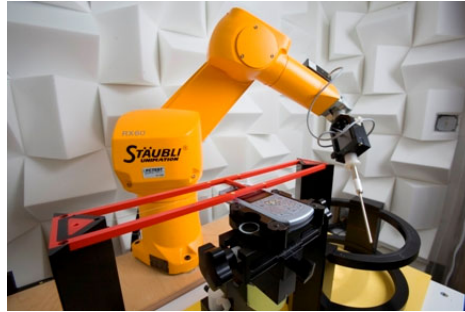
Figure 4-3 SPEAG Robotic System
