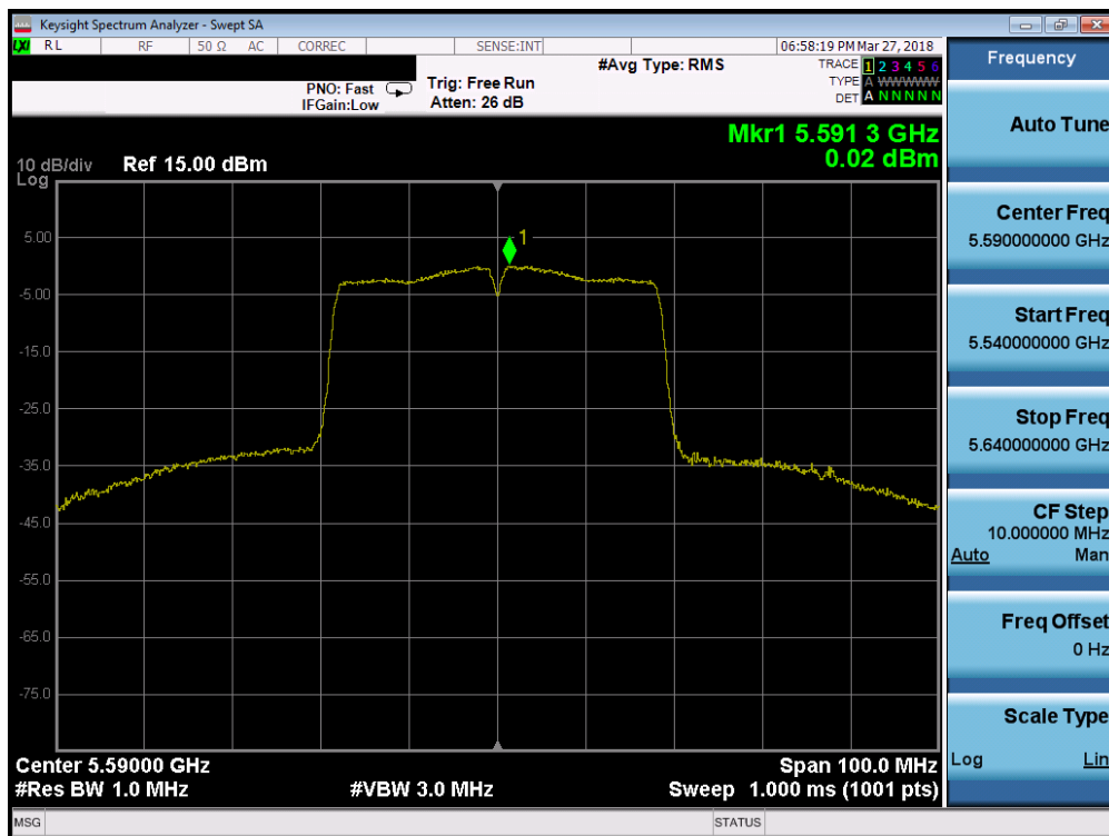
Plot 7-65. Power Spectral Density Plot (40MHz BW 802.11n (UNII Band 2C) – Ch. 118)
