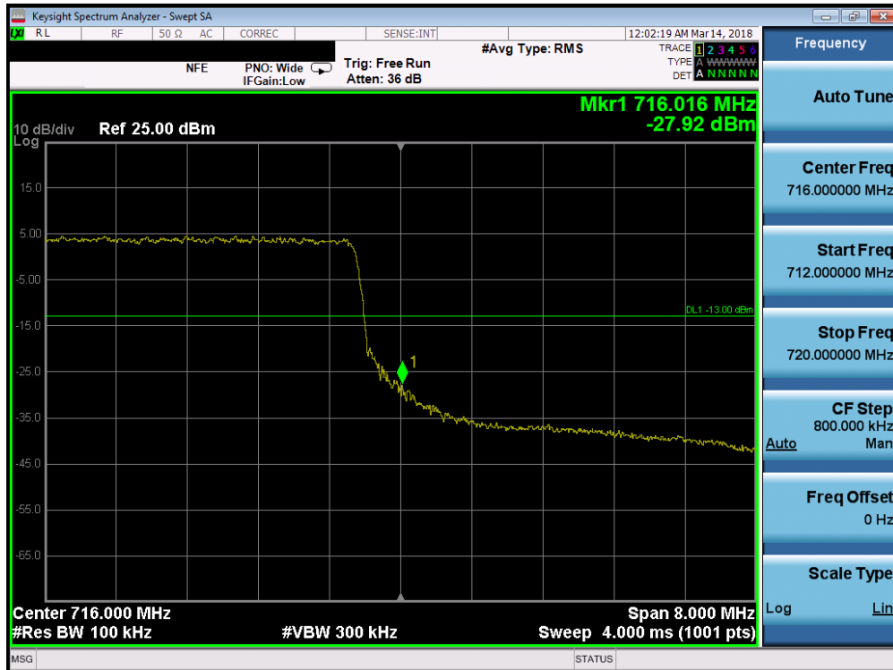
Plot 7-126. Upper Band Edge Plot (Band 12 - 10.0MHz QPSK - Full RB Configuration)
