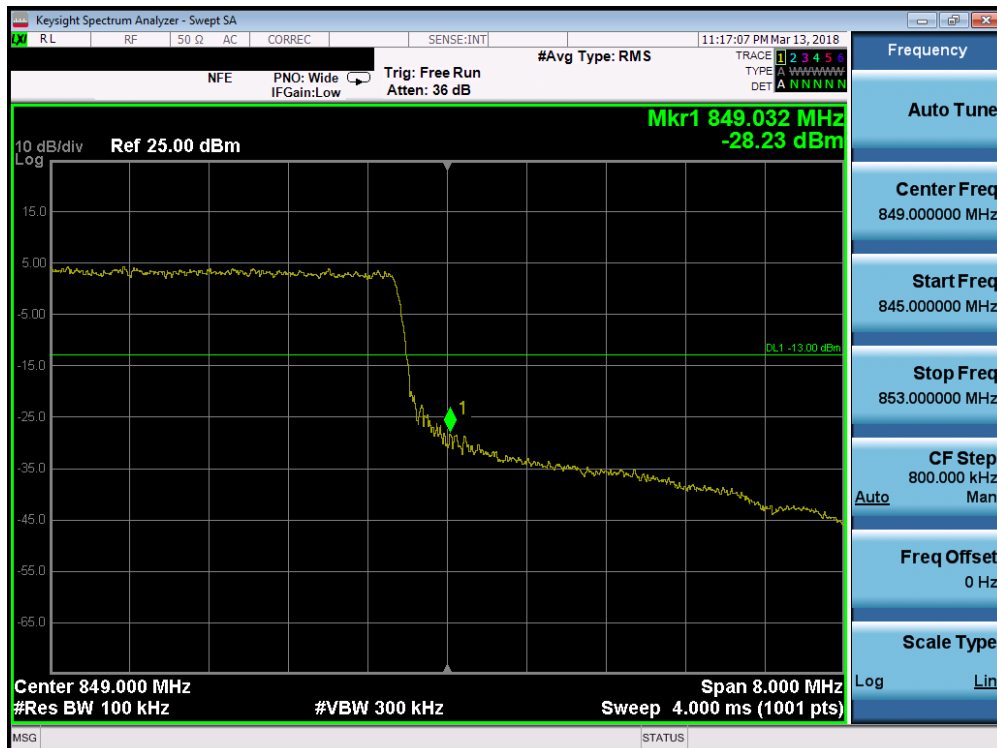
Plot 7-136. Upper Band Edge Plot (Band 5 - 10.0MHz QPSK - Full RB Configuration)
