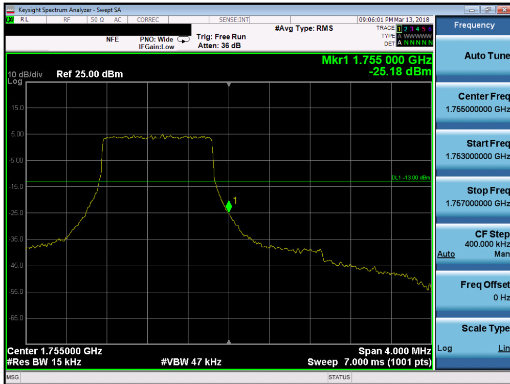
Plot 7-139. Upper Band Edge Plot (Band 4 - 1.4MHz QPSK - Full RB Configuration)
