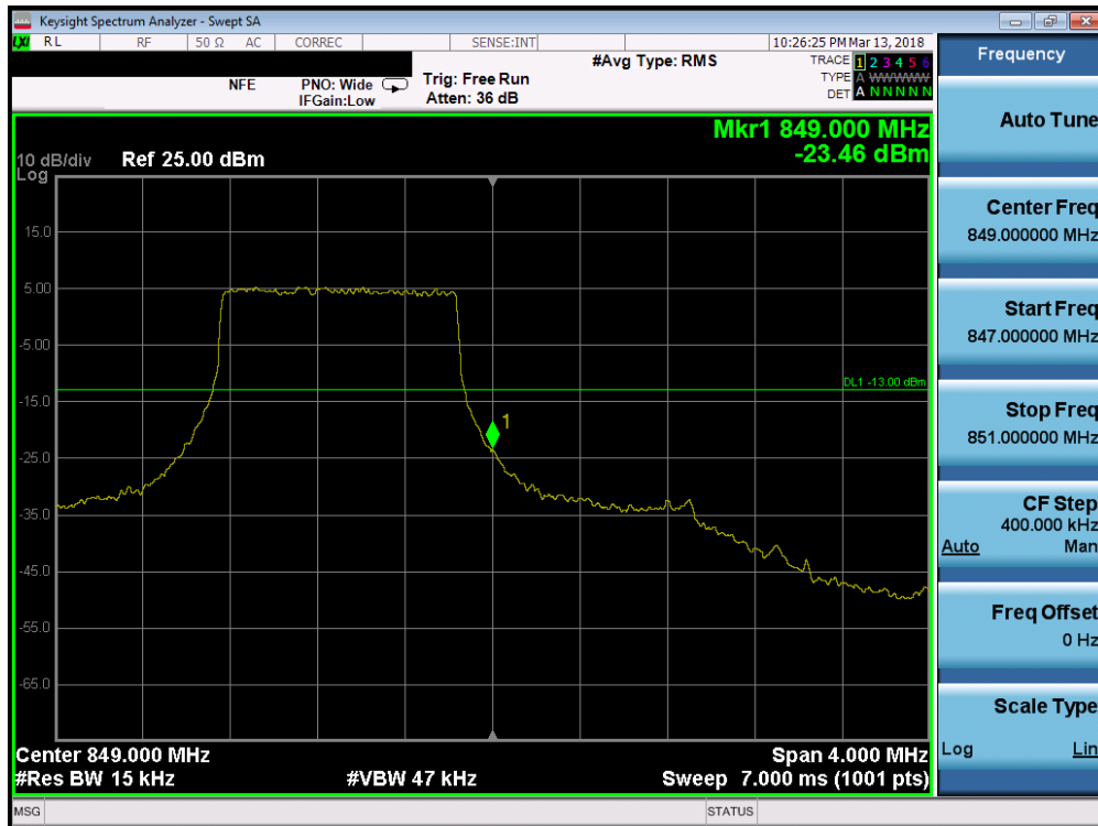
Plot 7-129. Upper Band Edge Plot (Band 5 - 1.4MHz QPSK - Full RB Configuration)
