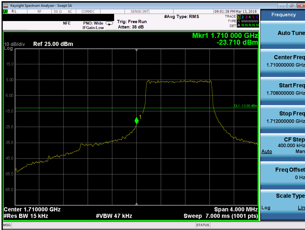
Plot 7-137. Lower Band Edge Plot (Band 66/4 - 1.4MHz QPSK - Full RB Configuration)
