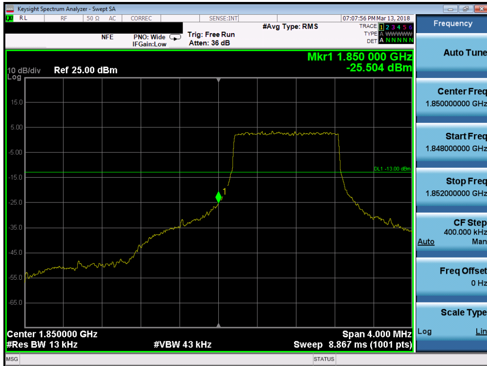
Plot 7-173. Lower Band Edge Plot (Band 2 - 1.4MHz QPSK - Full RB Configuration)
