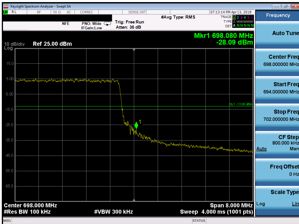
Plot 7-114. Upper Band Edge Plot (Band 71 - 10.0MHz QPSK - Full RB Configuration)
