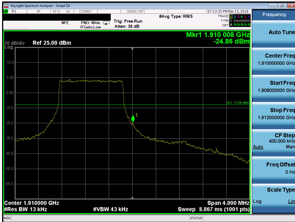
Plot 7-175. Upper Band Edge Plot (Band 2 - 1.4MHz QPSK - Full RB Configuration)
