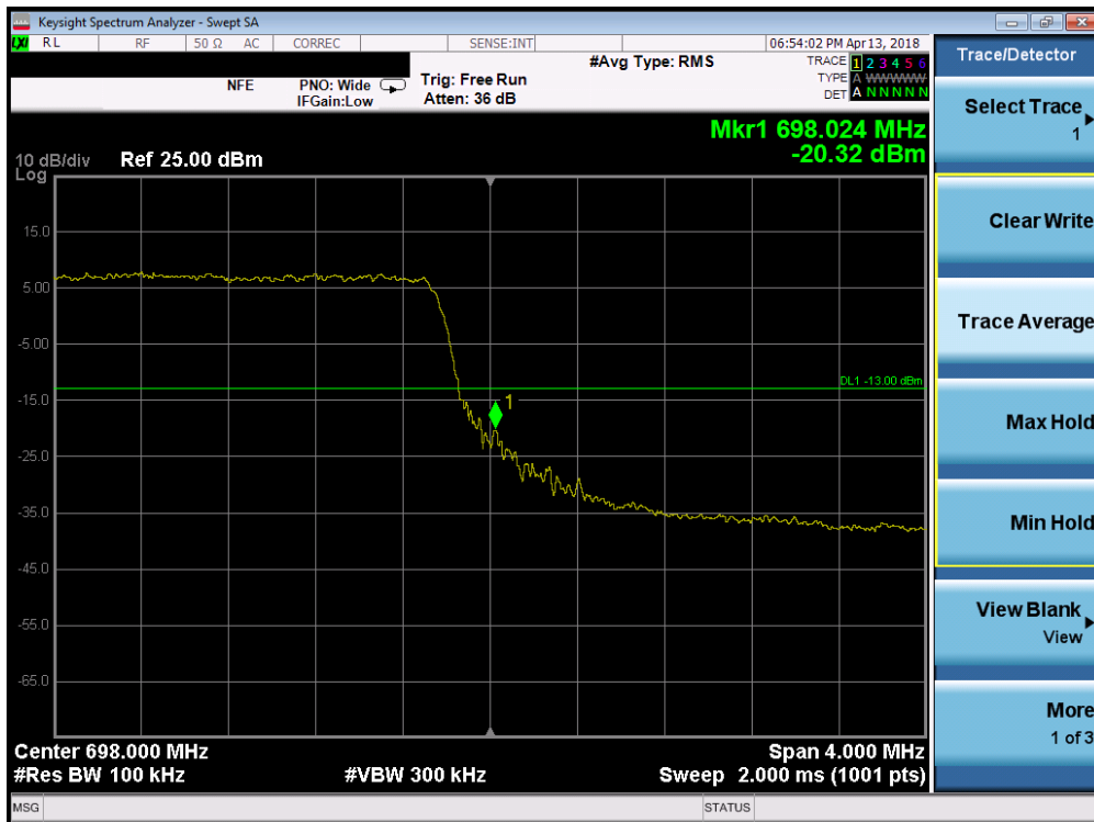
Plot 7-112. Upper Band Edge Plot (Band 71 - 5.0MHz QPSK - Full RB Configuration)
