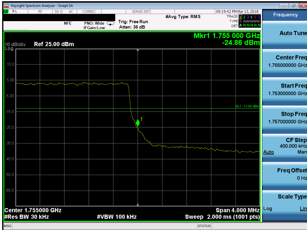
Plot 7-145. Upper Band Edge Plot (Band 4 - 3.0MHz QPSK - Full RB Configuration)
