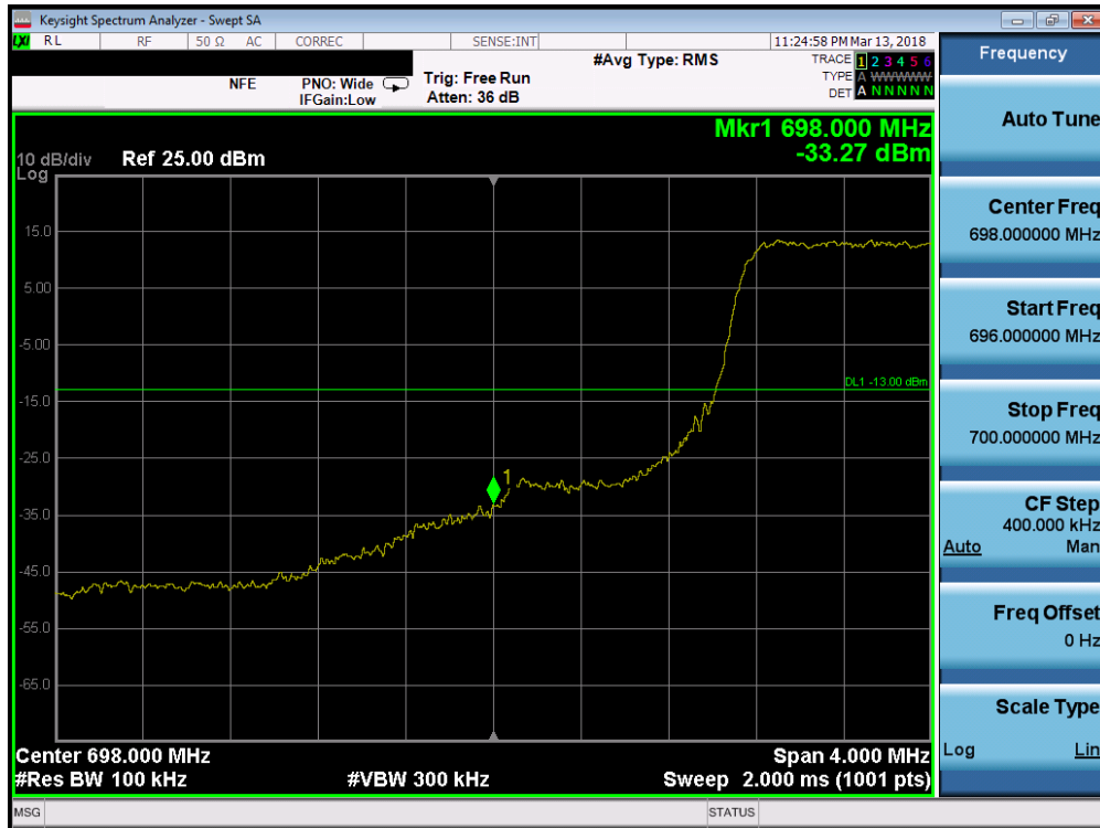
Plot 7-119. Lower Band Edge Plot (Band 12 - 1.4MHz QPSK - Full RB Configuration)
