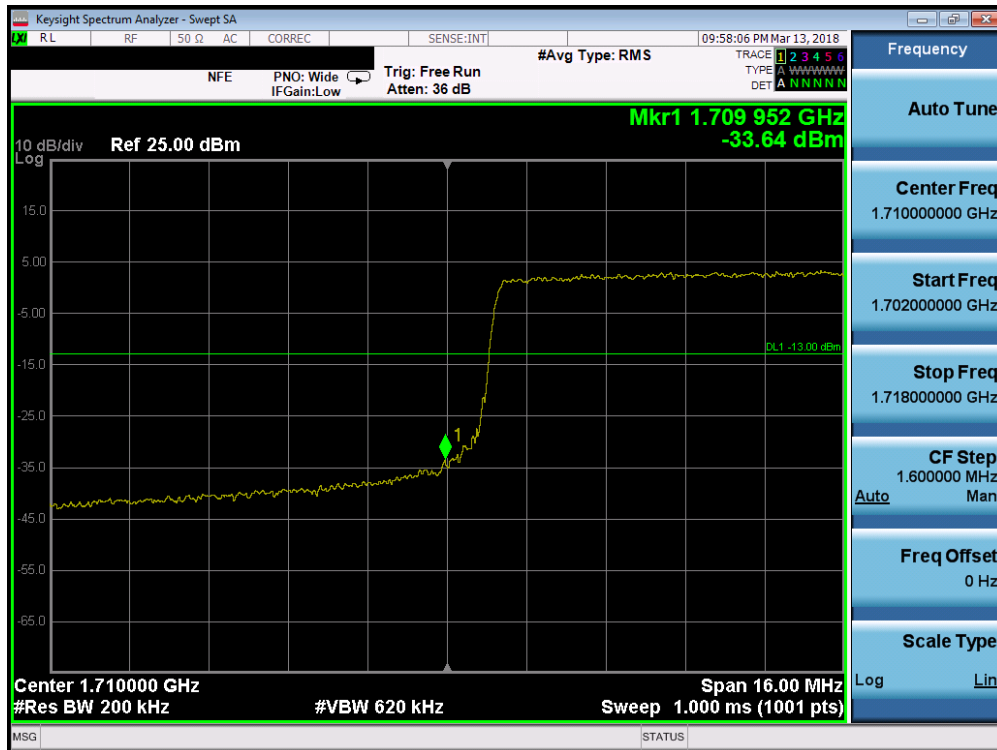
Plot 7-167. Lower Band Edge Plot (Band 66/4 - 20.0MHz QPSK - Full RB Configuration)
