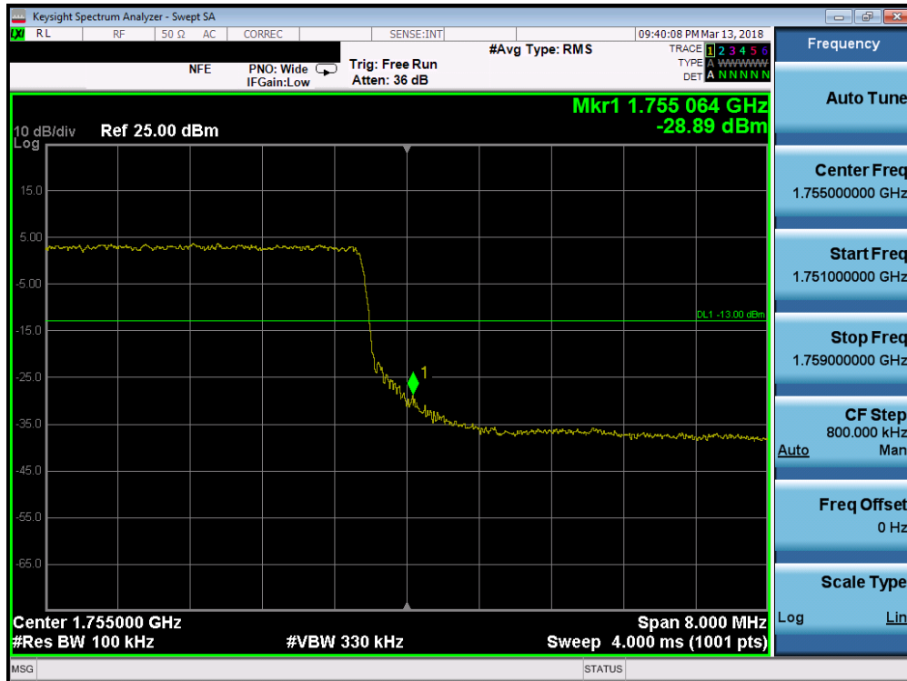
Plot 7-157. Upper Band Edge Plot (Band 4 - 10.0MHz QPSK - Full RB Configuration)
