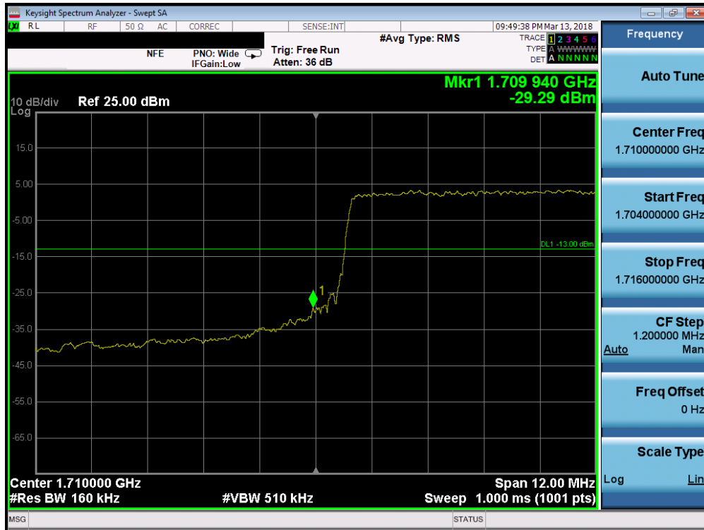
Plot 7-161. Lower Band Edge Plot (Band 66/4 - 15.0MHz QPSK - Full RB Configuration)
