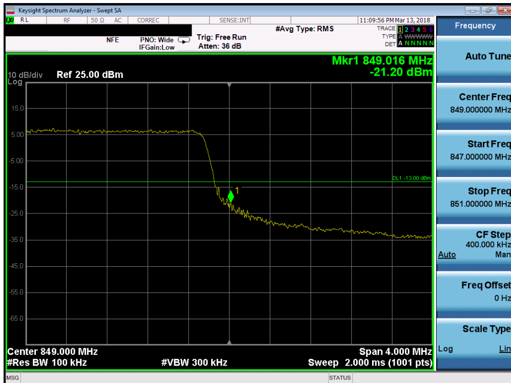
Plot 7-134. Upper Band Edge Plot (Band 5 - 5.0MHz QPSK - Full RB Configuration)
