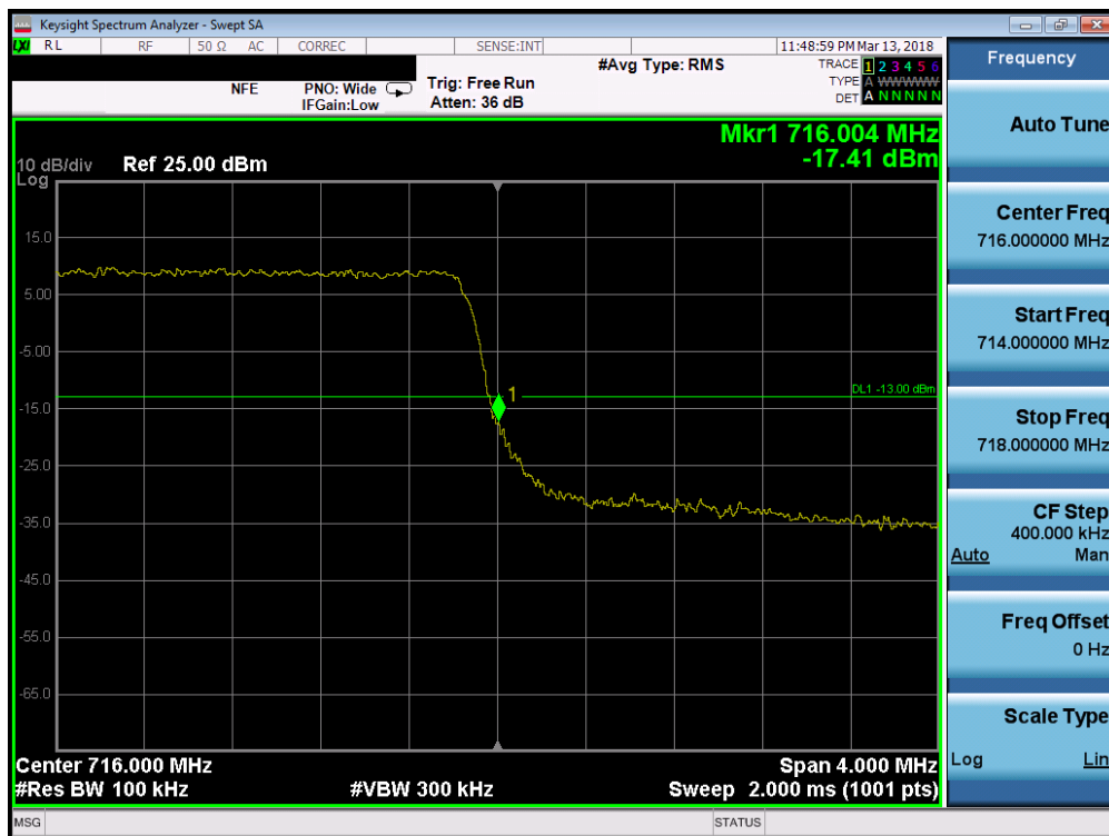
Plot 7-122. Upper Band Edge Plot (Band 12 - 3.0MHz QPSK - Full RB Configuration)
