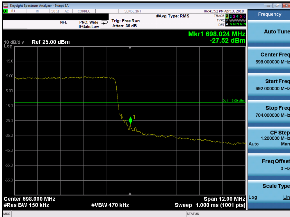
Plot 7-116. Upper Band Edge Plot (Band 71 - 15.0MHz QPSK - Full RB Configuration)
