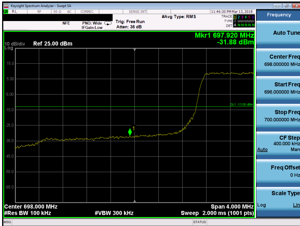
Plot 7-121. Lower Band Edge Plot (Band 12 - 3.0MHz QPSK - Full RB Configuration)
