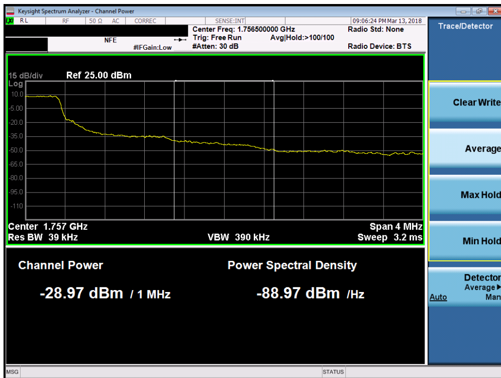
Plot 7-140. Upper Extended Band Edge Plot (Band 4 - 1.4MHz QPSK - Full RB Configuration)
