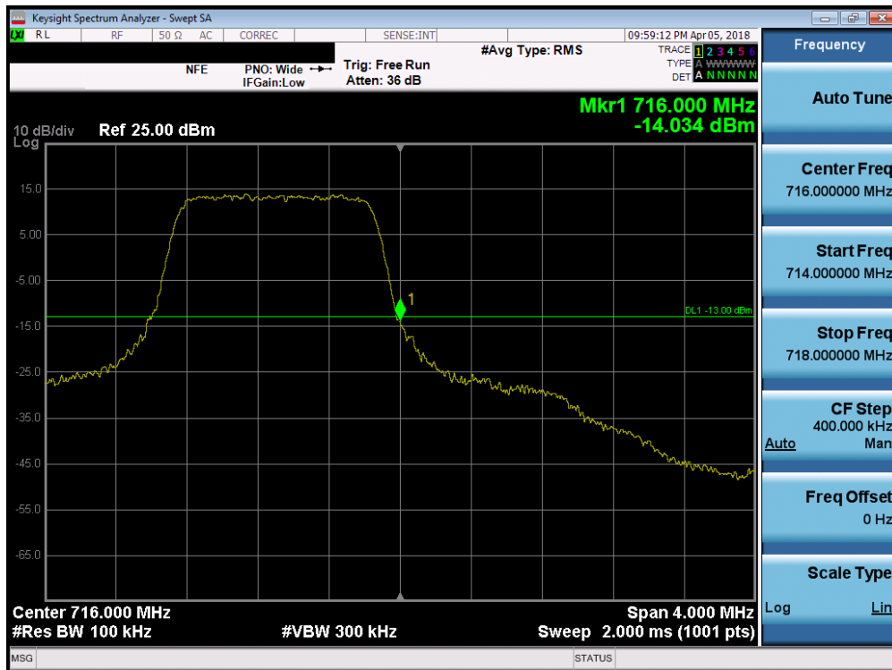
Plot 7-120. Upper Band Edge Plot (Band 12 - 1.4MHz QPSK - Full RB Configuration)
