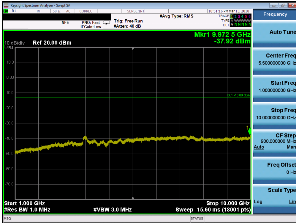
Plot 7-83. Conducted Spurious Plot (Band 5 - 3.0MHz QPSK - RB Size 1, RB Offset 0 - High Channel)
