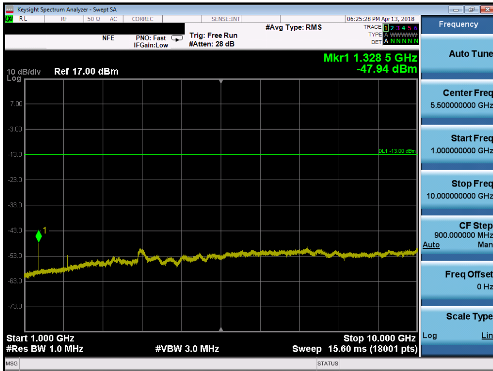
Plot 7-59. Conducted Spurious Plot (Band 71 - 20.0MHz QPSK - RB Size 1, RB Offset 0 - Low Channel)
