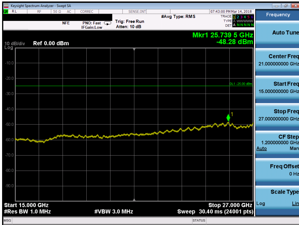
Plot 7-104. Conducted Spurious Plot (Band 7 - 10.0MHz QPSK - RB Size 1, RB Offset 0 - Low Channel)
