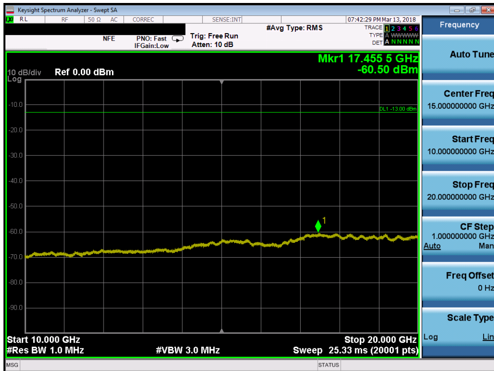
Plot 7-98. Conducted Spurious Plot (Band 2 - 5.0MHz QPSK - RB Size 1, RB Offset 0 - Mid Channel)
