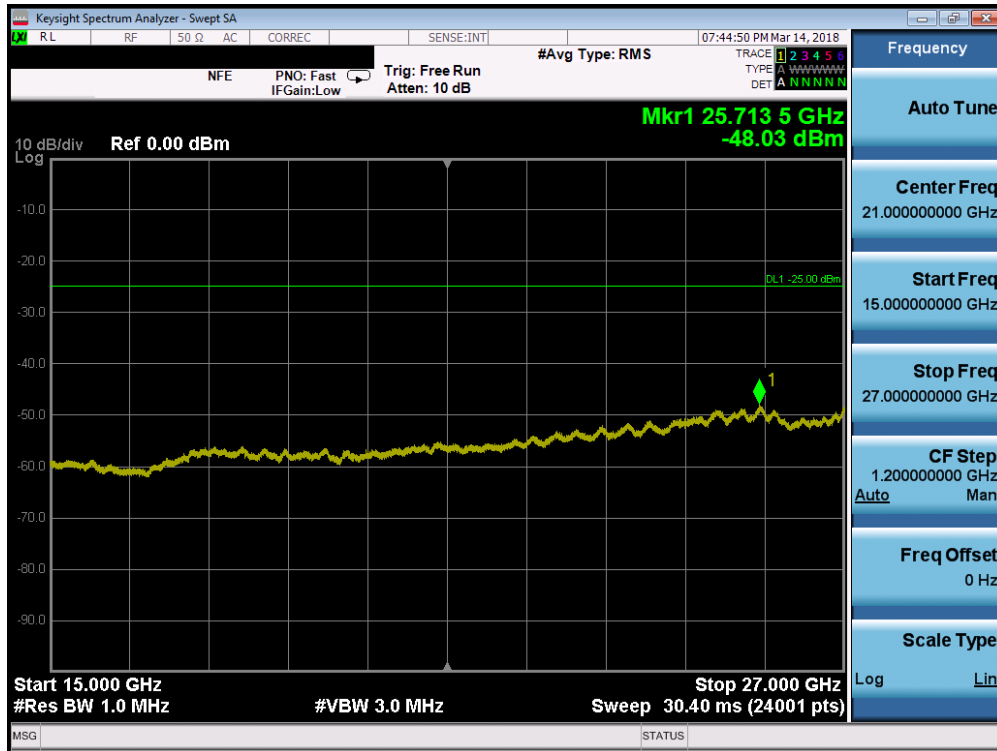
Plot 7-110. Conducted Spurious Plot (Band 7 - 10.0MHz QPSK - RB Size 1, RB Offset 0 - High Channel)
