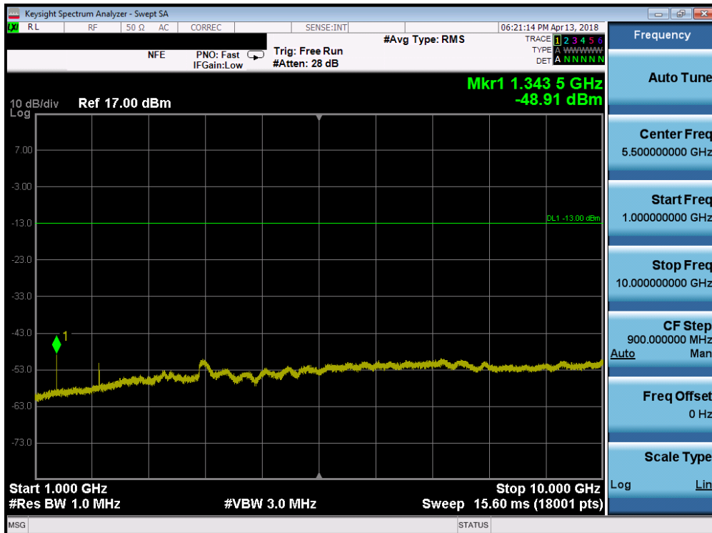
Plot 7-62. Conducted Spurious Plot (Band 71 - 20.0MHz QPSK - RB Size 1, RB Offset 0 - Mid Channel)
