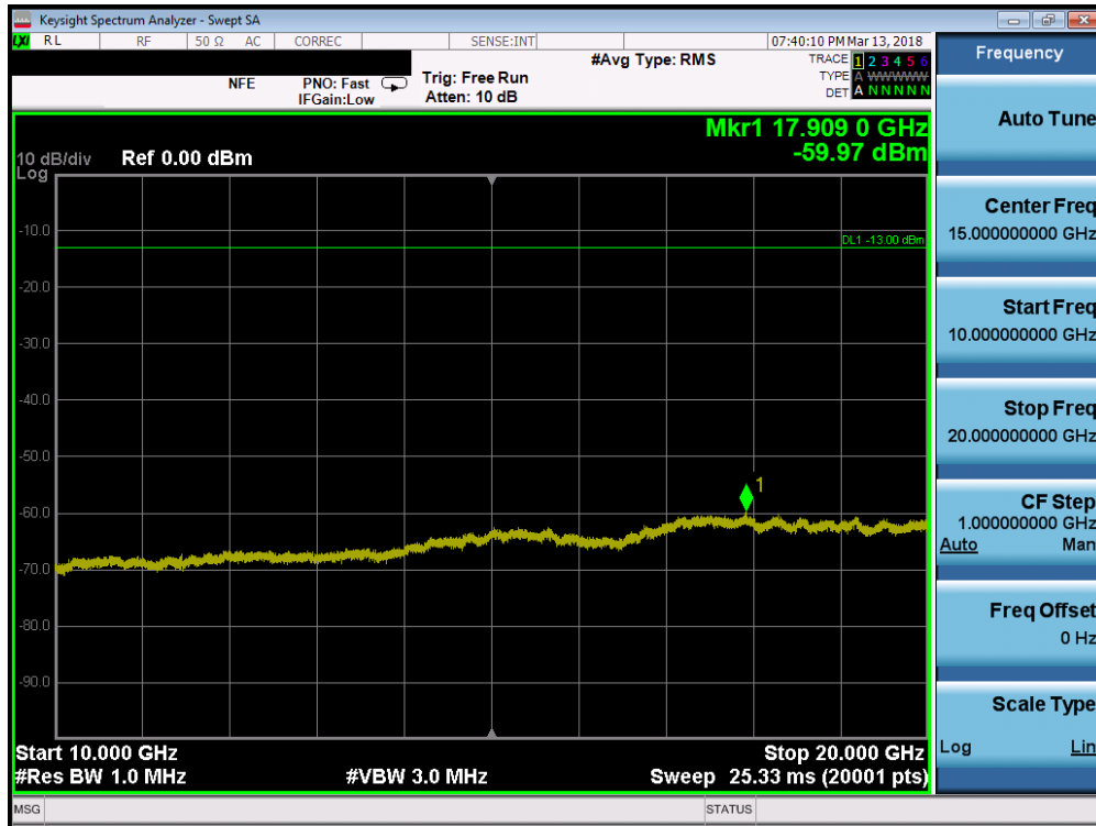
Plot 7-101. Conducted Spurious Plot (Band 2 - 5.0MHz QPSK - RB Size 1, RB Offset 0 - High Channel)
