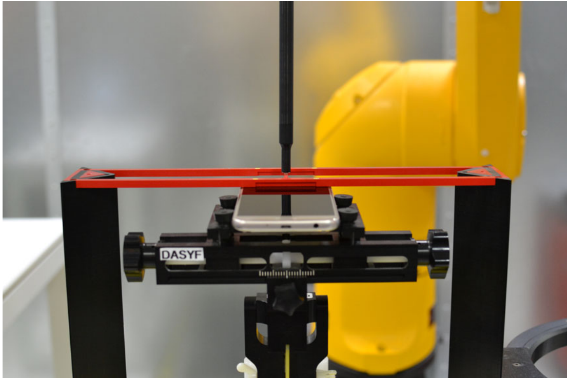
Figure 18-1 Ear Reference Point HAC Phantom Alignment
