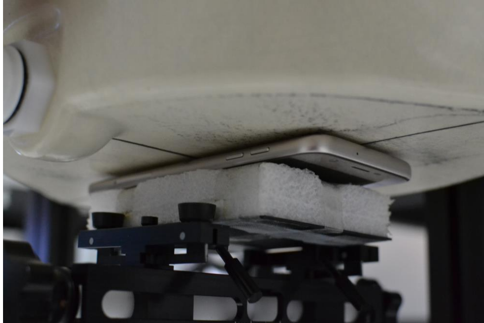
SAR Test Setup Photo 7: Back Side at 0.2 cm
