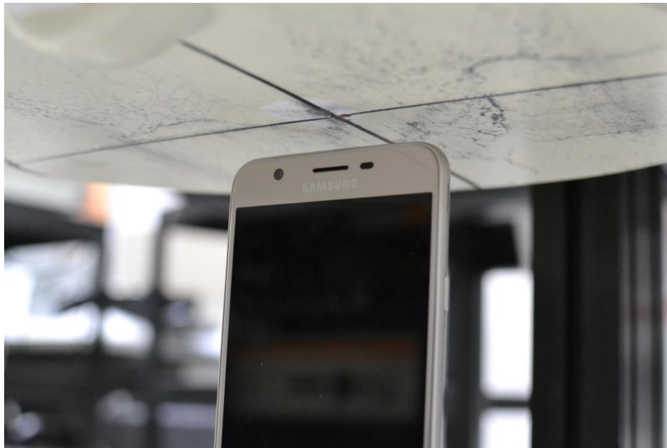
SAR Test Setup Photo 12: Top Edge at 1.0 cm
