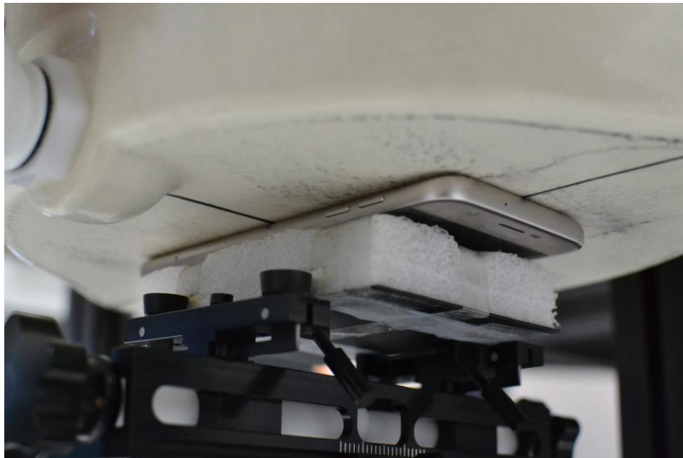
SAR Test Setup Photo 8: Back Side at 0.0 cm
