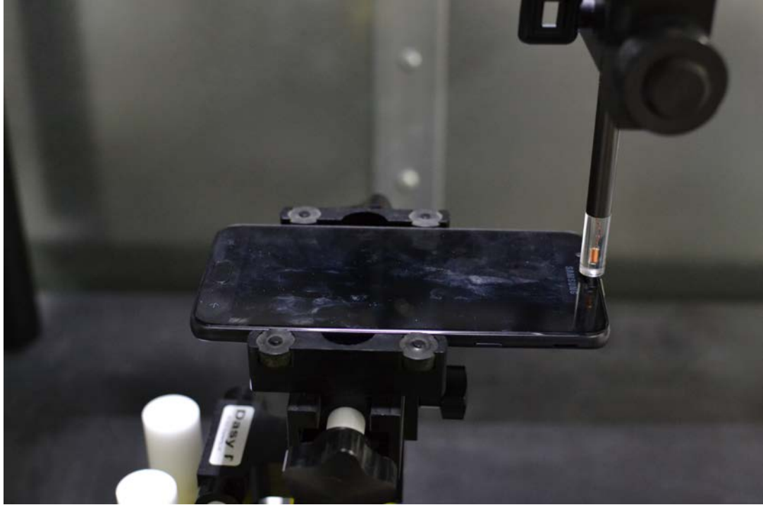
Figure 16-1 Test Setup for Wireless Device
