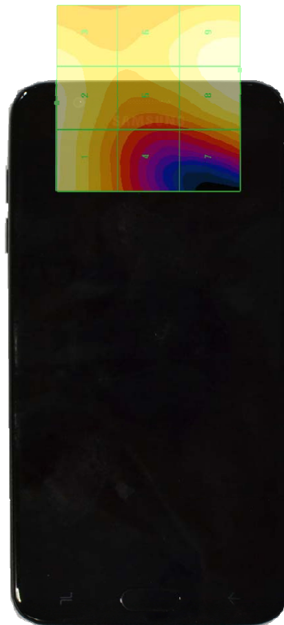
Figure 17-4 E-Field WD Scan overlay
