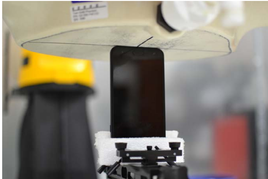
SAR Test Setup Photo 16 Bottom Edge at 0.0 cm
