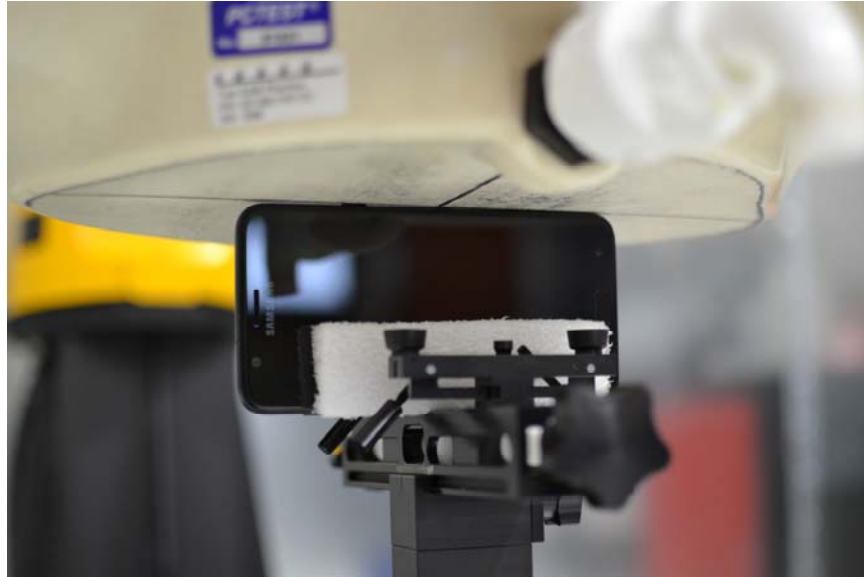
SAR Test Setup Photo 18 Right Edge at 0.0 cm
