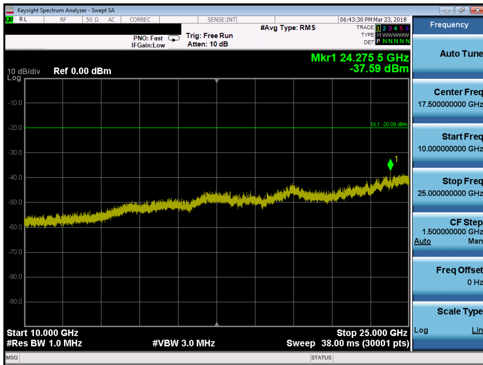
Plot 7-26. Conducted Spurious Plot (802.11b – Ch. 1)
