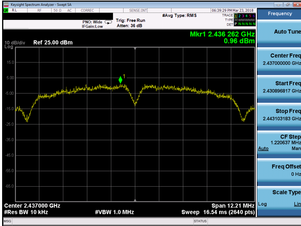
Plot 7-11. Power Spectral Density Plot (802.11b – Ch. 6)
