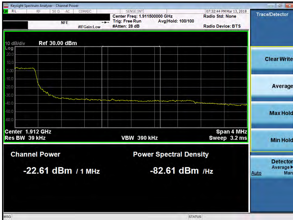
Plot 7-151. Upper Extended Band Edge Plot (Band 2 - 3.0MHz QPSK - Full RB Configuration)
