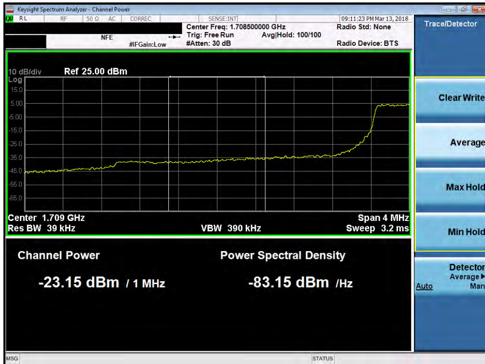
Plot 7-125. Lower Extended Band Edge Plot (Band 4 - 3.0MHz QPSK - Full RB Configuration)
