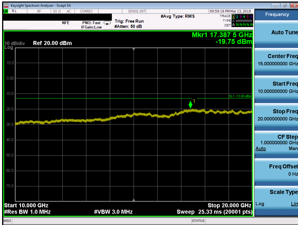
Plot 7-83. Conducted Spurious Plot (Band 4 - 20.0MHz QPSK - RB Size 1, RB Offset 0 - High Channel)
