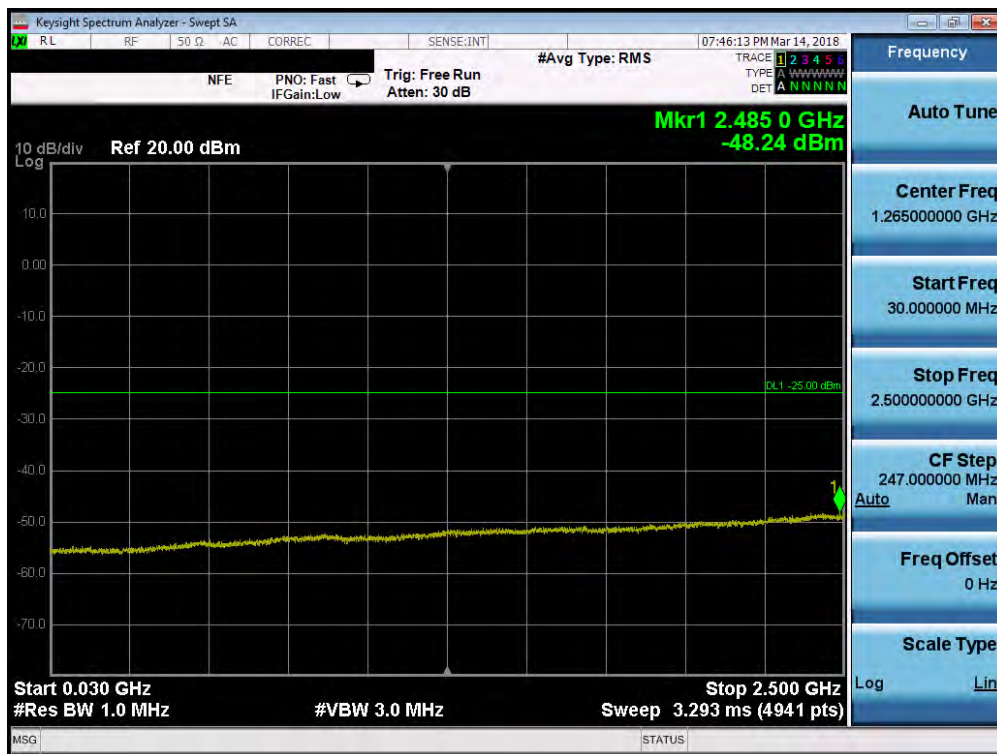
Plot 7-96. Conducted Spurious Plot (Band 7 - 10.0MHz QPSK - RB Size 1, RB Offset 0 - Mid Channel)
