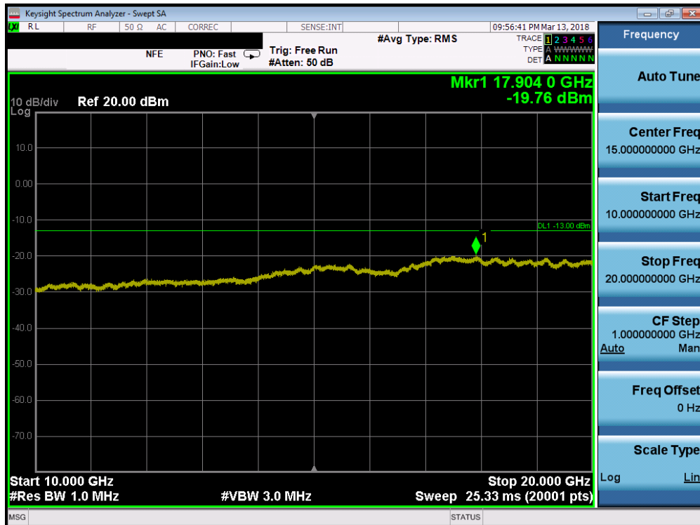
Plot 7-80. Conducted Spurious Plot (Band 4 - 20.0MHz QPSK - RB Size 1, RB Offset 0 - Mid Channel)
