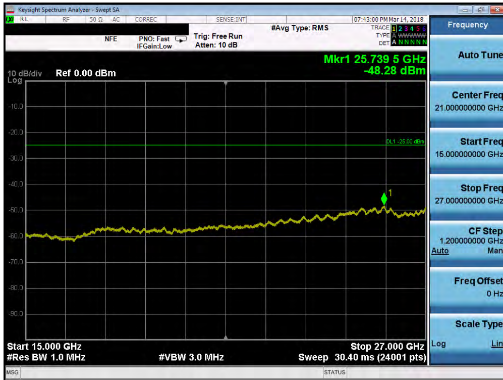
Plot 7-95. Conducted Spurious Plot (Band 7 - 10.0MHz QPSK - RB Size 1, RB Offset 0 - Low Channel)
