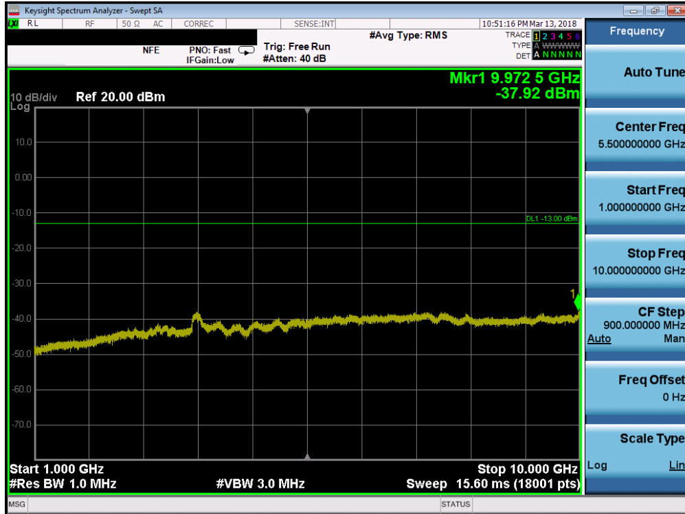
Plot 7-74. Conducted Spurious Plot (Band 5 - 3.0MHz QPSK - RB Size 1, RB Offset 0 - High Channel)
