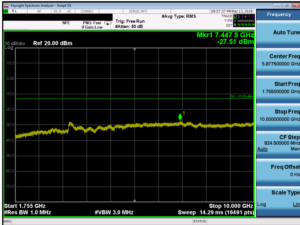
Plot 7-76. Conducted Spurious Plot (Band 4 - 20.0MHz QPSK - RB Size 1, RB Offset 0 - Low Channel)
