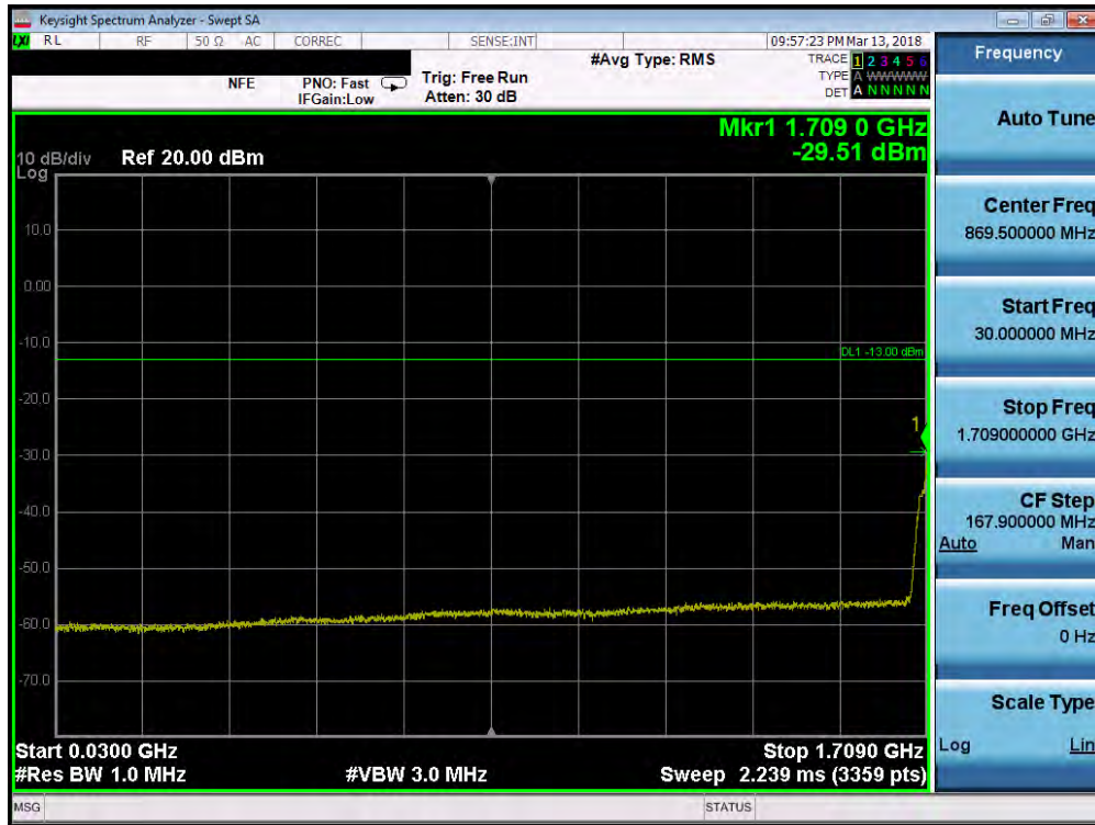
Plot 7-75. Conducted Spurious Plot (Band 4 - 20.0MHz QPSK - RB Size 1, RB Offset 0 - Low Channel)
