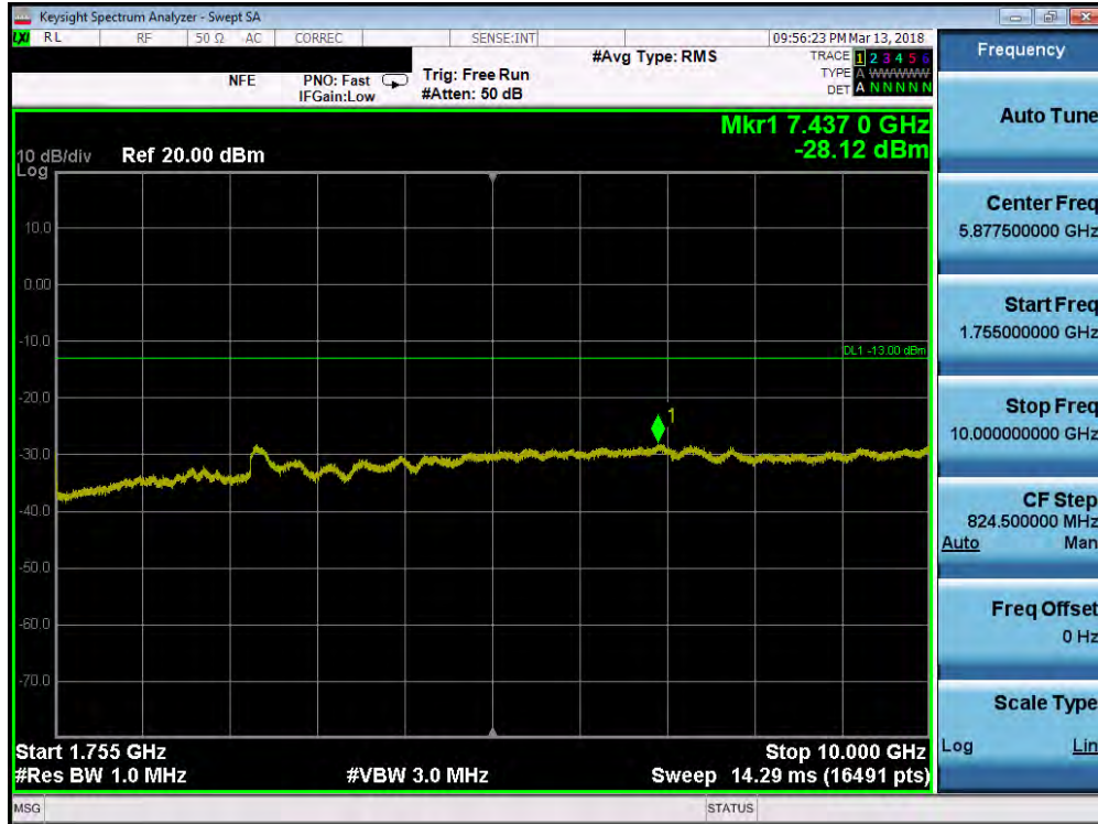
Plot 7-79. Conducted Spurious Plot (Band 4 - 20.0MHz QPSK - RB Size 1, RB Offset 0 - Mid Channel)
