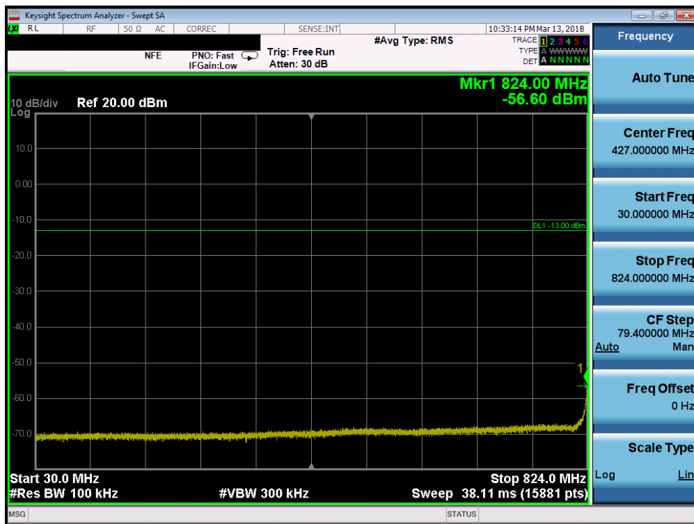
Plot 7-69. Conducted Spurious Plot (Band 5 - 3.0MHz QPSK - RB Size 1, RB Offset 0 - Mid Channel)
