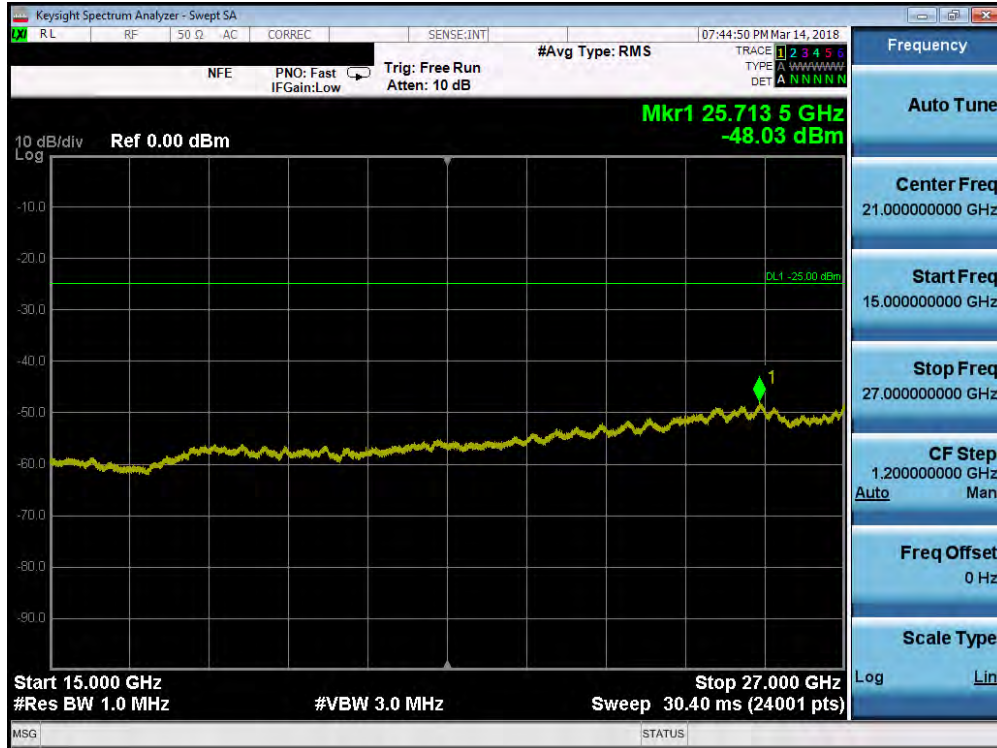
Plot 7-101. Conducted Spurious Plot (Band 7 - 10.0MHz QPSK - RB Size 1, RB Offset 0 - High Channel)
