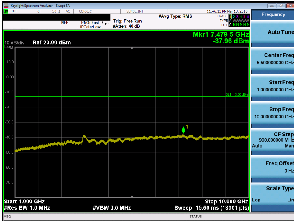
Plot 7-59. Conducted Spurious Plot (Band 12 - 3.0MHz QPSK - RB Size 1, RB Offset 0 - Low Channel)
