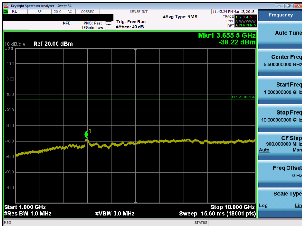
Plot 7-62. Conducted Spurious Plot (Band 12 - 3.0MHz QPSK - RB Size 1, RB Offset 0 - Mid Channel)
