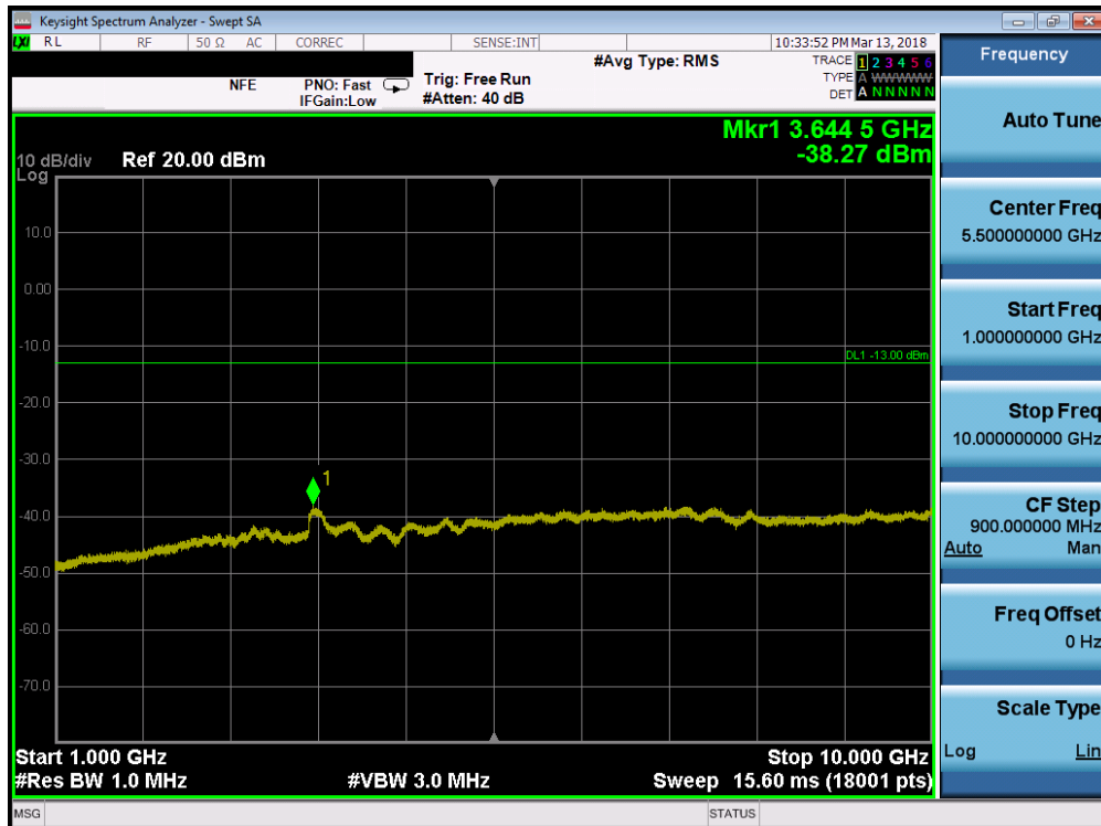
Plot 7-71. Conducted Spurious Plot (Band 5 - 3.0MHz QPSK - RB Size 1, RB Offset 0 - Mid Channel)
