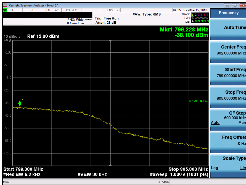
Plot 7-17. Upper Emission Mask Band Edge Plot (LTE B14 - 5MHz QPSK – RB Size 25)
