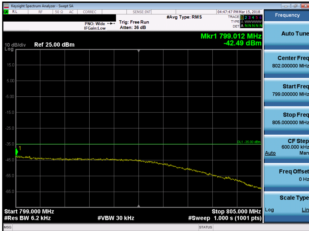
Plot 7-21. Upper Emission Mask Band Edge Plot (LTE B14 - 10MHz QPSK – RB Size 50)
