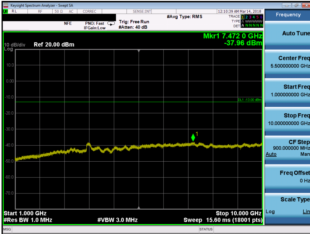
Plot 7-7. Conducted Spurious Plot (LTE B14 – 5.0MHz QPSK – RB Size 1, RB Offset 0 – Low Channel)
