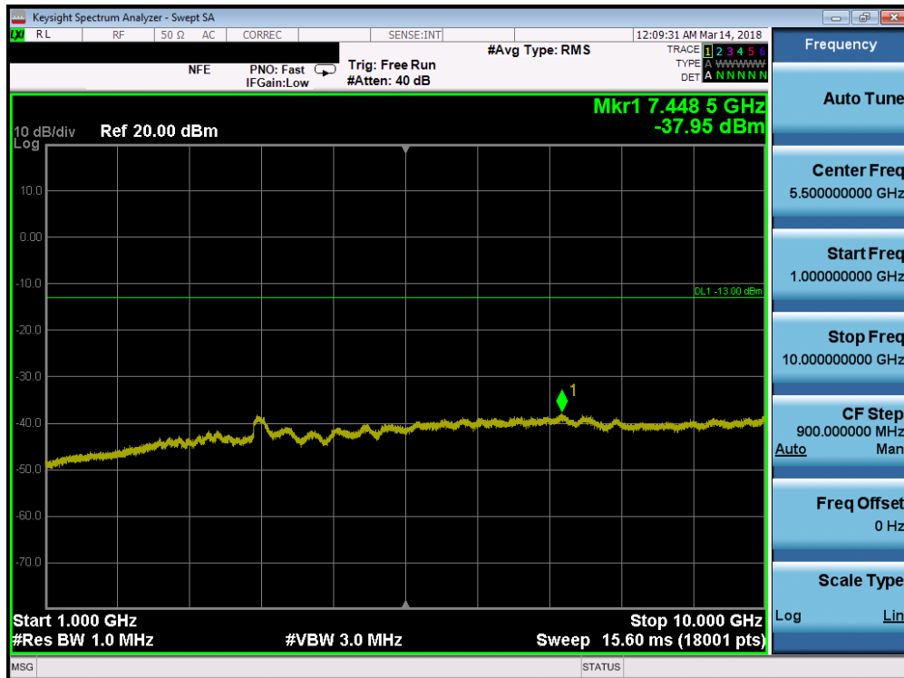
Plot 7-10. Conducted Spurious Plot (LTE B14 – 5.0MHz QPSK – RB Size 1, RB Offset 0 – Mid Channel)
