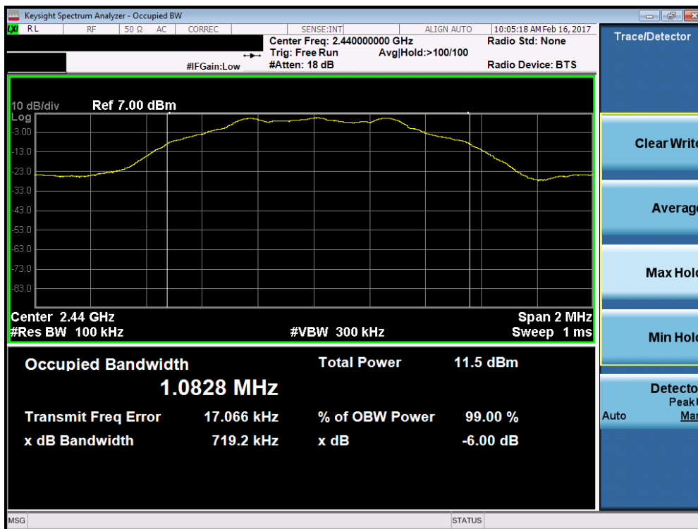
Plot 7-2. 6dB Bandwidth Plot (Bluetooth (LE) – Ch. 19)
