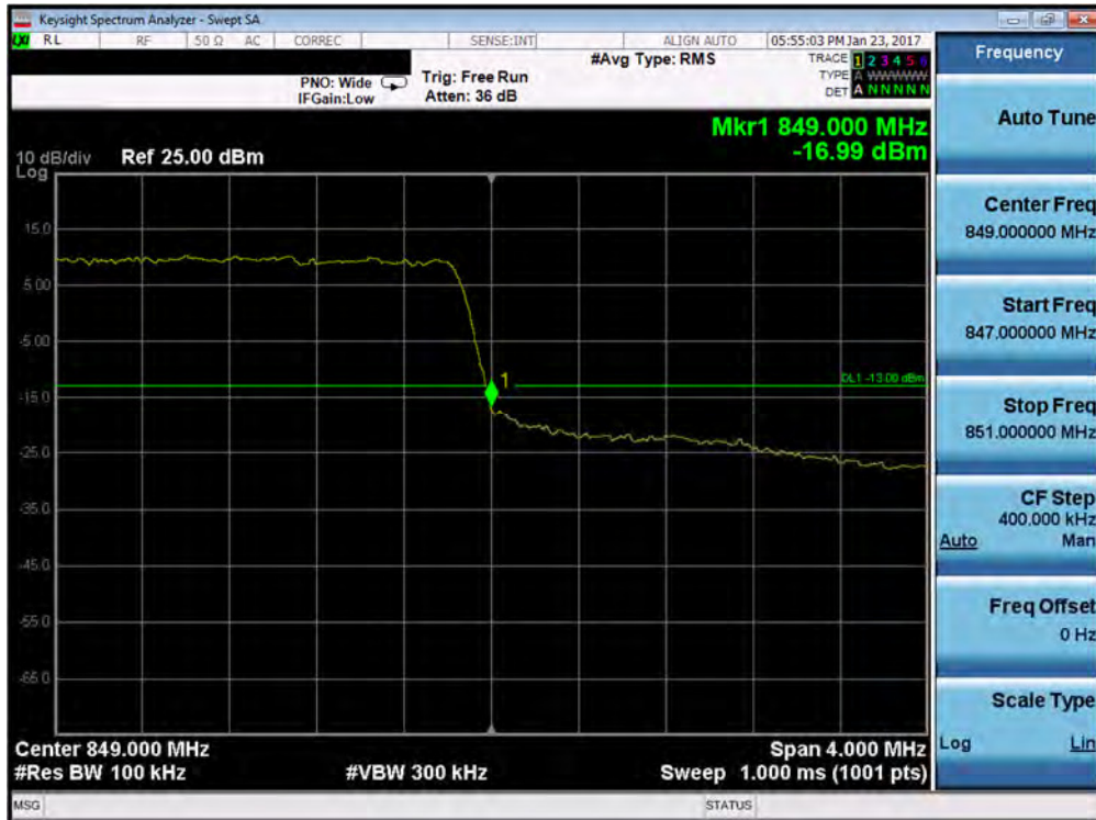
Plot 7-90. Upper Band Edge Plot (Band 5 – 3.0MHz QPSK – RB Size 15)
