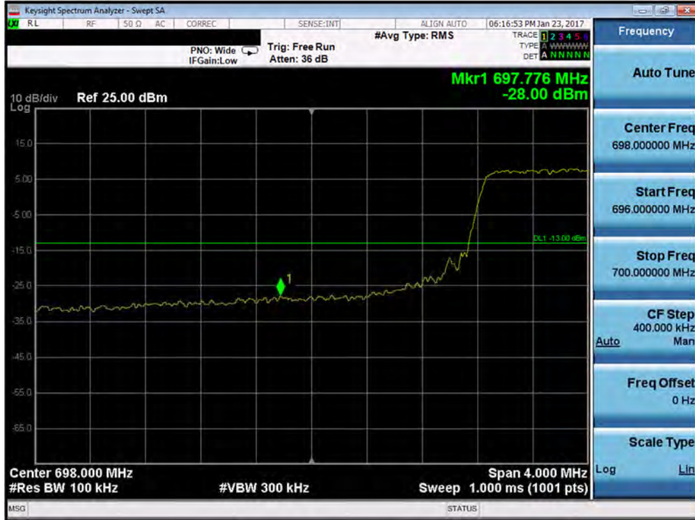
Plot 7-81. Lower Band Edge Plot (Band 12 – 5.0MHz QPSK – RB Size 25)
