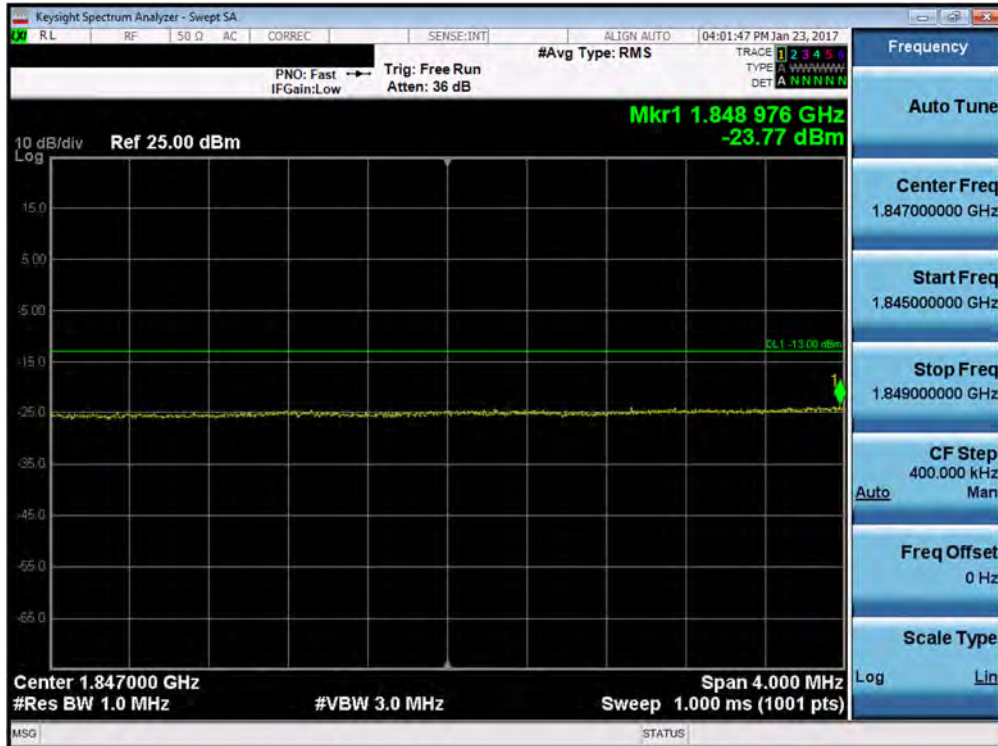
Plot 7-140. Lower Extended Band Edge Plot (Band 2 – 20.0MHz QPSK – RB Size 100)
