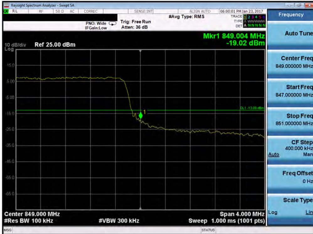
Plot 7-92. Upper Band Edge Plot (Band 5 – 5.0MHz QPSK – RB Size 25)
