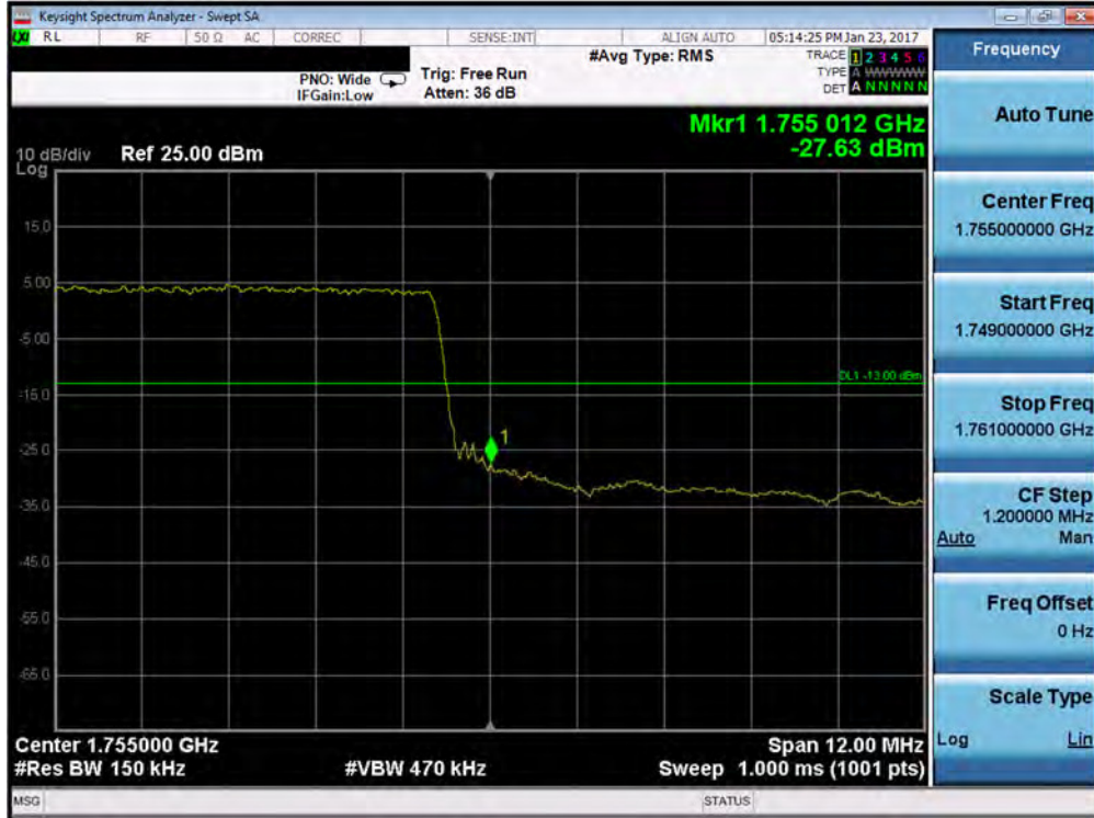
Plot 7-113. Upper Band Edge Plot (Band 4 – 15.0MHz QPSK – RB Size 75)
