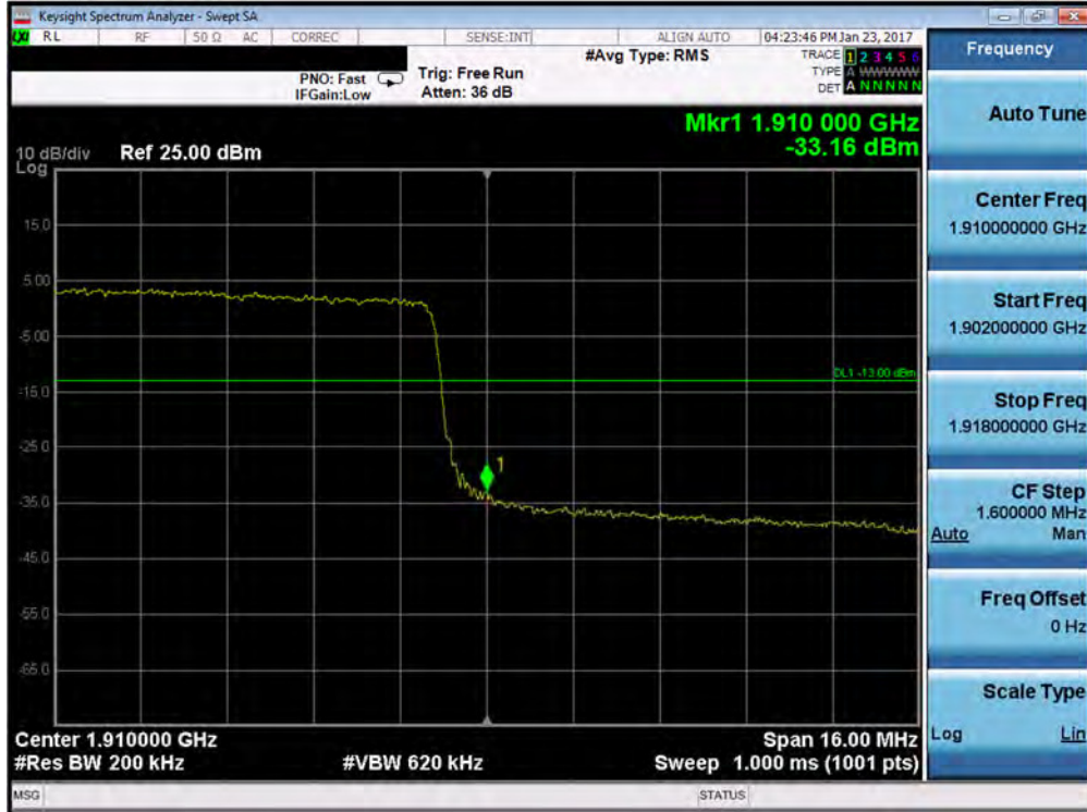
Plot 7-141. Upper Band Edge Plot (Band 2 – 20.0MHz QPSK – RB Size 100)
