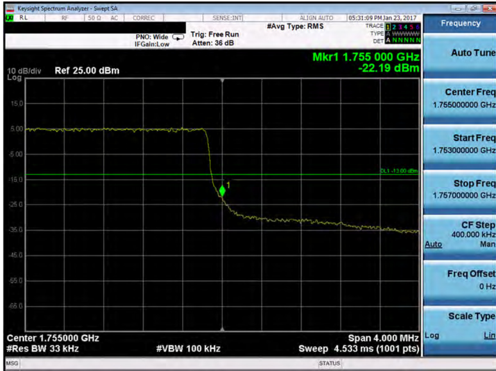
Plot 7-101. Upper Band Edge Plot (Band 4 – 3.0MHz QPSK – RB Size 15)
