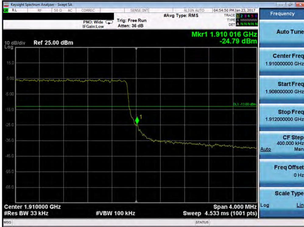
Plot 7-125. Upper Band Edge Plot (Band 2 – 3.0MHz QPSK – RB Size 15)
