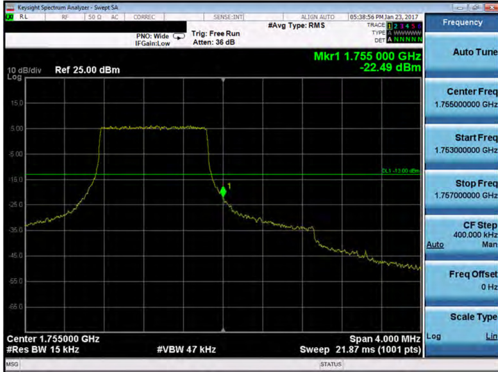
Plot 7-97. Upper Band Edge Plot (Band 4 – 1.4MHz QPSK – RB Size 6)
