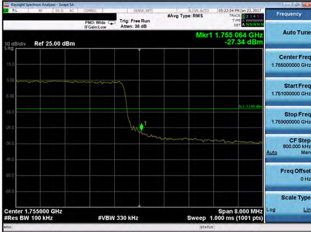
Plot 7-109. Upper Band Edge Plot (Band 4 – 10.0MHz QPSK – RB Size 50)
