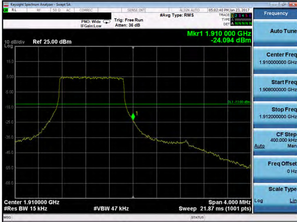
Plot 7-121. Upper Band Edge Plot (Band 2 – 1.4MHz QPSK – RB Size 6)
