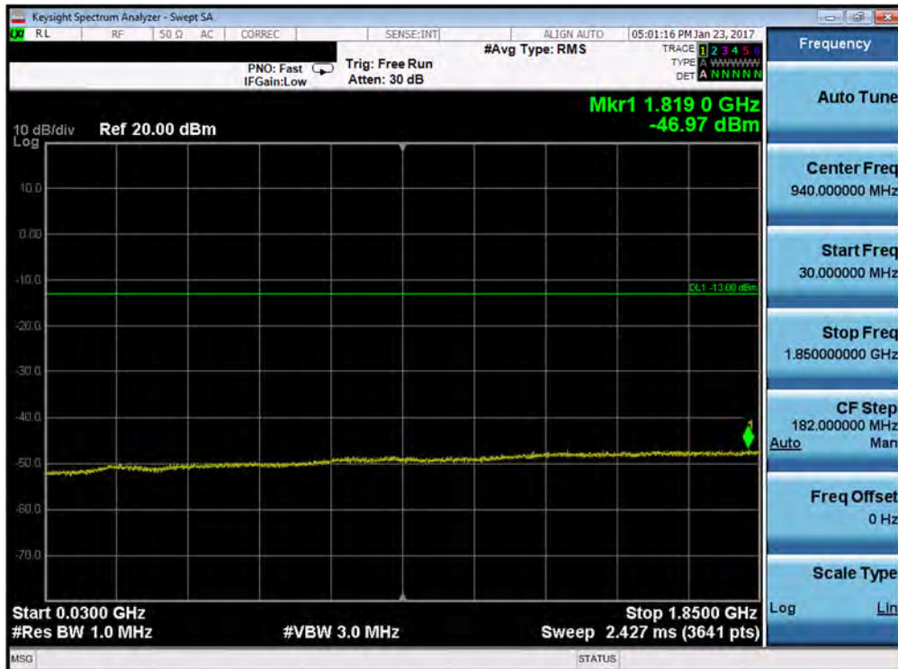
Plot 7-74. Conducted Spurious Plot (Band 2 – 1.4MHz QPSK – RB Size 1, RB Offset 0 – High Channel)
