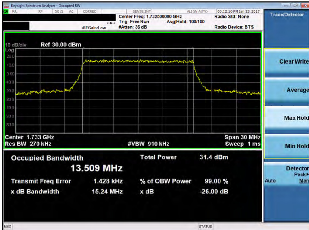
Plot 7-26. Occupied Bandwidth Plot (Band 4 – 15.0MHz 16-QAM – RB Size 75)
