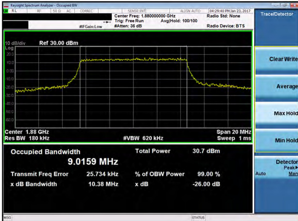
Plot 7-36. Occupied Bandwidth Plot (Band 2 – 10.0MHz 16-QAM – RB Size 50)
