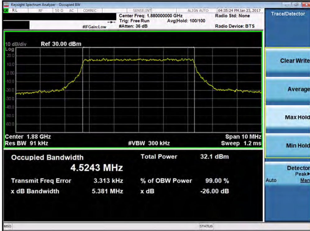
Plot 7-33. Occupied Bandwidth Plot (Band 2 – 5.0MHz QPSK – RB Size 25)
