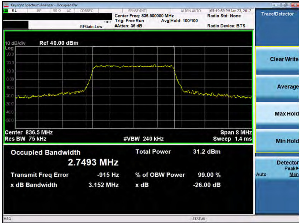
Plot 7-12. Occupied Bandwidth Plot (Band 5 – 3.0MHz 16-QAM – RB Size 15)
