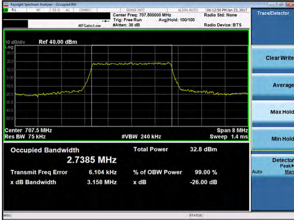
Plot 7-3. Occupied Bandwidth Plot (Band 12 – 3.0MHz QPSK – RB Size 15)
