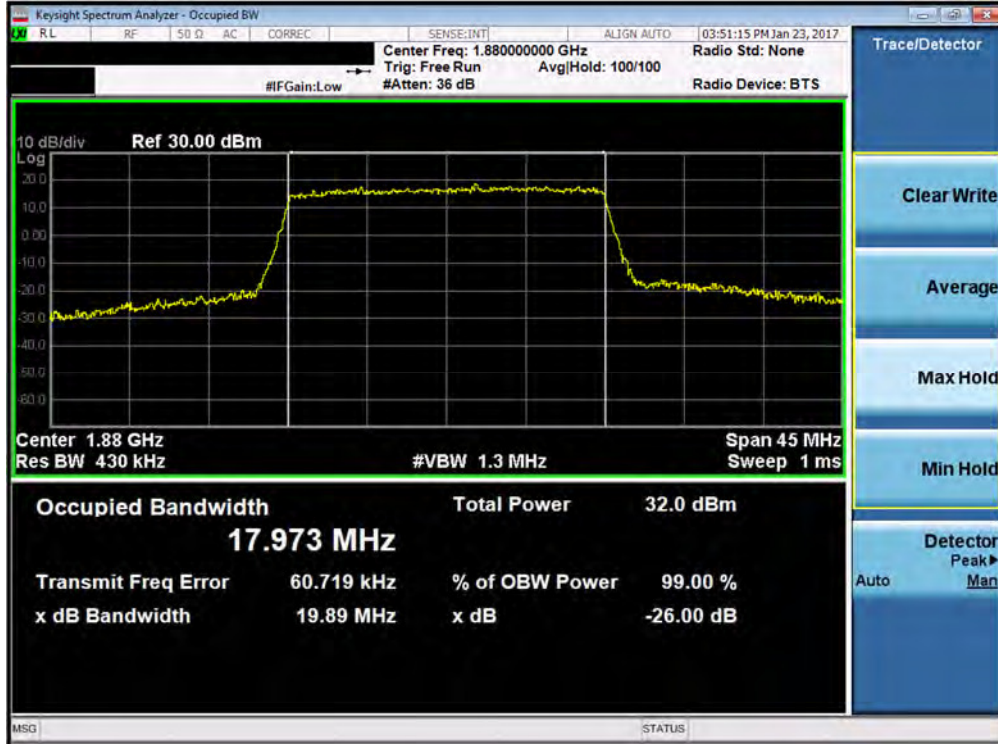
Plot 7-39. Occupied Bandwidth Plot (Band 2 – 20.0MHz QPSK – RB Size 100)
