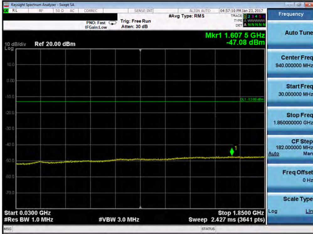
Plot 7-71. Conducted Spurious Plot (Band 2 – 1.4MHz QPSK – RB Size 1, RB Offset 0 – Mid Channel)
