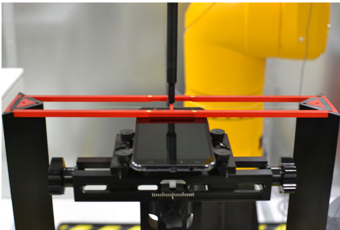
Figure 17-1 Ear Reference Point HAC Phantom Alignment
