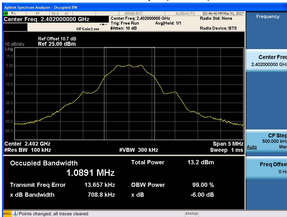
6 dB Bandwidth plot (Low-CH 0)
