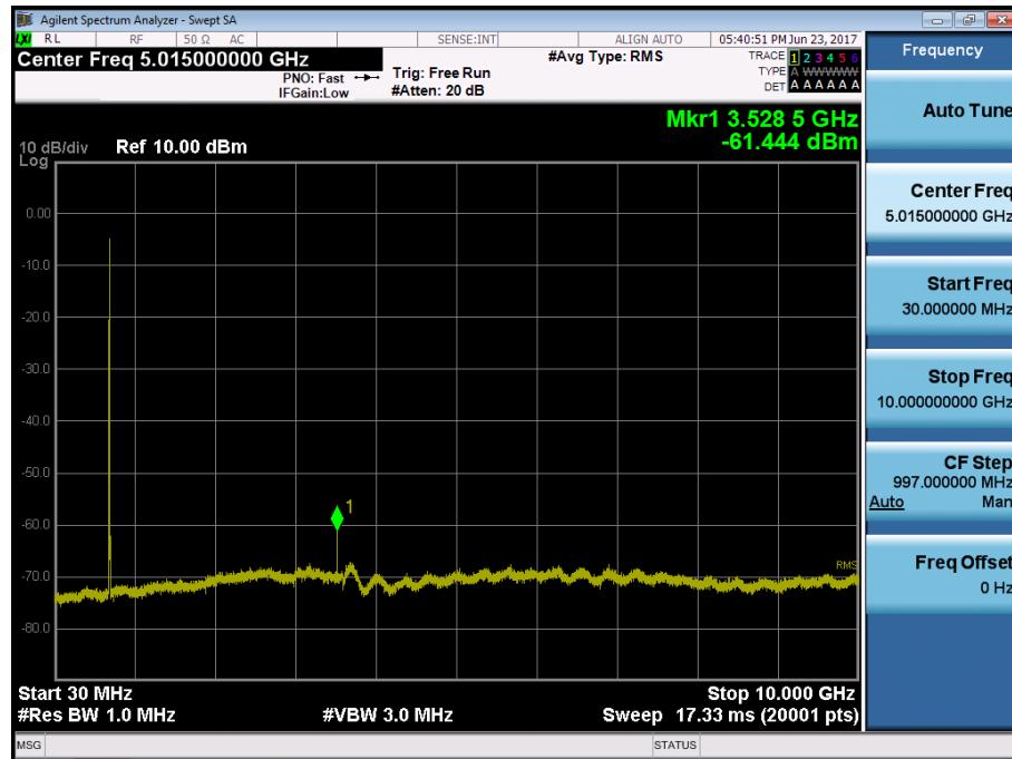
BAND 17. Conducted Spurious Plot\_ (23800ch\_10MHz\_QPSK\_RB 1\_0)
