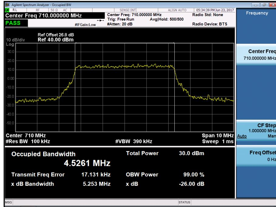
BAND 17. Occupied Bandwidth Plot (10M BW Ch.23790 QPSK RB 50)
