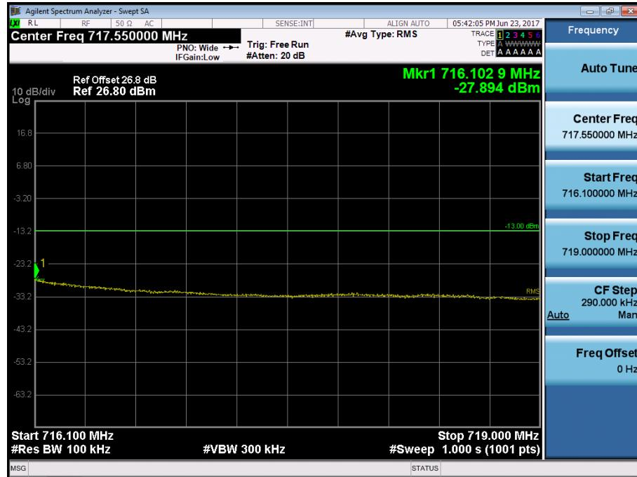
BAND 17. Conducted Spurious Plot\_ (23755ch\_5MHz\_QPSK\_RB 1\_0)
