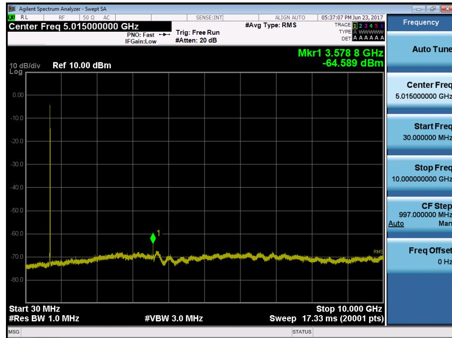
BAND 17. Conducted Spurious Plot\_ (23780ch\_10MHz\_QPSK\_RB 1\_0)
