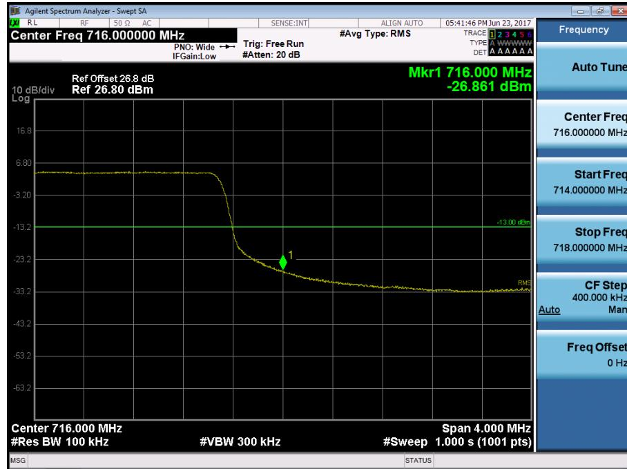
BAND 17. Upper Extended Band Edge Plot (10M BW Ch.23800 QPSK\_RB50) -3
