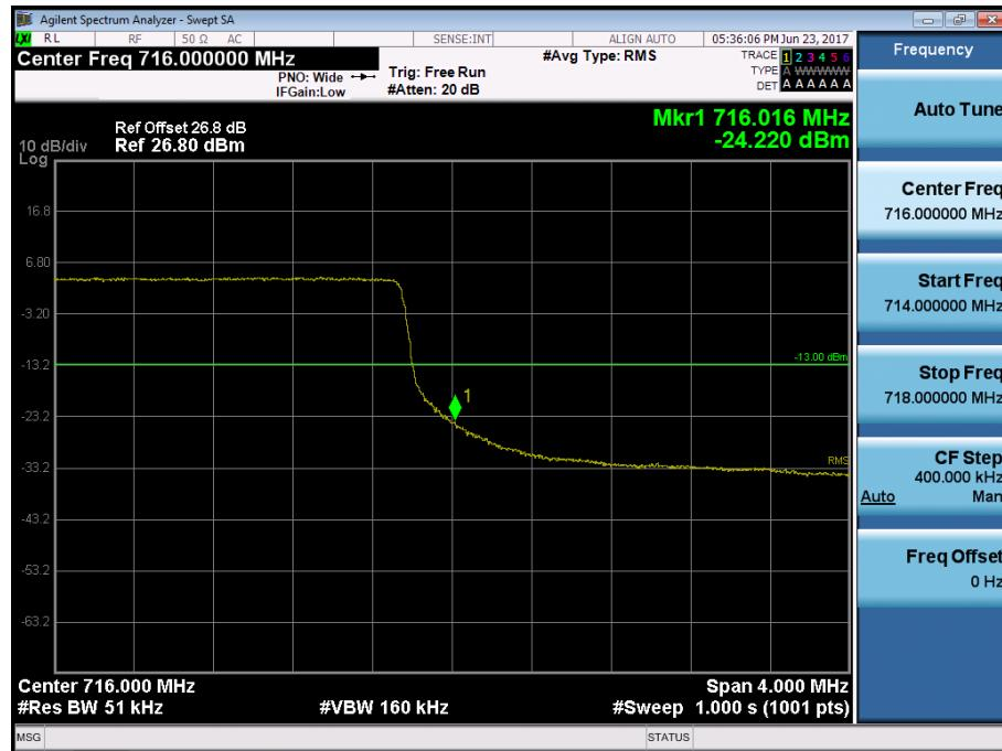
BAND 17. Upper Extended Band Edge Plot (5M BW Ch.23825 QPSK\_RB25) -3
