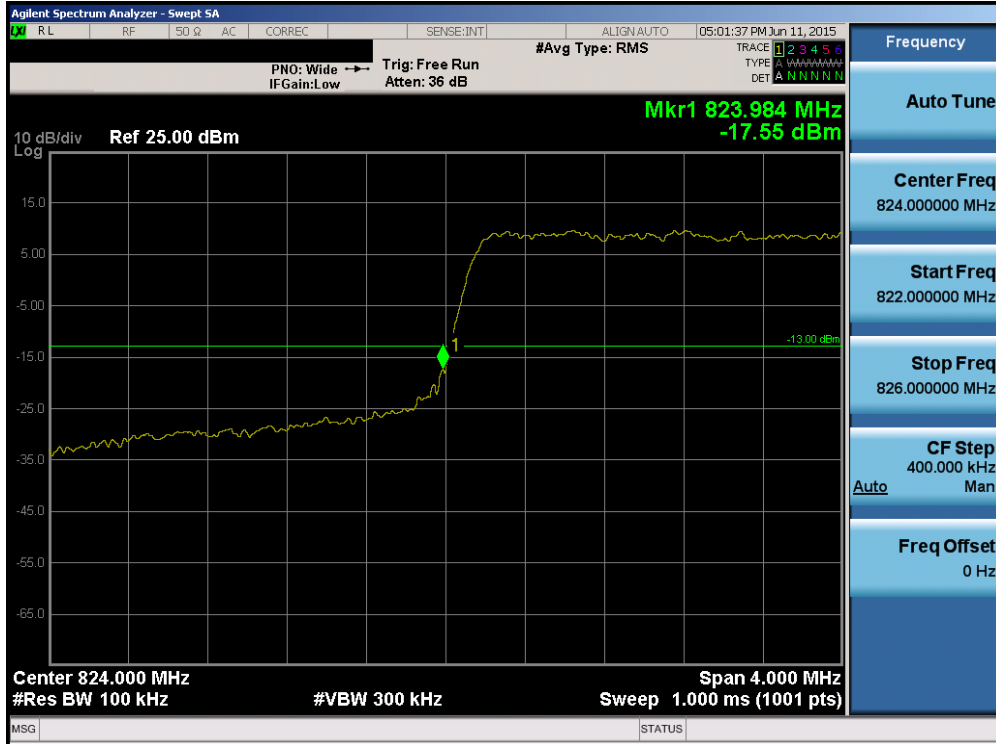
Plot 6-81. Lower Band Edge Plot (Band 5 – 3.0MHz QPSK – RB Size 15)
