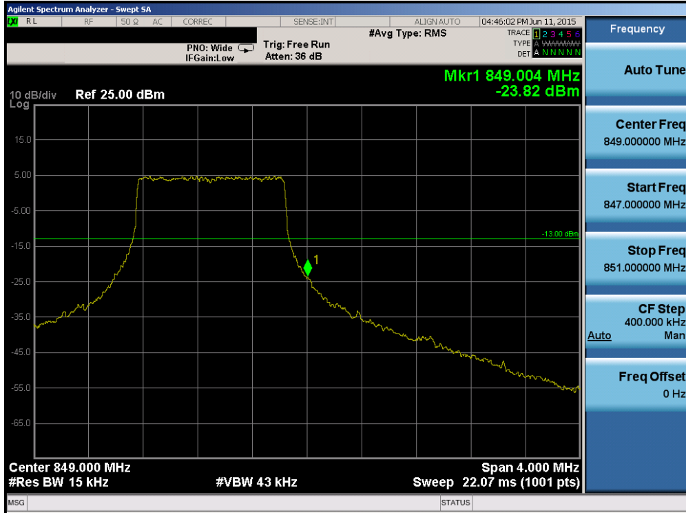
Plot 6-79. Upper Band Edge Plot (Band 5 – 1.4MHz QPSK – RB Size 6)
