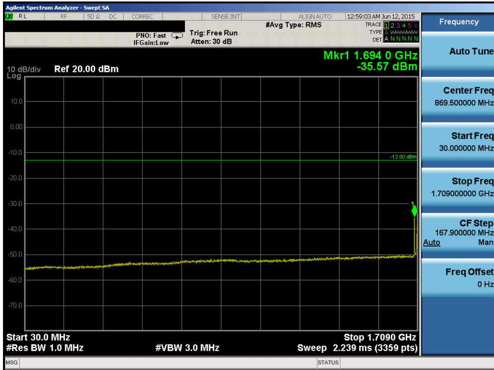
Plot 6-55. Conducted Spurious Plot (Band 4 – 20.0MHz QPSK – RB Size 1, RB Offset 0– Low Channel)
