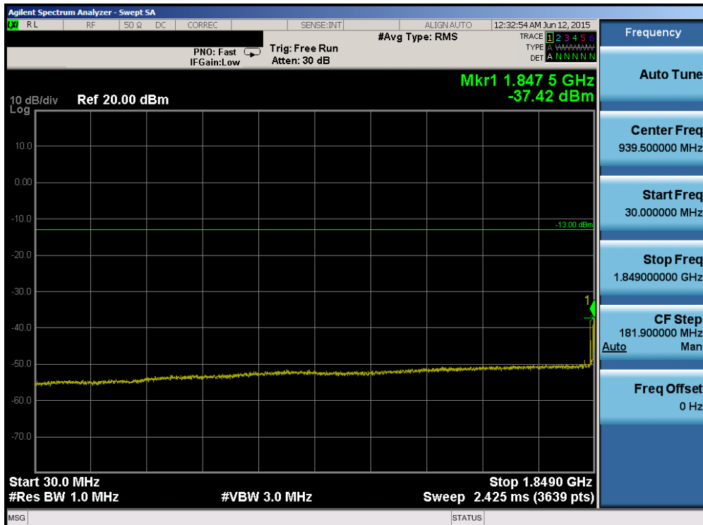
Plot 6-64. Conducted Spurious Plot (Band 2 – 20.0MHz QPSK – RB Size 1, RB Offset 0– Low Channel)
