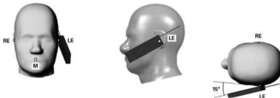
Figure 6.5. Tilt 15° position of the wireless device
